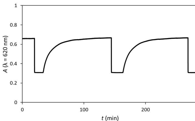
**Figure S3.2.** Response and recovery spectra of the 3D printed XB indicator film recorded under an alternative gas stream of Air and 100% CO<sub>2</sub>, revealing a 50% response time of  $t_{50\downarrow} = 0.17$  min and 50% recovery time of  $t_{50\uparrow} = 8.3$  min.
