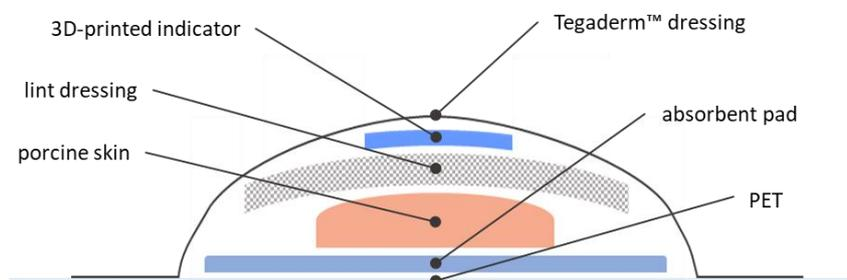
**Figure S2.2:** Schematic of the ‘smart’ wound dressing with a sample of inoculated, damaged porcine skin placed on a 50 µm film of clear PET. The dressing itself comprised a damp absorbent pad, on top of which were placed, a piece of inoculated damaged porcine skin, followed by a lint dressing and the 3D-printed indicator, all sealed in with a Tegaderm™ occlusive dressing.
