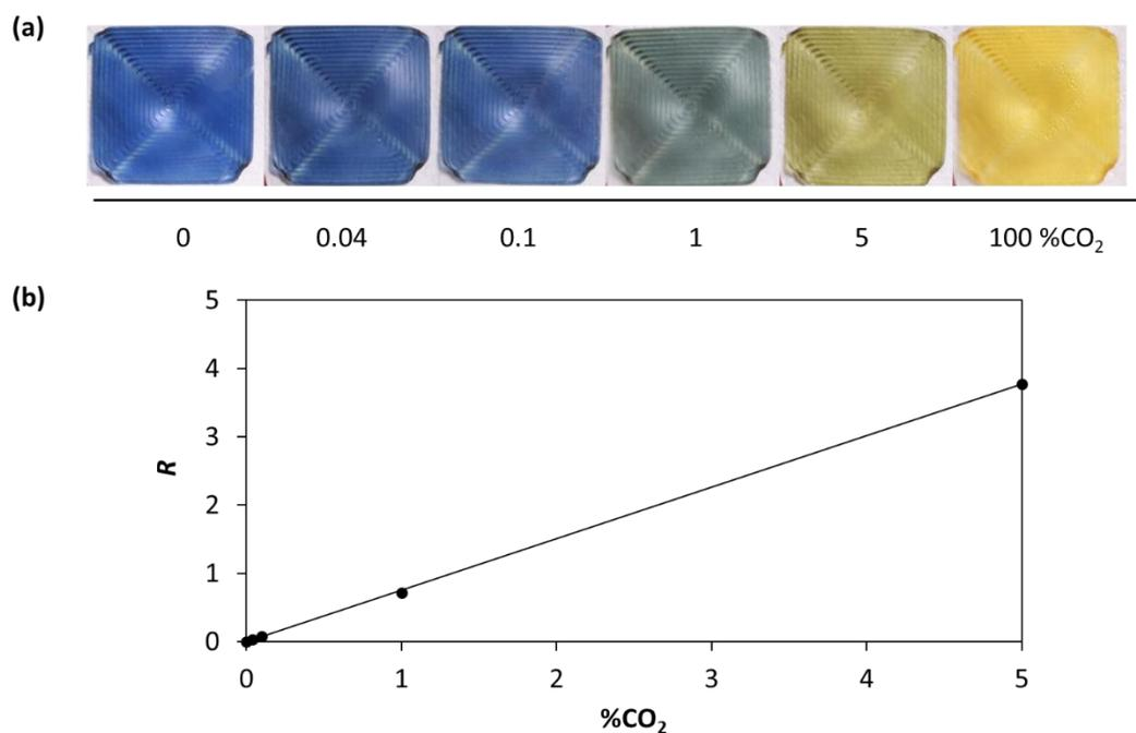
**Figure S3.3(a).** Digital photographs of the 3D printed XB indicator film in a 30°C gas cell as a function of the %CO<sub>2</sub> in the 100% humid gas stream. **(b).** Plot of  $R$  vs %CO<sub>2</sub>, where  $R$  values were calculated using eqn (S2) and apparent absorbance values,  $A'$  derived from colour analysis of the images given in Figure S3.3(a). The  $R$  vs %CO<sub>2</sub> plot yields a gradient of  $0.79 \pm 0.05 \text{ \%}^{-1}$  ( $R^2 = 0.9962$ ).
