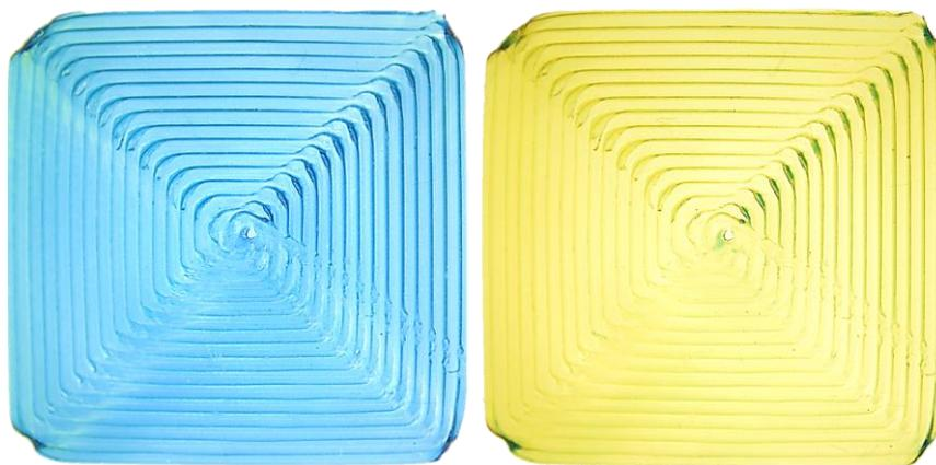
**Figure S3.1.** From left to right photographic images of the 12 mm square 3D printed, XB CO<sub>2</sub> indicator in the absence of CO<sub>2</sub> (in Argon) and in its present (100% CO<sub>2</sub>), respectively.
