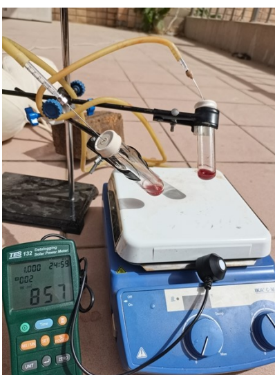
Fig. S22 photocatalytic devices under the irradiation of natural sunlight.
