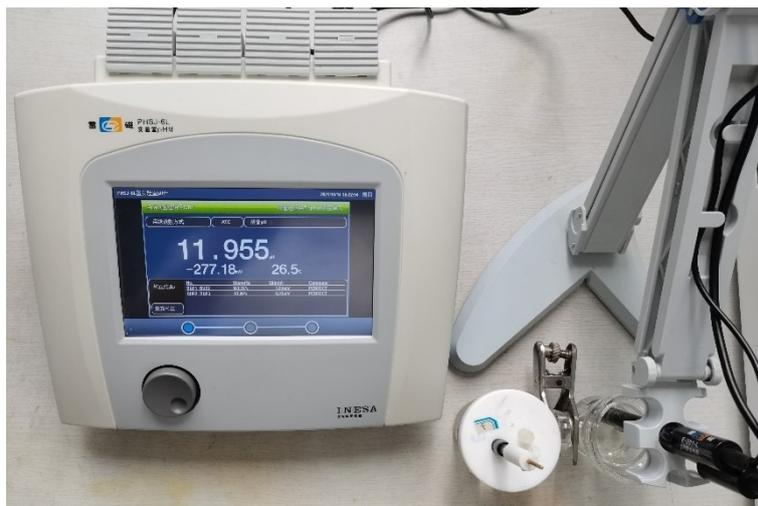
**Fig. S11** Photograph of pH test with electrolyte after 10 h of  $\text{NO}_2^-$ -RR electrolysis.
