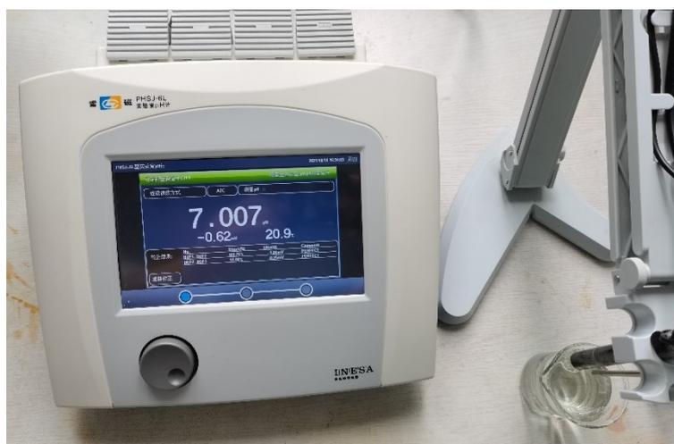
**Fig. S9** Photograph of pH test with electrolyte before  $\text{NO}_2^-$ RR electrolysis.
