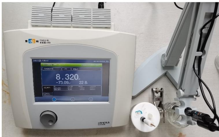
**Fig. S10** Photograph of pH test with electrolyte after 2 h of  $\text{NO}_2^-$ -RR electrolysis.
