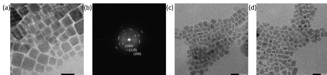
**Fig. S1** a, b) HRTEM image and its FFT pattern of  $\text{CsPb}_{1-x}\text{Mn}_x\text{Cl}_3$  NCs with nominal Mn content of 10 mol%. c, d) HRTEM images of  $\text{CsPb}_{1-x}\text{Mn}_x\text{Cl}_3$  NCs with nominal Mn content of 90 mol%. The black particles around the edges and corners of NCs been  $\text{Pb}^0$  caused by electron beam damage (ACS Nano 2017, 11, 2, 2124–2132; Chem. Mater. 2020, 32, 5410-5423).
