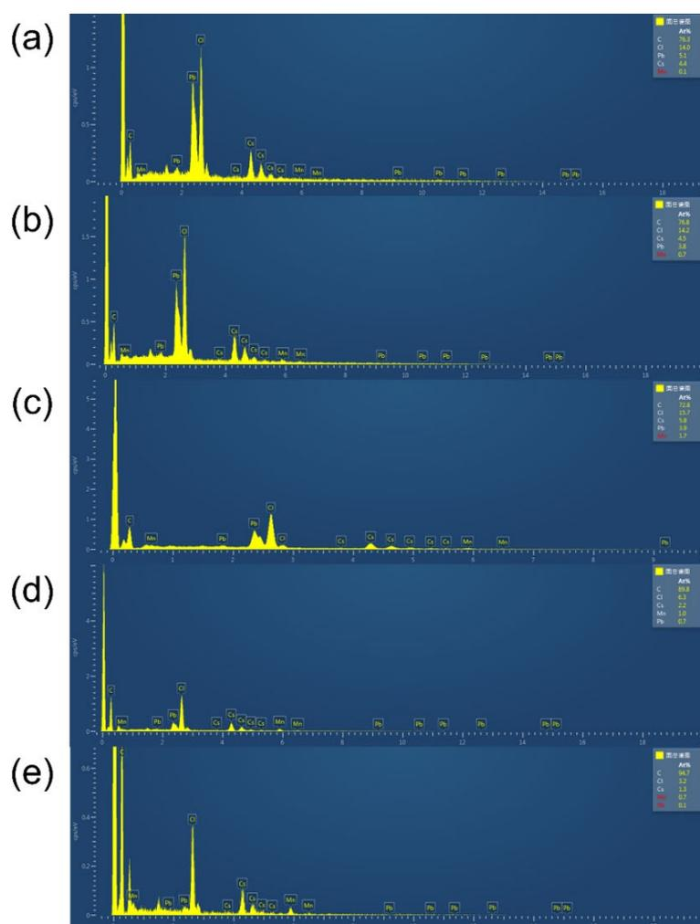
**Fig. S2** Energy dispersive X-ray (EDX) spectra of the  $\text{CsPb}_{1-x}\text{Mn}_x\text{Cl}_3$  NCs synthesized with  $\text{MnAc}_2:\text{PbAc}_2$  molar feed ratios of (a) 0.1: 0.9 (b) 0.3: 0.7 (c) 0.5: 0.5 (d) 0.7: 0.3 (e) 0.9: 0.1.
