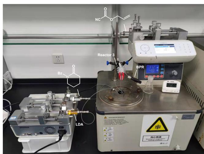
The flow reactor equipment consists of three pumps for reagent/solvent delivery. Before the start of the actual experiment, all reactors were primed with dry THF. Reactor 1 was pre-cooled to  $-40 \text{ }^\circ\text{C}$ , Reactor 2 was pre-cooled to  $-40 \text{ }^\circ\text{C}$  and Reactor 3 was kept at room temperature. The Pump A was used to pump the solution of
