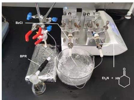
The flow reactor equipment consists of two pumps for reagent/solvent delivery. Before the start of the actual experiment, all reactors were primed with CH<sub>2</sub>Cl<sub>2</sub>. The Pump A was used to pump the mixture of the starting material **12** and Et<sub>3</sub>N which was 8 mL in total. The Pump B was used to pump BzCl. Solutions A and B were mixed at a T-piece and pumped through Reactor. A 5 bar back pressure regulator (BPR) was connected after
