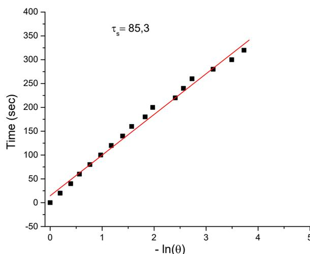
**Figure S6.** Linear relationship between time (sec) and  $\ln(\theta)$ , the slope is the time constant ( $\tau_s$ ).
