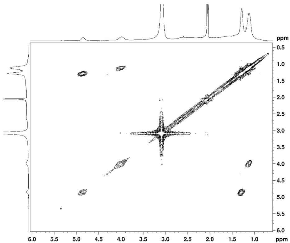
**Figure S2.** 2D-COSY NMR spectrum (acetone-d<sub>6</sub>, 297 K) of CDPs-PNM prepared by heating at 300 °C for 4 hrs.
