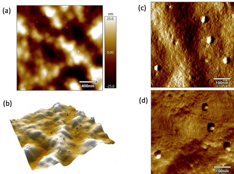
**Figure S3.** AFM images for CPDs-PNM on a 2  $\mu\text{m}$  (a: 2D height, z scale = 50 nm; b: 3D height) and a 500 nm (c: amplitude; d: phase) scan size area.
