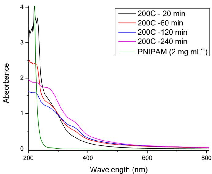
**Figure S4.** Optical absorption spectrum of CPDs-PNM dispersion at various carbonization process time.
