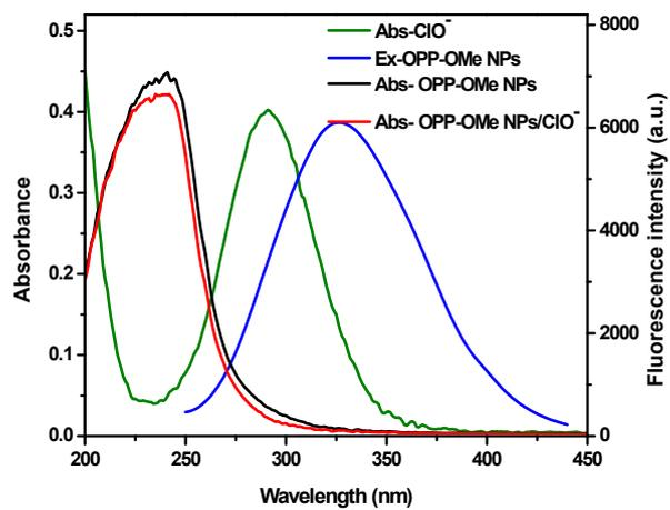
**Fig. S9** Absorption spectra of ClO<sup>-</sup> and OPP-OMe NPs before and after the addition of ClO<sup>-</sup>, and fluorescence excitation spectrum of OPP-OMe NPs.
