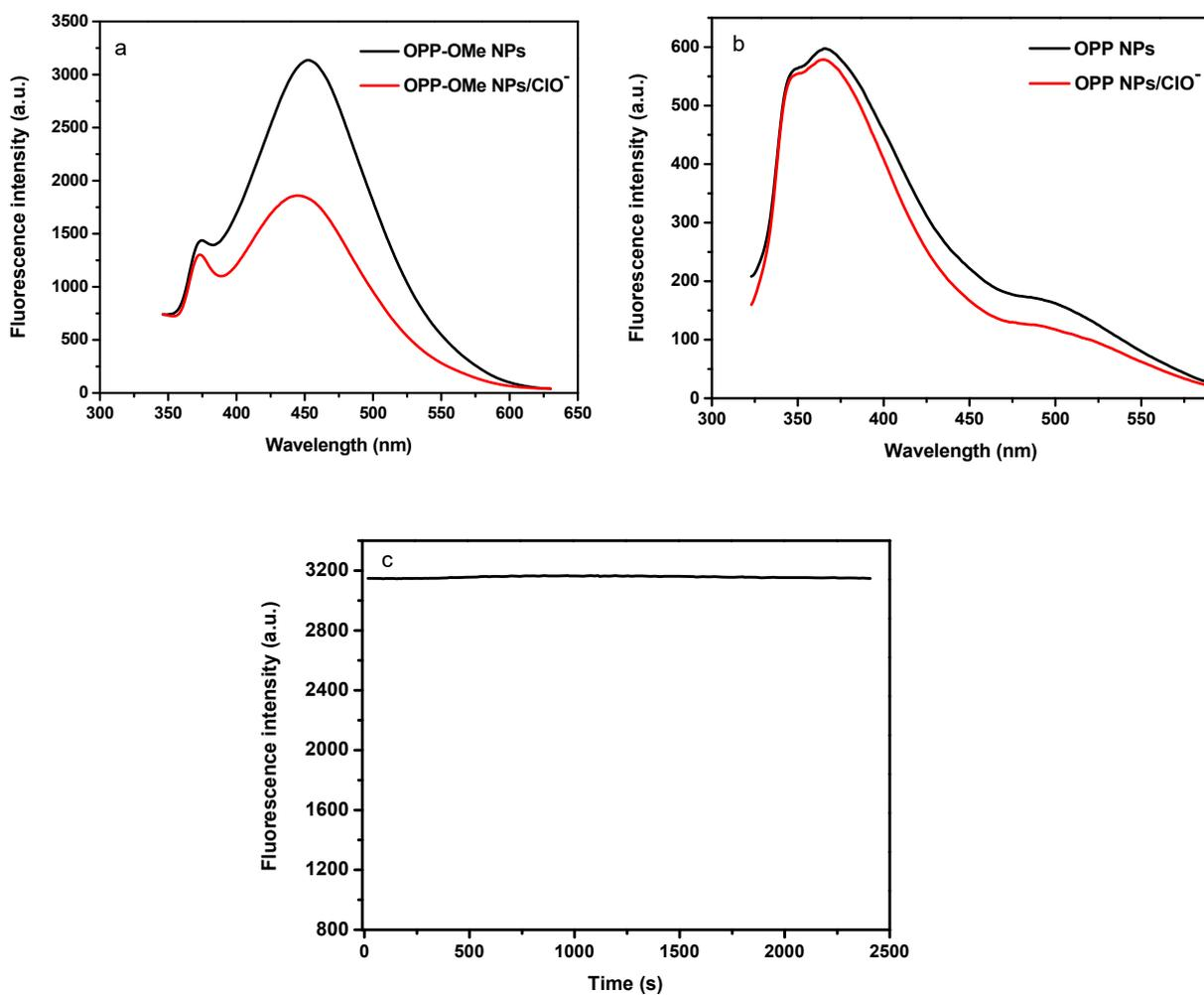
**Fig. S6** Fluorescence spectra of OPP-OMe NPs (a) and OPP NPs (b) in the absence and presence of  $\text{ClO}^-$ . (c) Photostability of OPP-OMe NPs in PBS buffer (pH = 7.4) upon irradiation at 327 nm for 40 min.
