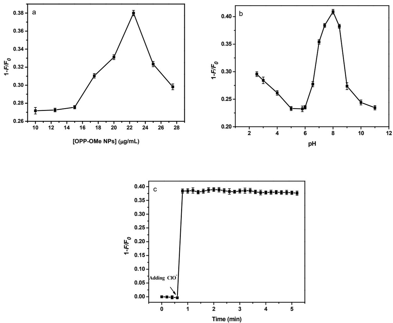
**Fig. S11** The influence of nanoprobe concentration (a), pH (b) and response time (c) on the fluorescence quenching efficiency.  $[\text{ClO}^-] = 5.0 \times 10^{-5} \text{ M}$ .  $F_0$  and  $F$  are the fluorescence intensity of OPP-OMe NPs before or after adding  $\text{ClO}^-$ , respectively.  $\lambda_{\text{ex}} = 327 \text{ nm}$ .
