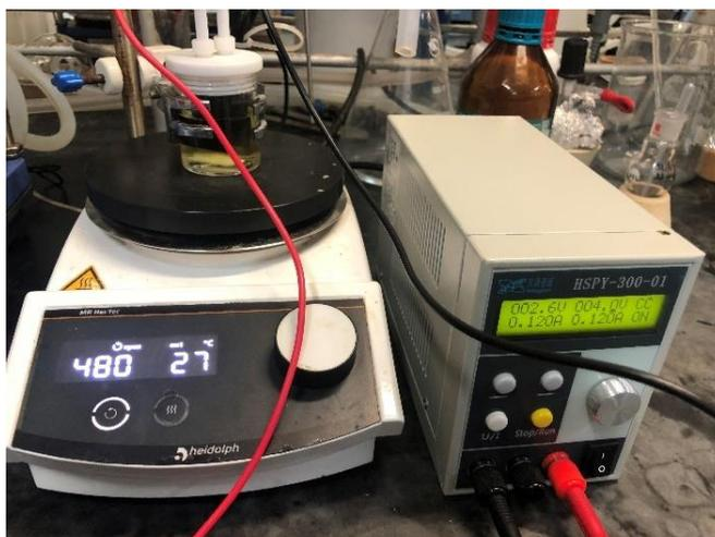
**(Left)** Graphite electrode (30 mm × 30 mm × 3 mm) and Platinum plate electrode (30 mm × 30 mm × 0.1 mm); **(Right)** The setup for the gram-scale reaction.
