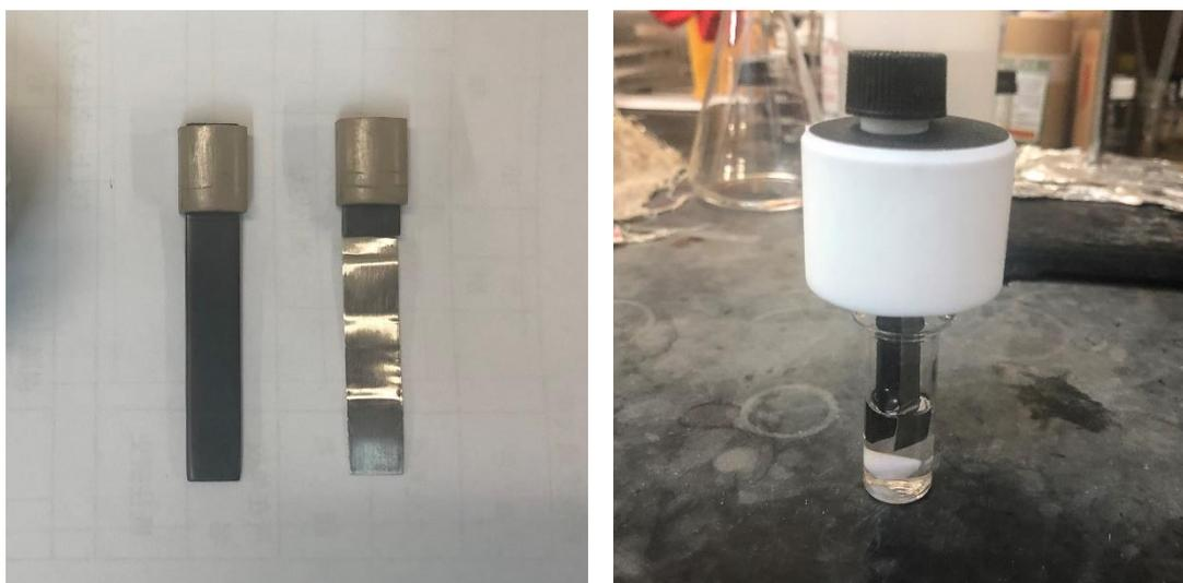
**(Left)** Graphite electrode (2 mm × 8 mm × 52 mm) and Platinum electrode (0.1 mm × 8 mm × 52 mm) were inserted into the holders on the connector; Platinum plate electrode was stuck with a section of graphite **(Right)** The electrode connector was plugged into the ElectraSyn Vial cap. (The distance between two electrodes is 0.5 cm)
