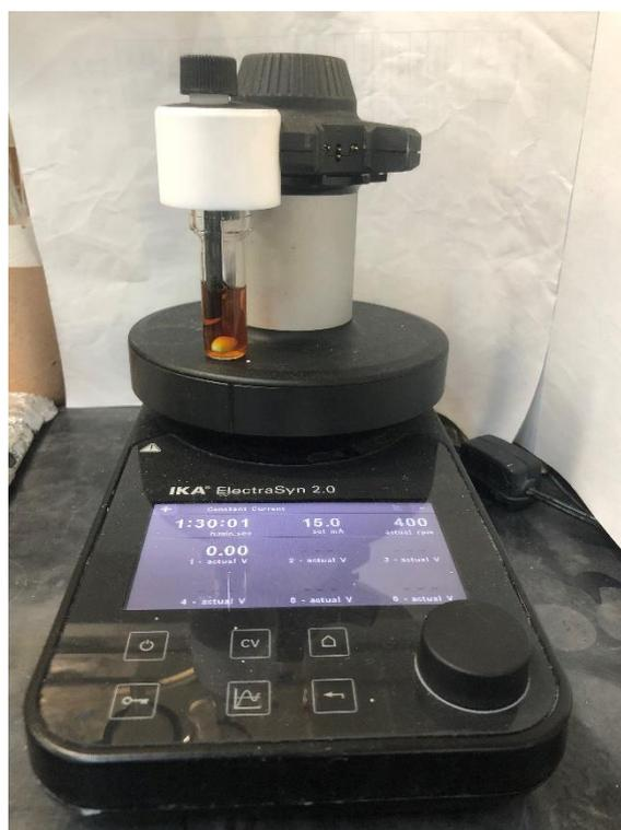
The electrochemical cell was plugged into ElectraSyn 2.0 equipped with IKA Carousel (six parallel reactions module available).
