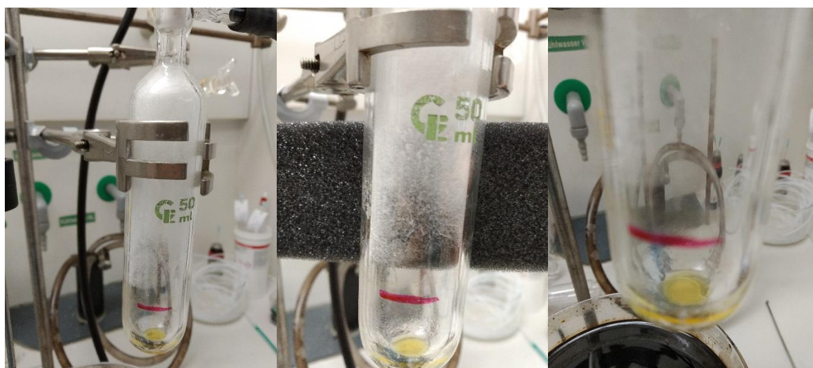
Figure S38. Spontaneous separation of the two product species 8 and 9 under the reaction conditions: Hydrodefluorinated borane 9 (white crystalline solid on the upper part of the vessel) and fluorodisiloxane 8 (yellow oily residue on the bottom part of the vessel).
