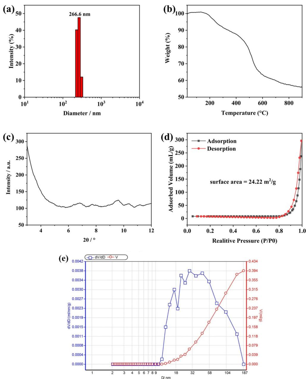
**Figure S16.** (a) DLS date of **P5COMs** crushed by ultrasonic cell disruptor at 25 °C. (b) Thermogravimetric (TG) analyses for **P5COMs** under N<sub>2</sub>. (c) Powder XRD patterns of experimental data of **P5COMs**. (d) Nitrogen sorption isotherm of **P5COMs**. black symbols: adsorption, red symbols: desorption. (e) Barrett-Joyner-Halenda (BJH) investigation of **P5COMs**.
