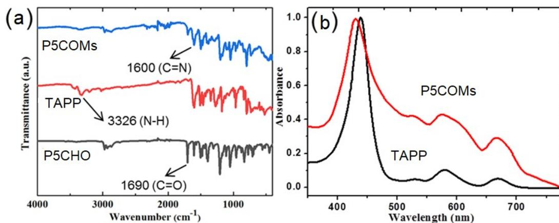
**Figure S14.** (a) FTIR spectra for **P5COMs** (top) in comparison with model compound **M** and corresponding monomers **P5CHO** and **TAPP**. (b) UV-Vis absorption spectra (DMSO, RT) of **TAPP**, **P5COMs** and **P5CHO**.
