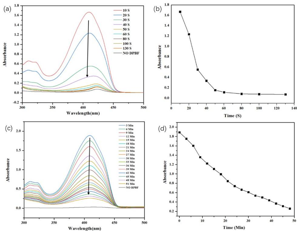
Figure 23. (a) UV-vis spectra of DPBF incubated with P5COMs under light irradiation, (b) The absorbance at 426 nm of (a) with different irradiation time, (c) UV-vis spectra of DPBF incubated with pure TAPP under light irradiation, (d) The absorbance at 426 nm of (c) with different irradiation time.  $[P5COMs] = [TAPP] = 0.01 \text{ mmol}$ , light:  $660 \text{ nm}$ ,  $1.0 \text{ W cm}^{-2}$ .
