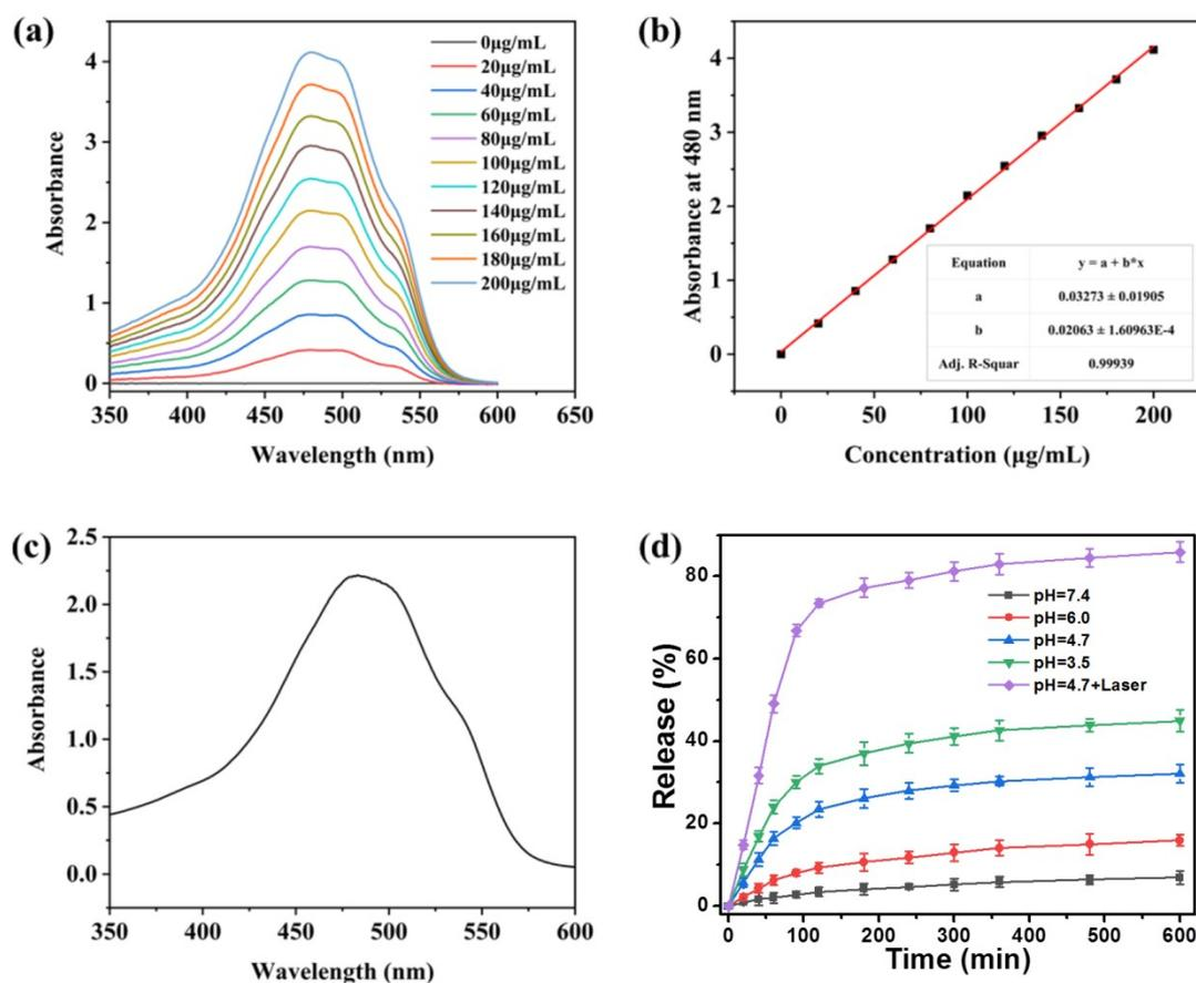
**Figure S20.** (a) UV-Vis absorption spectra (H<sub>2</sub>O, RT) of different concentrations of Dox. (b) Absorbance intensity at 480 nm as a function of the concentration of Dox in solution. (c) The UV-vis absorbance of the supernatant after Dox loading. (d) Drug release curves of P5COMs/FA-Py/Dox in PBS solutions of different pH values at 37° C.
