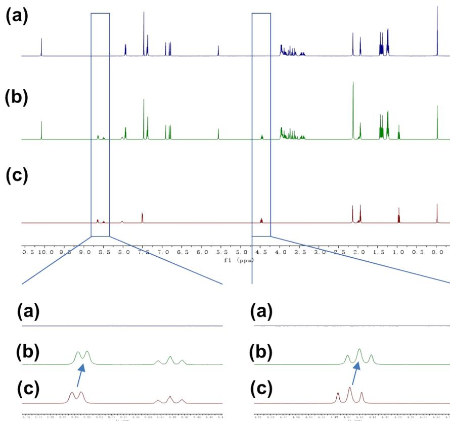
**Figure S13.**  $^1\text{H}$  NMR spectra (400 MHz,  $\text{CDCl}_3/\text{Acetonitrile-}D_3$ , 298 K) of (a) **P5CHO** (10.0 mM), (b) **P5CHO** + **G** ( $[\text{P5CHO}] = 10.0$  mM,  $[\text{G}] = 10.0$  mM), and (c) **G** (10.0 mM).
