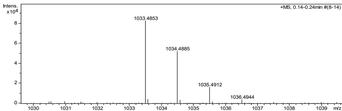
**Figure S3.** Mass spectra of **P5CHO** Calcd. for  $\text{C}_{65}\text{H}_{70}\text{O}_{10}\text{Na}$  ( $[\text{M}+\text{Na}]^+$ ): 1033.4867, found: 1033.4853.
