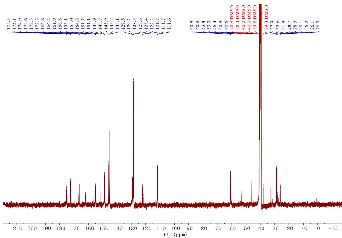
**Figure S12.** <sup>13</sup>C NMR spectra (100 MHz, 298 K, DMSO-*d*<sub>6</sub>) of FA-Py.
