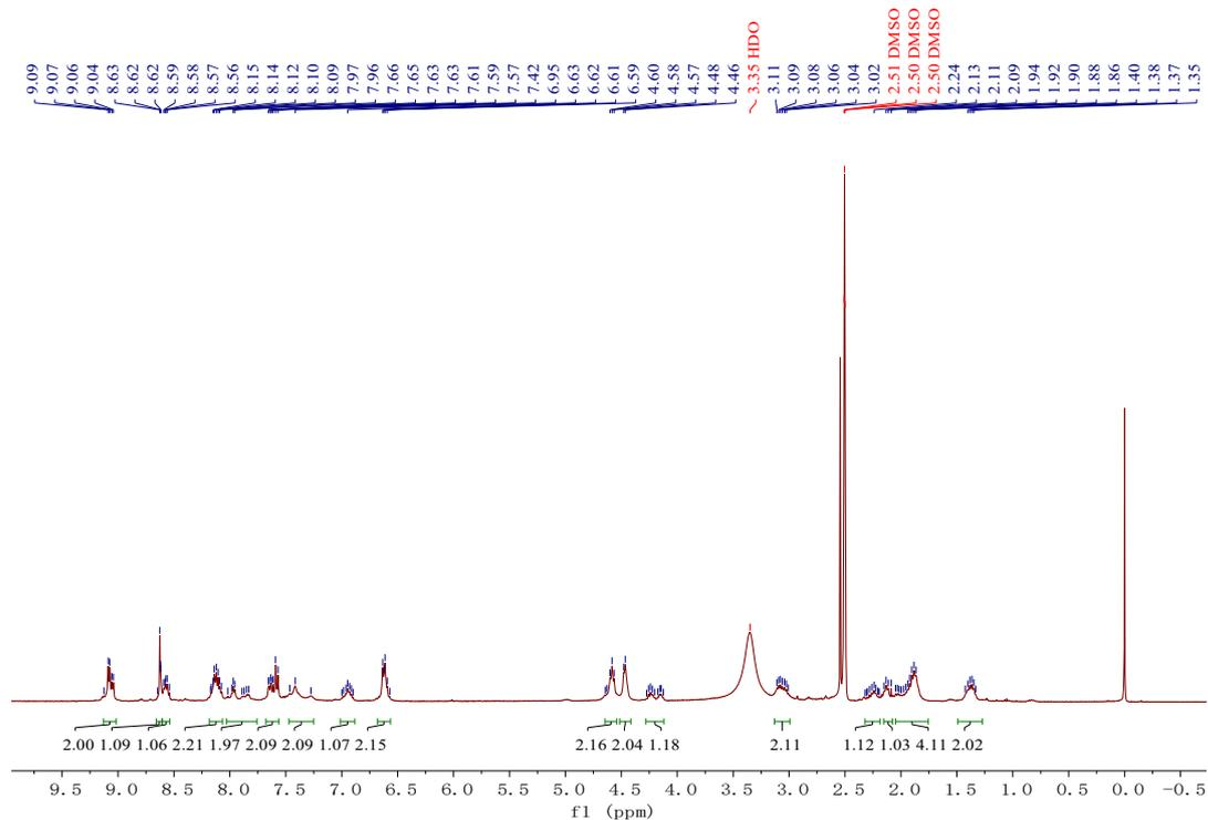
**Figure S11.** <sup>1</sup>H NMR (400 MHz, DMSO) spectrum of FA-Py.
