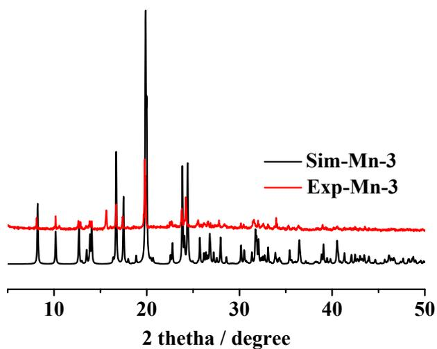
Figure S3. Powder X-ray diffractions of Mn-3.
