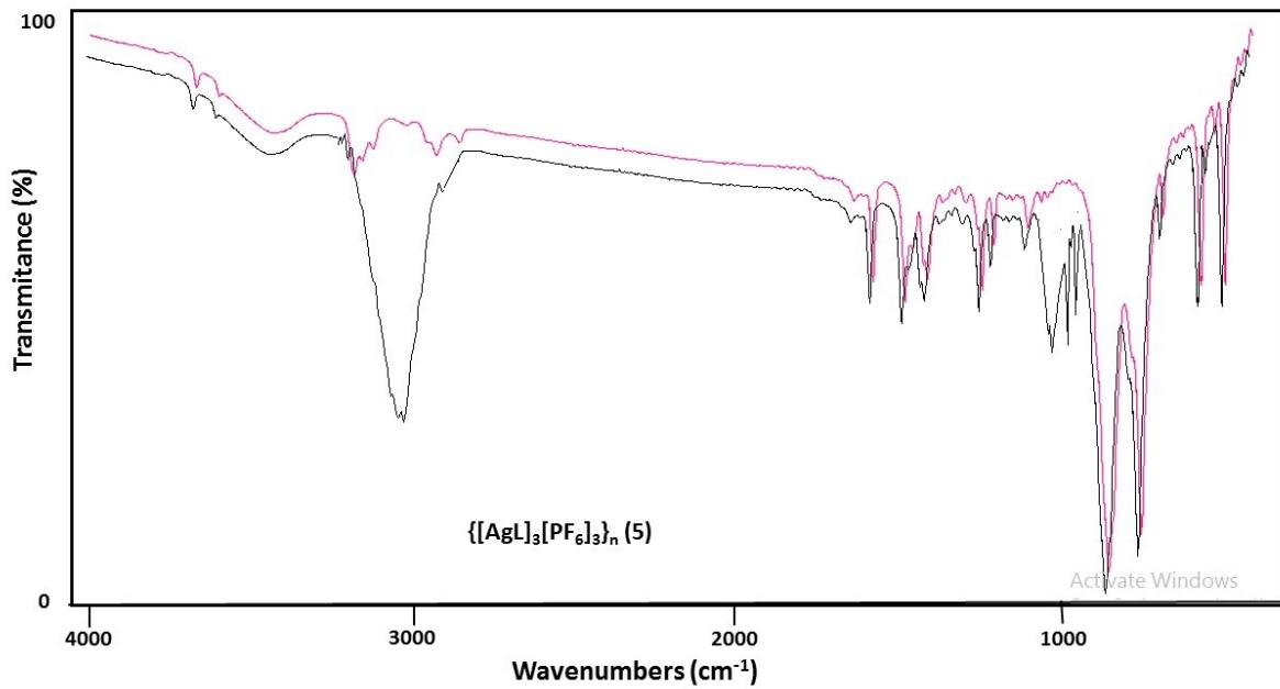
**Figure S4.** FT-IR spectra for coordination polymers **1-5** before (pink) and after (black) exposure to NH<sub>3</sub> gas.
