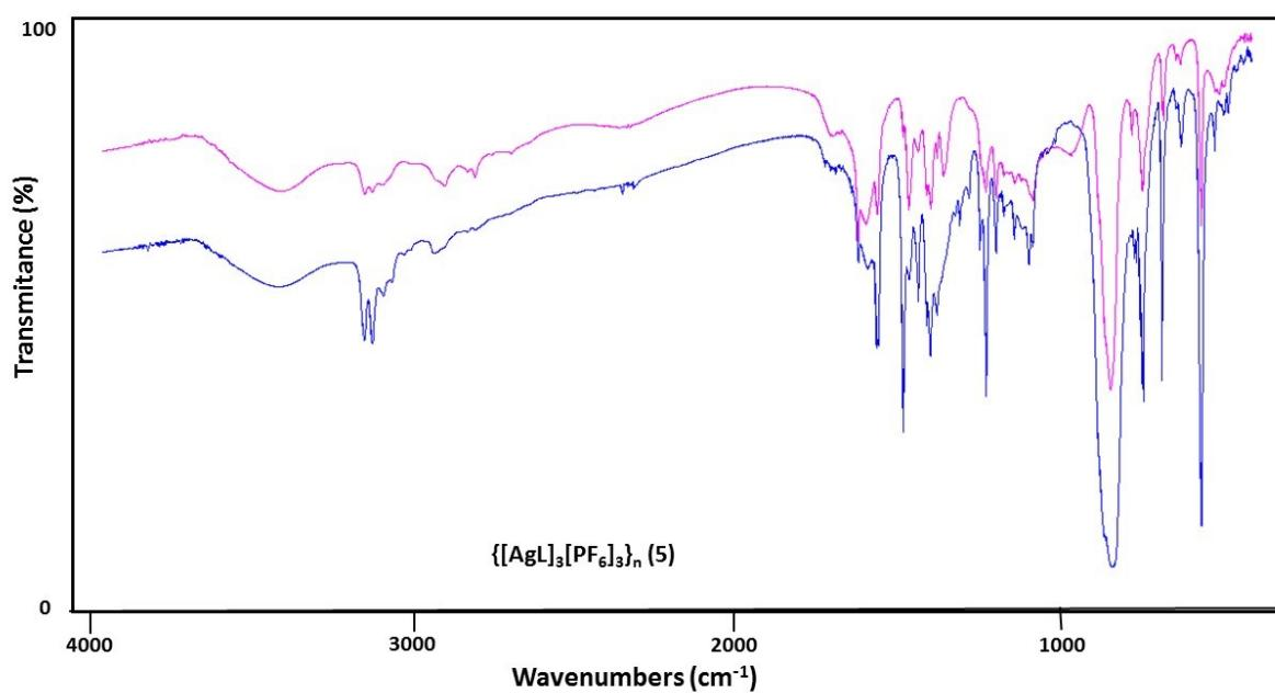
**Figure S2.** FT-IR spectra for coordination polymers **1-5** before (blue) and after (pink) exposure to H<sub>2</sub>S gas.
