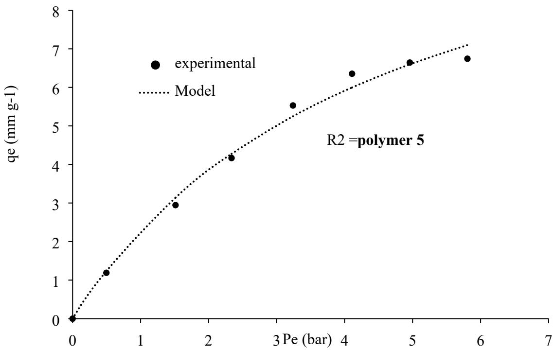
**Figure S1:** Volumetric adsorption isotherms of H<sub>2</sub>S measured at 278 K for polymer **1-5**.
