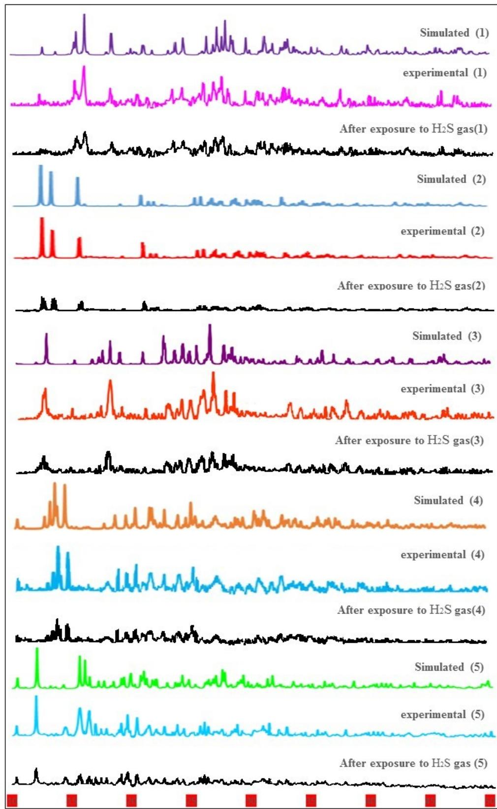
**Figure S3.** PXRD patterns for polymers **1-5** the simulated and experimental before and after exposure to H<sub>2</sub>S gas.
