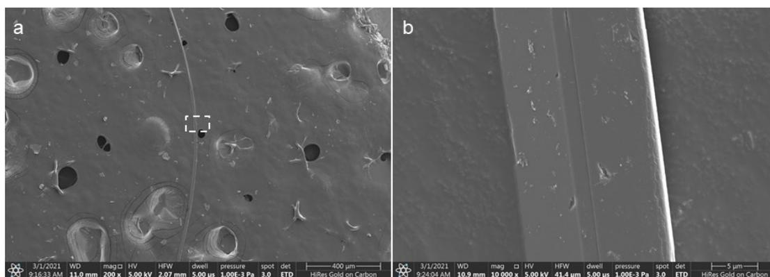
**Figure S7.** SEM images of the Cry-1R in bent state (a: 200X magnification b:10000X magnification)
