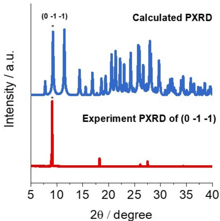
**Figure S6.** Calculated and experimental PXRD patterns of the Cry-1R (0-1-1) face.
