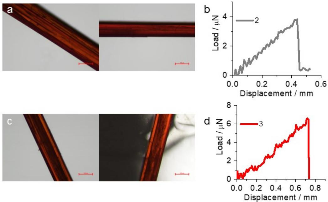
**Figure S3.** Microscope images (a,c) of the other 2 three-point bending experiments and the corresponding displacement-load curve (b,d)
