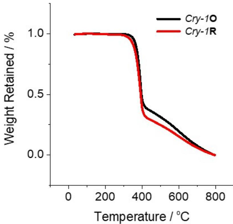
**Figure S2.** TGA analysis of *Cry-1O* and *Cry-1R*
