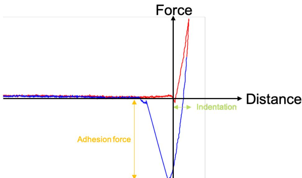
Figure S2: Example force-distance curve obtained on paracetamol exposed to a water-ethanol mixture. The indentation is the distance the tip travels into the surface before reaching the force limit, while adhesion force is the force required to retract the tip.
