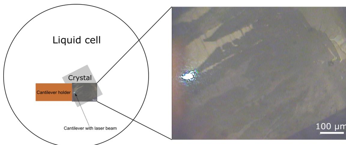
Figure S1: A schematic of the liquid cell arrangement (left) shows the cantilever placement on the crystal. An optical image (right) of the tip placement on the crystal surface is shown with a scale bar.
