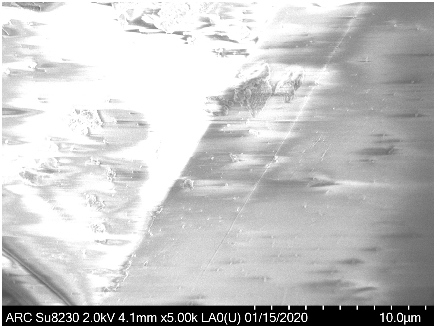
Figure S6. 3MOT loaded in hexanes and heated does not show polymer nodules or coating on the HKUST-1 surface.
