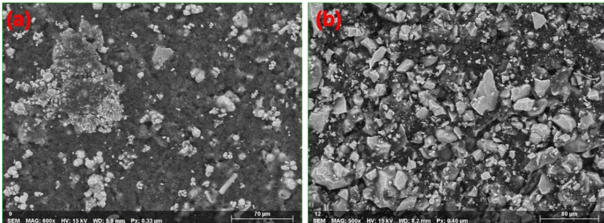
*Figure s4 SEM images of (a) Sc<sub>2</sub>Mo<sub>3</sub>O<sub>12</sub> electrode and (b) lithium discharged Sc<sub>2</sub>Mo<sub>3</sub>O<sub>12</sub>.*
