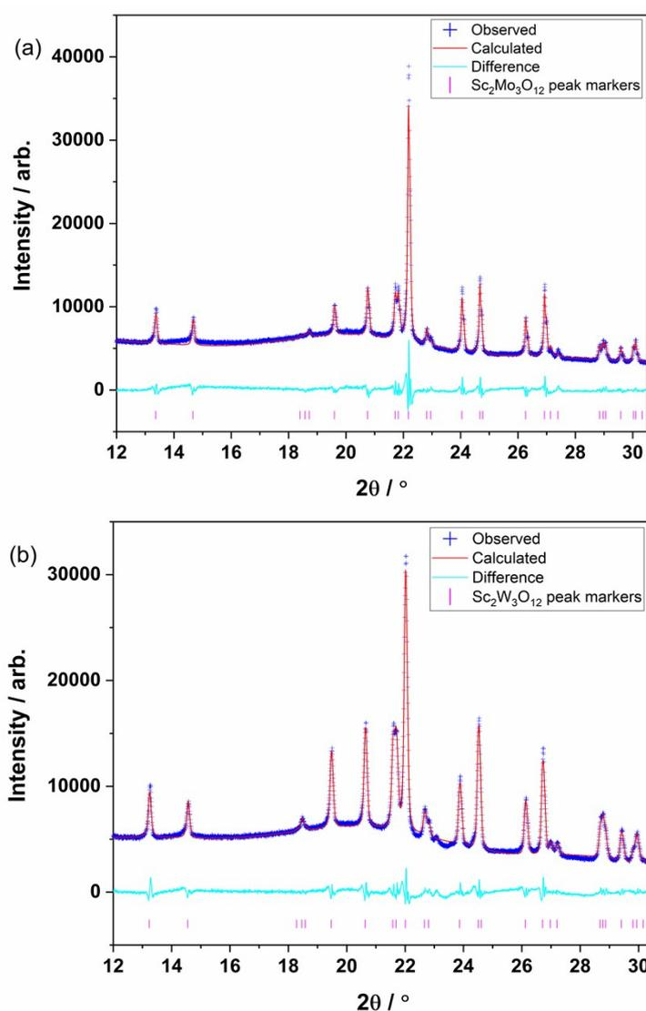
Figure S1 XRD data of (a) lithium discharged  $\text{Sc}_2\text{Mo}_3\text{O}_{12}$  at 1.7 V (b) lithium discharged  $\text{Sc}_2\text{W}_3\text{O}_{12}$  at 1.3 V.
