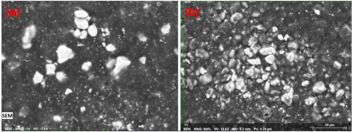
*Figure s5 SEM images of (a)  $Sc_2W_3O_{12}$  electrode and (b) lithium discharged  $Sc_2W_3O_{12}$ .*
