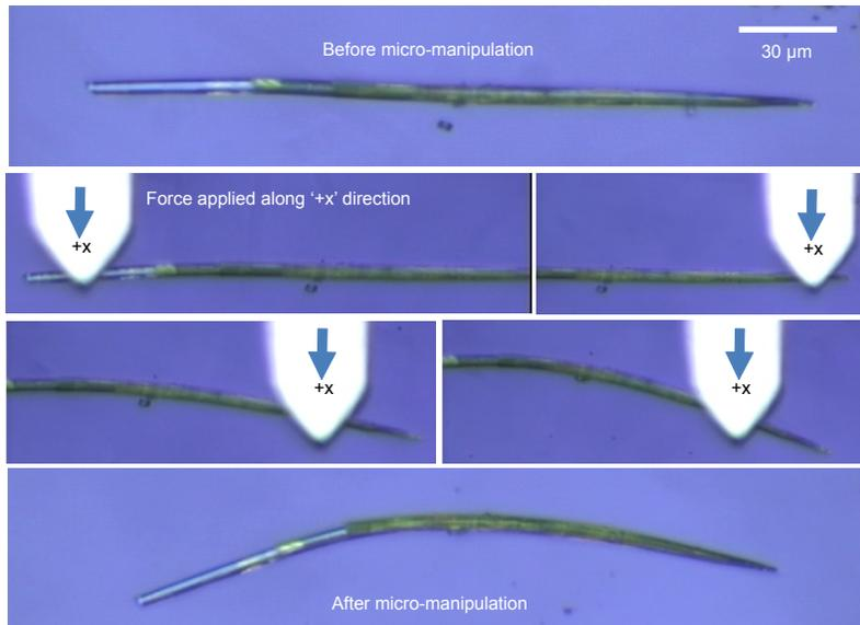
**Figure S2.** Micromanipulation of PTX-2CF<sub>3</sub>.
