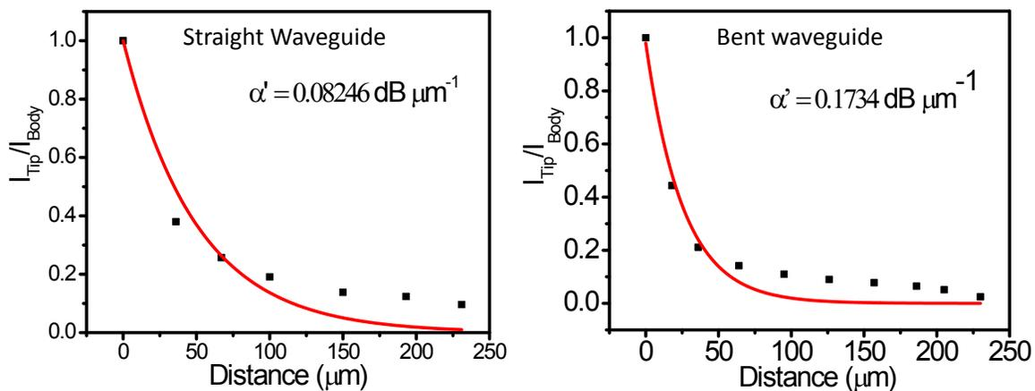
**Figure S3.** Optical loss fitting curves for straight and bent waveguides of **PTX-2CF<sub>3</sub>**.
