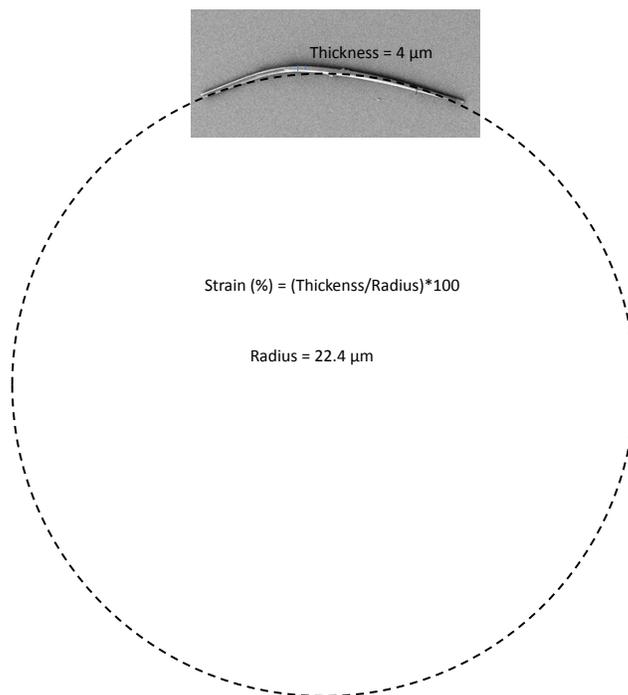
**Figure S4.** Strain caused due to bending of **PTX-2CF<sub>3</sub>** straight crystal with AFM tip.
