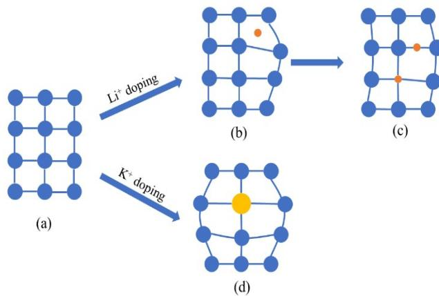
**Fig. S1** Schematic illustration for the influence and formation mechanism of alkali ions introduced in  $\text{NaYF}_4$  nanocrystals. (a) untreated  $\text{NaYF}_4$  nanocrystals (b)  $\text{Li}^+$  ions enter the gap of  $\text{NaYF}_4$  nanocrystals (c)  $\text{Li}^+$  ions enter the gap of  $\text{NaYF}_4$  nanocrystals and occupy the lattice position (d)  $\text{K}^+$  ions occupy the lattice position of  $\text{NaYF}_4$  nanocrystals
