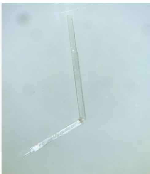
**Fig. S2** Crystal **1** was brittle when the stress was applied to the (001) face.
