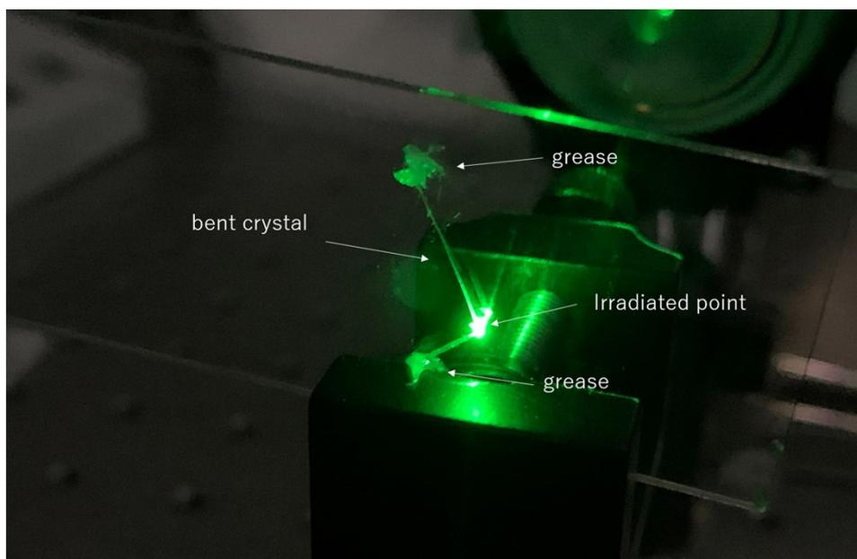
**Fig. S14** The femtosecond near-IR pulses ( $\lambda_{\text{em}} = 1064 \text{ nm}$ ) were applied to the bent position of **1** in the SHG measurement. The focus point is shown with a green light.
