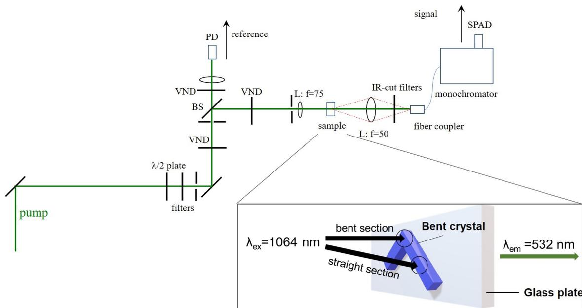
**Fig. S13** Schematic diagram of equipment configuration and sampling in the SHG measurement.
