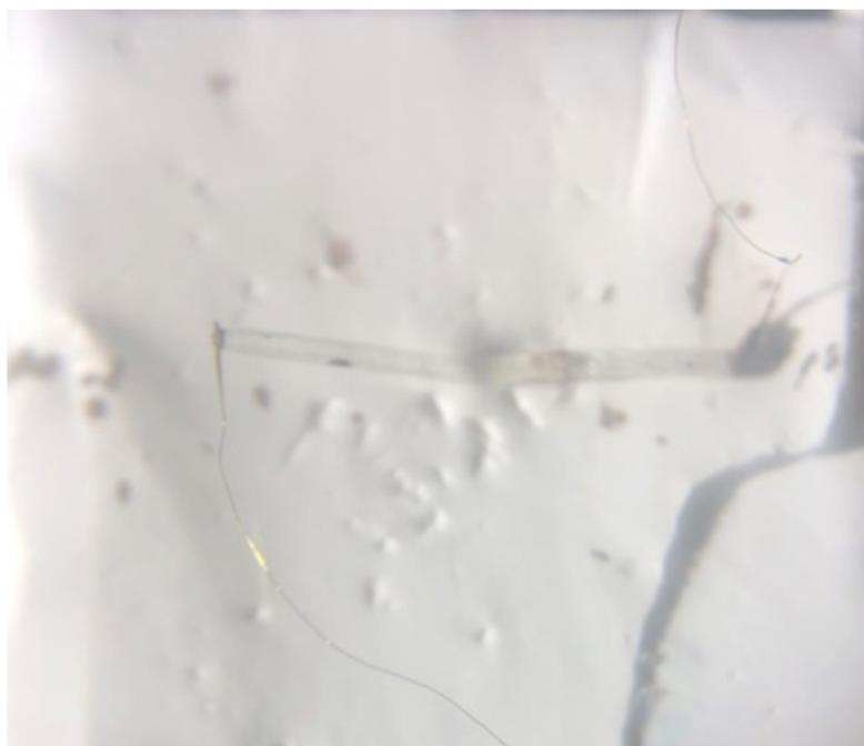
**Fig. S10** Plastically bent crystal (6 mm length x 0.1 mm thickness x 0.3 mm width) for measurement of
