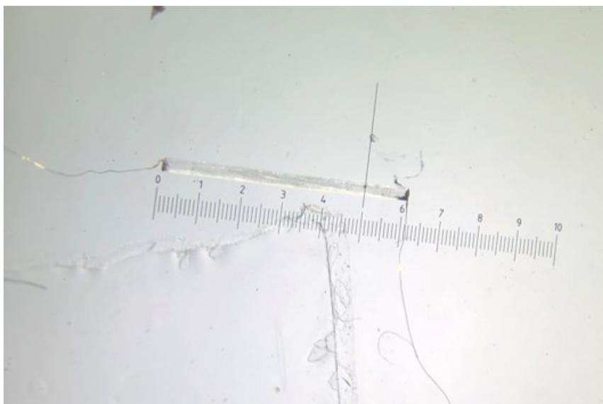
**Fig. S9** Straight crystal (6 mm length x 0.1 mm thickness x 0.3 mm width) for measurement of dielectric constants by Wayne Kerr 6440B LCR meter. Both ends of a single crystal were attached to gold wires.
