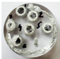
Fig. S1 (\text{Mn,Ni,Cu})_3\text{BO}_5 and (\text{Mn,Ni})_3\text{BO}_5 samples with different composition, molded into plastic and mechanically polished for EDX analysis.
