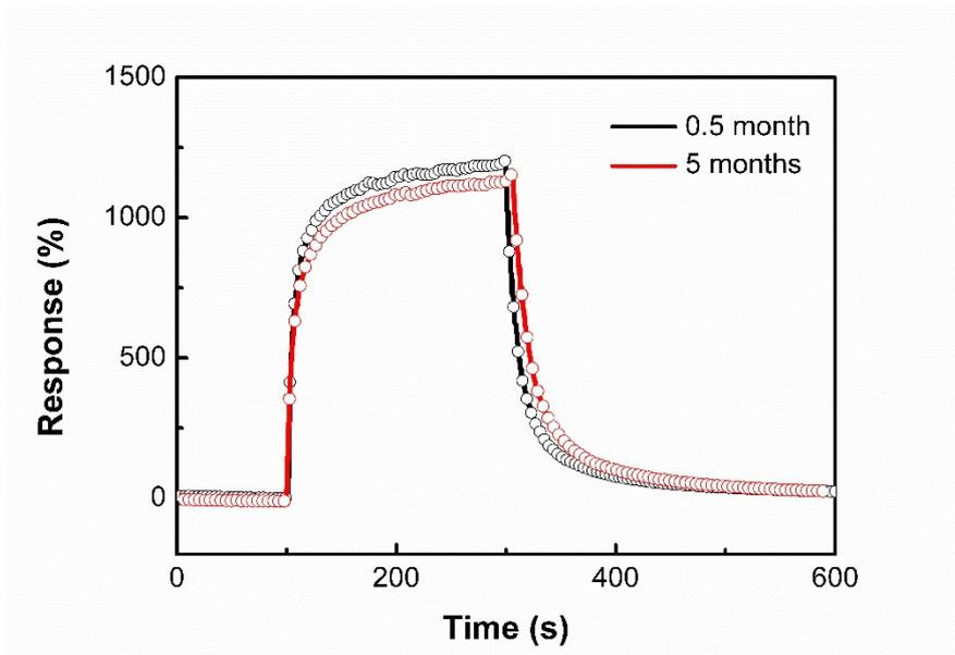
**Fig. S8** The response and recovery curve of the SnSe<sub>2</sub> sensor after aging 0.5 month and 5 months to 10 ppm NO<sub>2</sub> at room-temperature.
