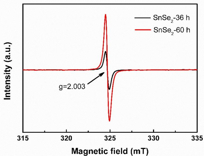
**Fig. S11** EPR spectra of SnSe<sub>2</sub>-36h and SnSe<sub>2</sub>-60h samples.
