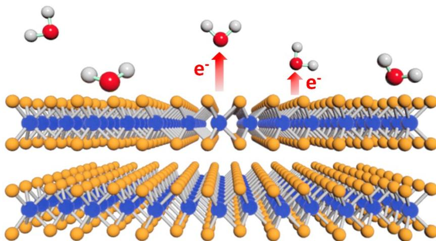
**Fig. S9** Sensing mechanism of SnSe<sub>2</sub> exposed to NO<sub>2</sub>.
