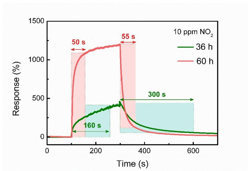
**Fig. S5** Response/recovery curves of SnSe<sub>2</sub>-36h and SnSe<sub>2</sub>-60h to 10 ppm NO<sub>2</sub>.
