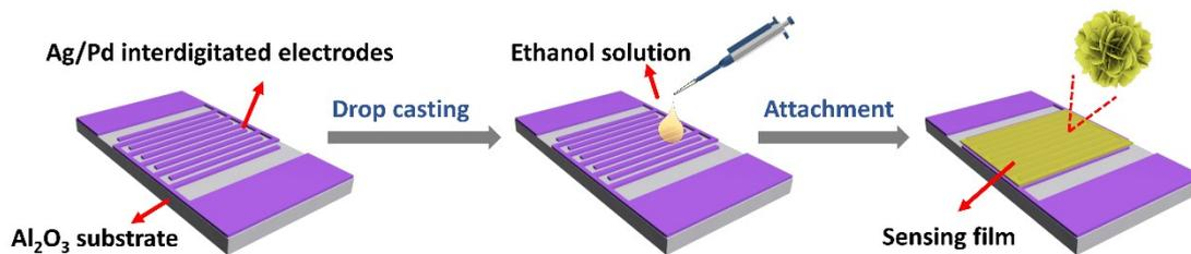
**Fig. S1** Fabricated technological process diagram of gas sensor.
