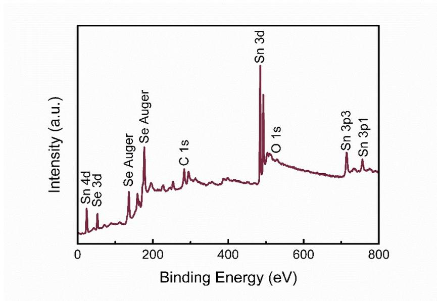
**Fig. S4** Survey XPS spectrum of the SnSe<sub>2</sub> hierarchical nanostructures.
