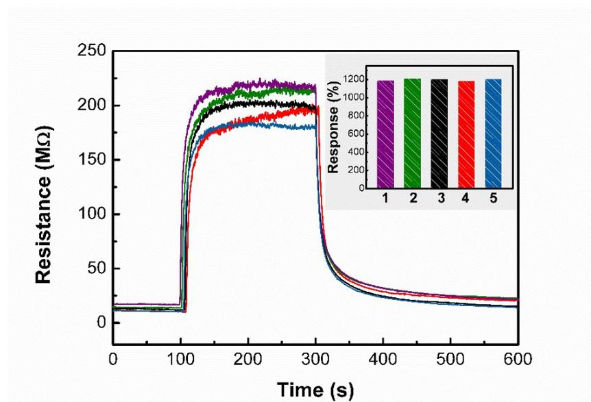
**Fig. S7** The resistance variations and sensing response (inset) of the SnSe<sub>2</sub> hierarchical structures toward 10 ppm NO<sub>2</sub> on 5 different sensing devices.
