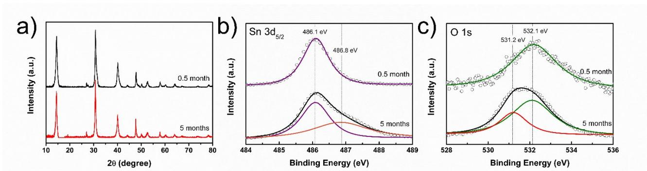
**Fig. S12** (a) XRD patterns and XPS spectra of (b) Sn 3d orbital and (c) O 1s orbital of the SnSe<sub>2</sub> sensor after aging 0.5 month and 5 months.
