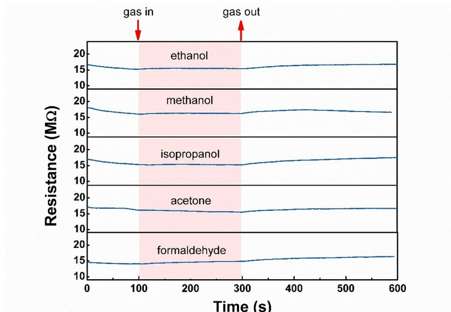
**Fig. S6** Selectivity response of SnSe<sub>2</sub> sensor toward 100 ppm VOCs (ethanol, methanol, isopropanol, acetone, and formaldehyde).
