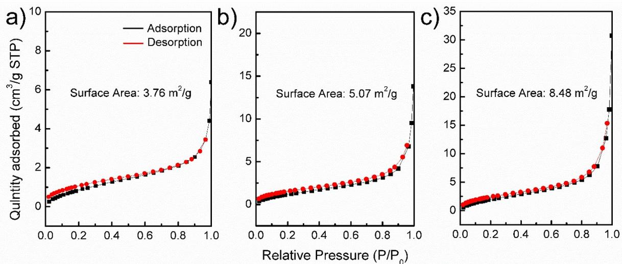
**Fig. S10** Nitrogen adsorption/desorption isotherms of (a) SnSe<sub>2</sub>-36h, (b) SnSe<sub>2</sub>-48h and (c) SnSe<sub>2</sub>-60h samples.
