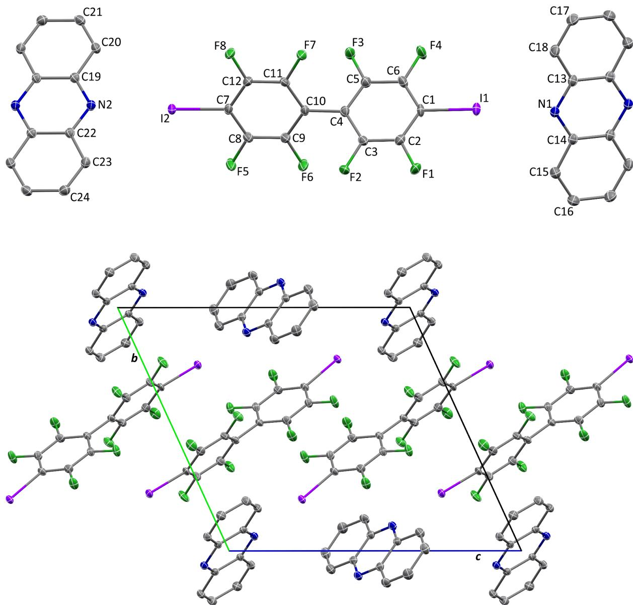
**Figure SI49.** Solid-state structure (top) and unit cell packing (bottom, viewed down the *a* axis) of  $(\text{I}_2\text{F}_8\text{bph})(\text{phenaz})$ . Atomic displacement ellipsoids are shown at the 50% probability level. Hydrogen atoms have been omitted for clarity.
