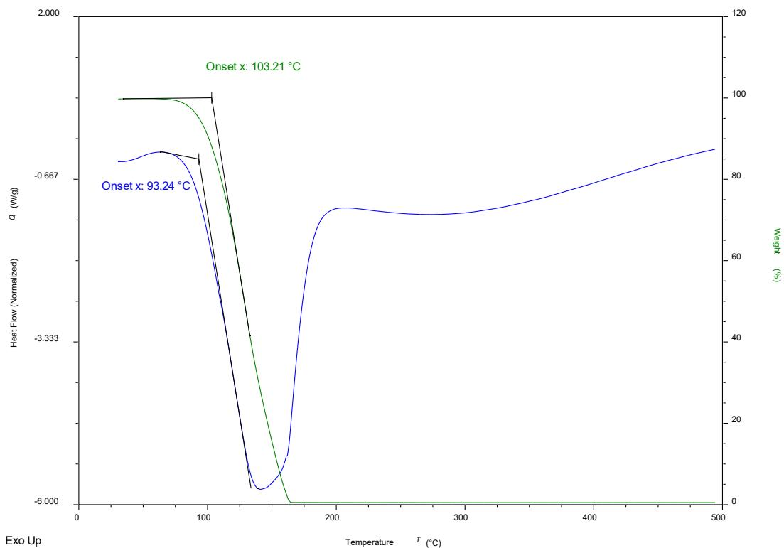
**Figure SI18.** SDT of  $(\text{I}_2\text{F}_4\text{bz})(4,4'\text{-Me}_2\text{-}2,2'\text{-bipy})$
