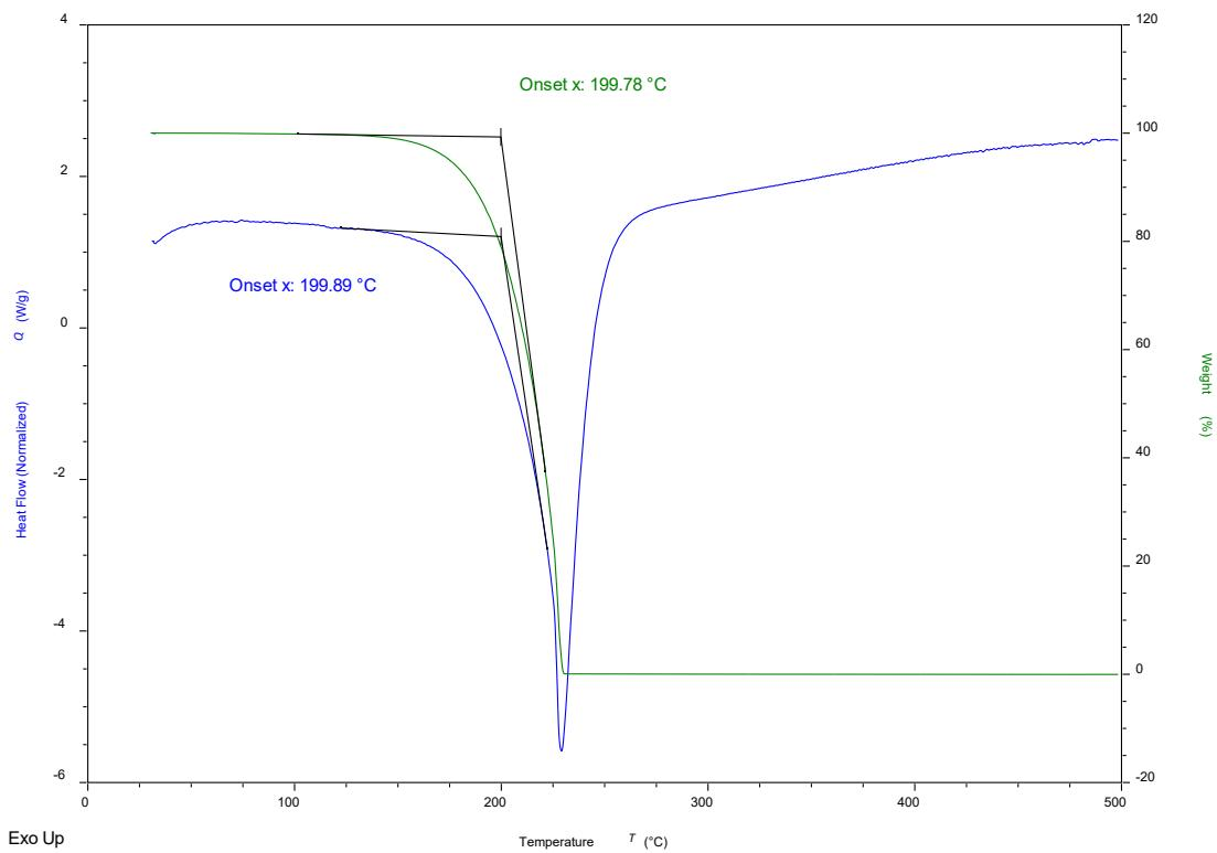
**Figure SI27.** SDT of  $(\text{I}_2\text{F}_8\text{bph})(\text{DABCO})$
