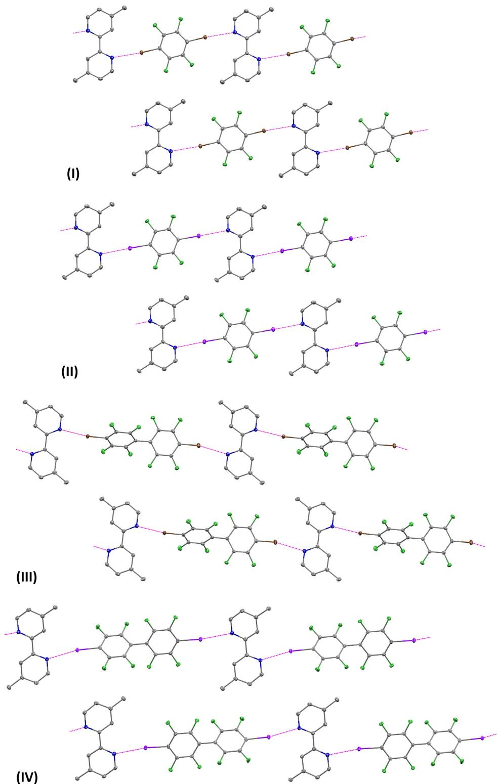
**Figure SI33.** Neighboring 1-d halogen bonding chains in  $(Br_2F_4bz)(4,4'-Me_2-2,2'-bipy)$  (I),  $(I_2F_4bz)(4,4'-Me_2-2,2'-bipy)$  (II),  $(Br_2F_8bph)(4,4'-Me_2-2,2'-bipy)$  (III), and  $(I_2F_8bph)(4,4'-Me_2-2,2'-bipy)$  (IV). Halogen bonds are shown as magenta dashed lines.
