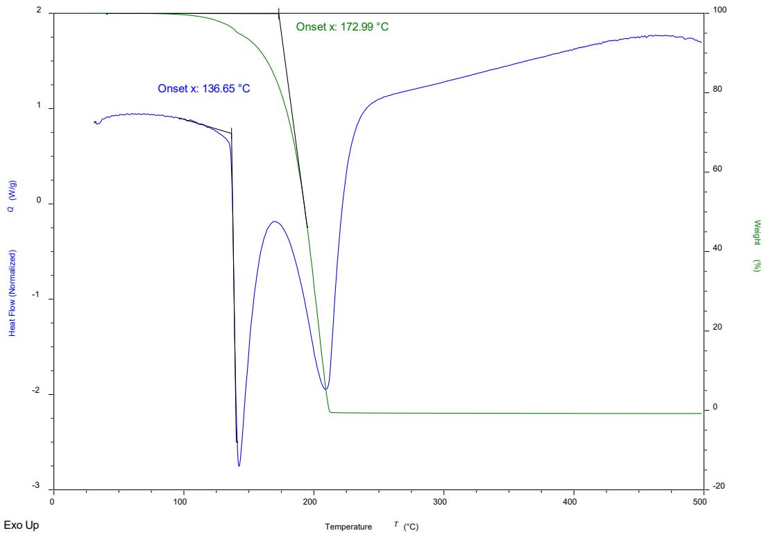
**Figure SI26.** SDT of  $(Br_2F_8bph)(DABCO)$
