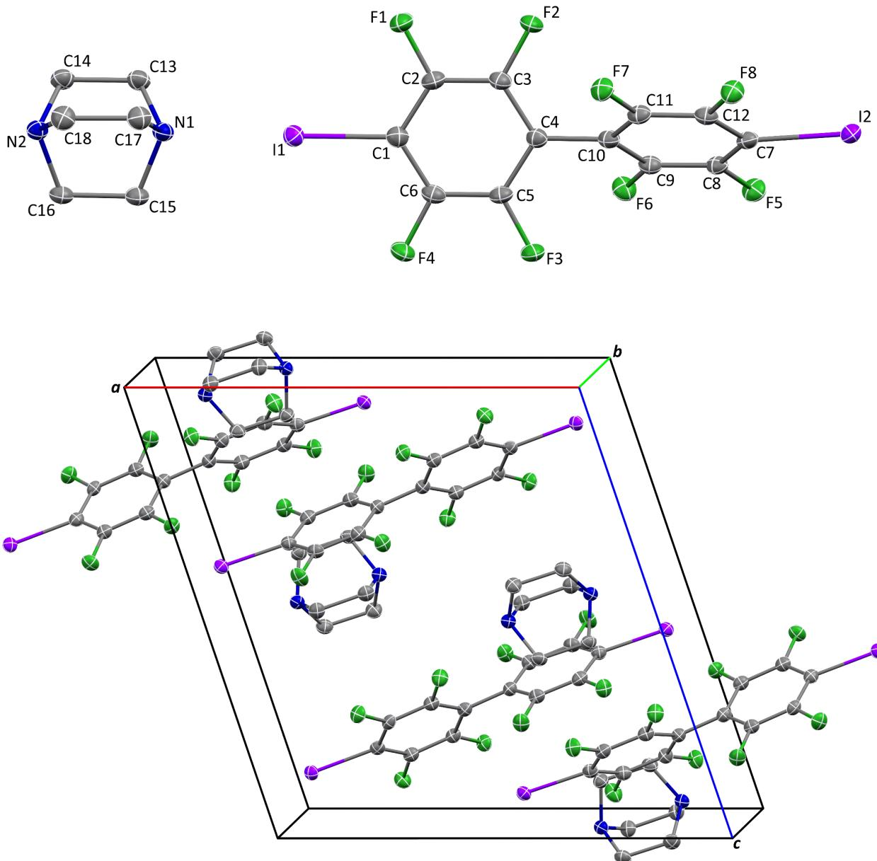
**Figure SI63.** Solid-state structure (top) and unit cell packing (bottom) of  $(\text{I}_2\text{F}_8\text{bph})(\text{DABCO})$ . Atomic displacement ellipsoids are shown at the 50% probability level. Hydrogen atoms have been omitted for clarity.
