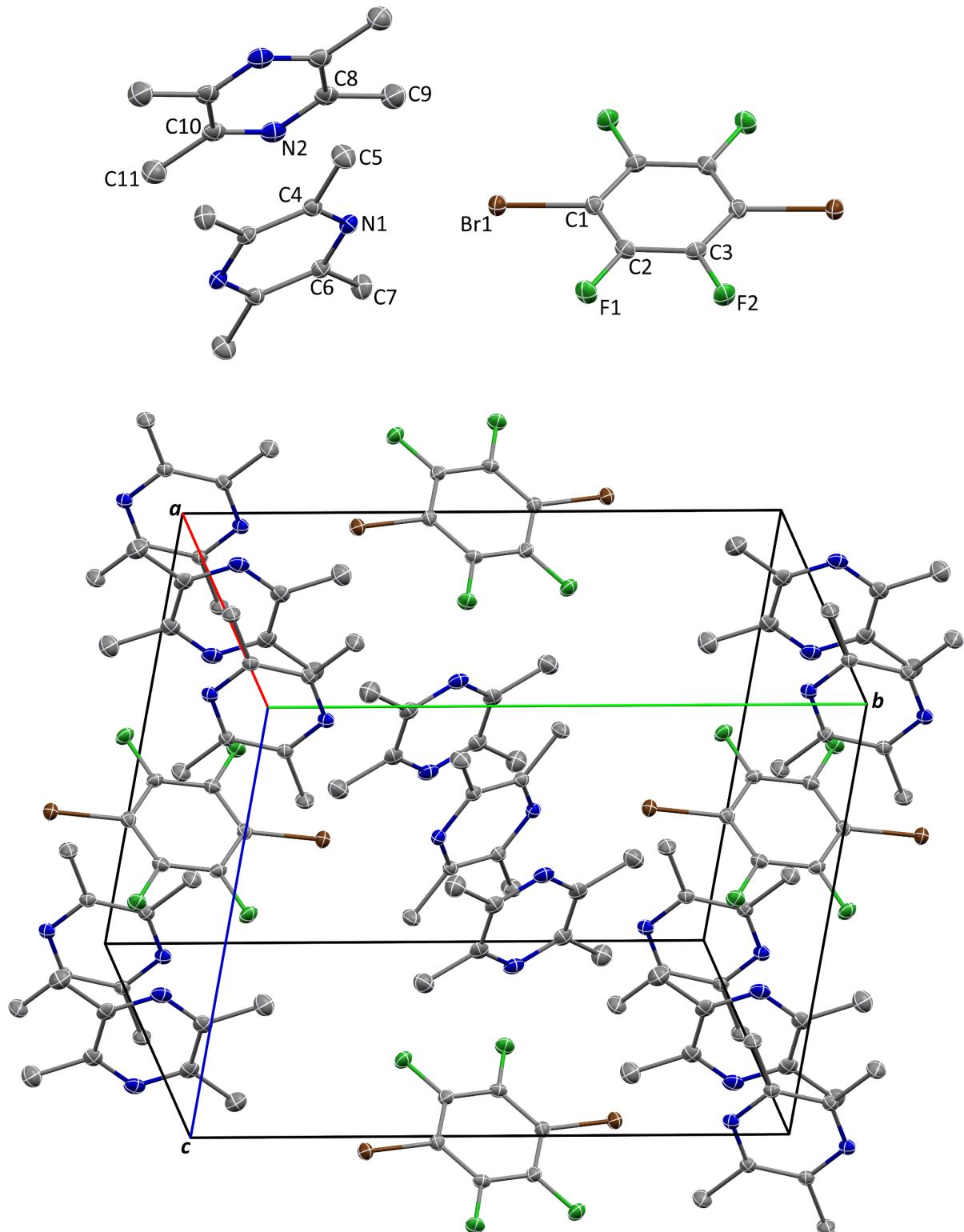
**Figure SI42.** Solid-state structure (top) and unit cell packing (bottom) of  $(\text{Br}_2\text{Fbz})_2(\text{Me}_4\text{pyrz})$ . Atomic displacement ellipsoids are shown at the 50% probability level. Hydrogen atoms have been omitted for clarity.
