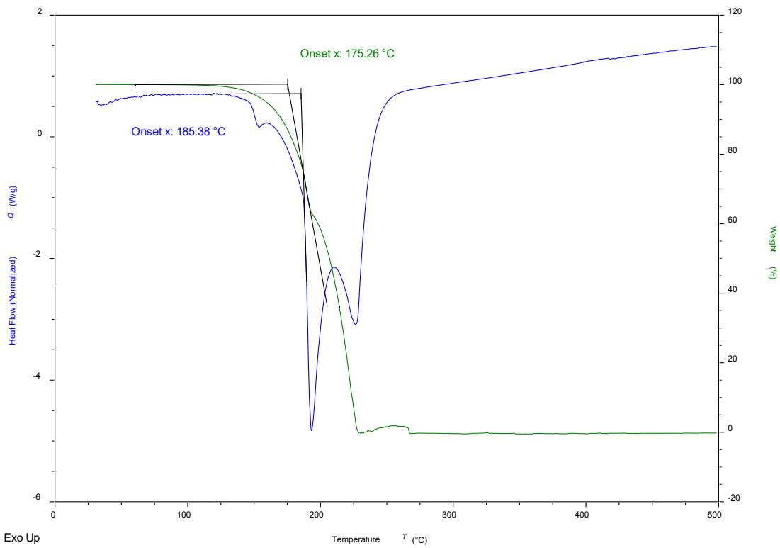
**Figure SI25.** SDT of  $(I_2F_8bph)(dpe)$
