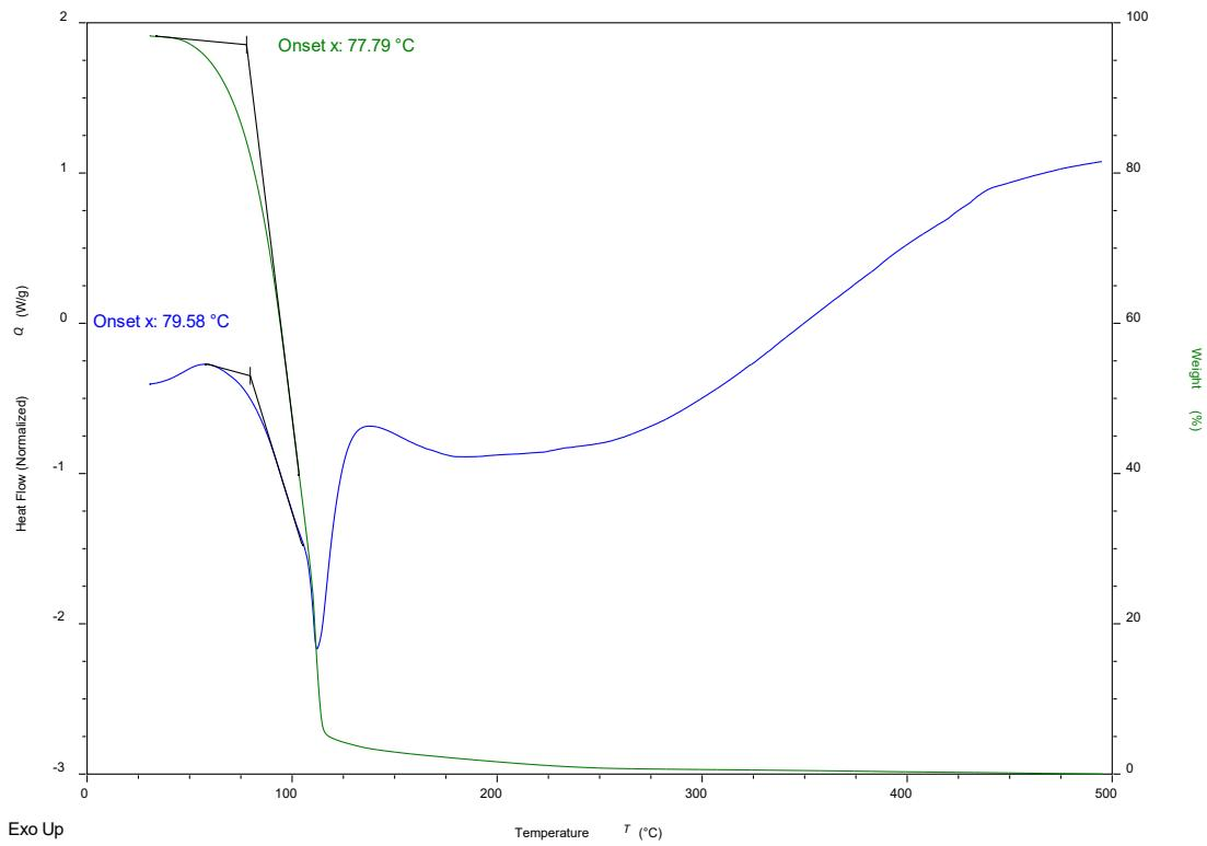
**Figure SI17.** SDT of  $(\text{Br}_2\text{F}_4\text{bz})(4,4'\text{-Me}_2\text{-}2,2'\text{-bipy})$
