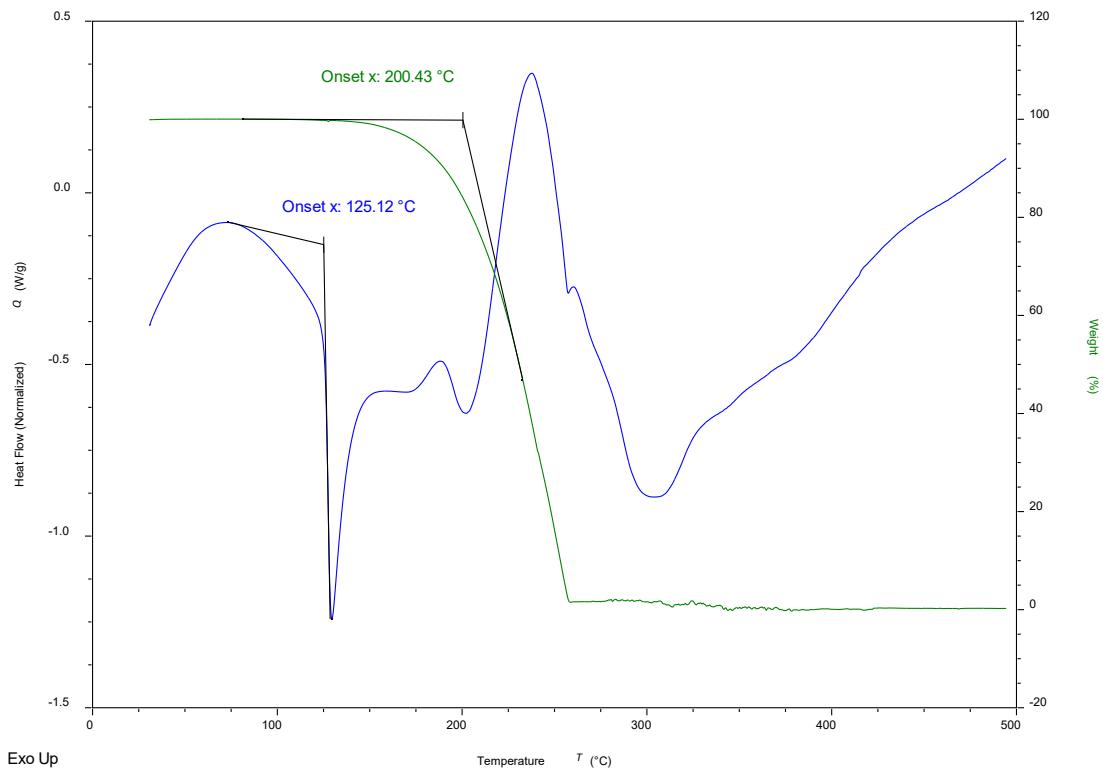
**Figure SI14.** SDT of  $(Br_2F_4bz)(2,2'\text{-bipy})$
