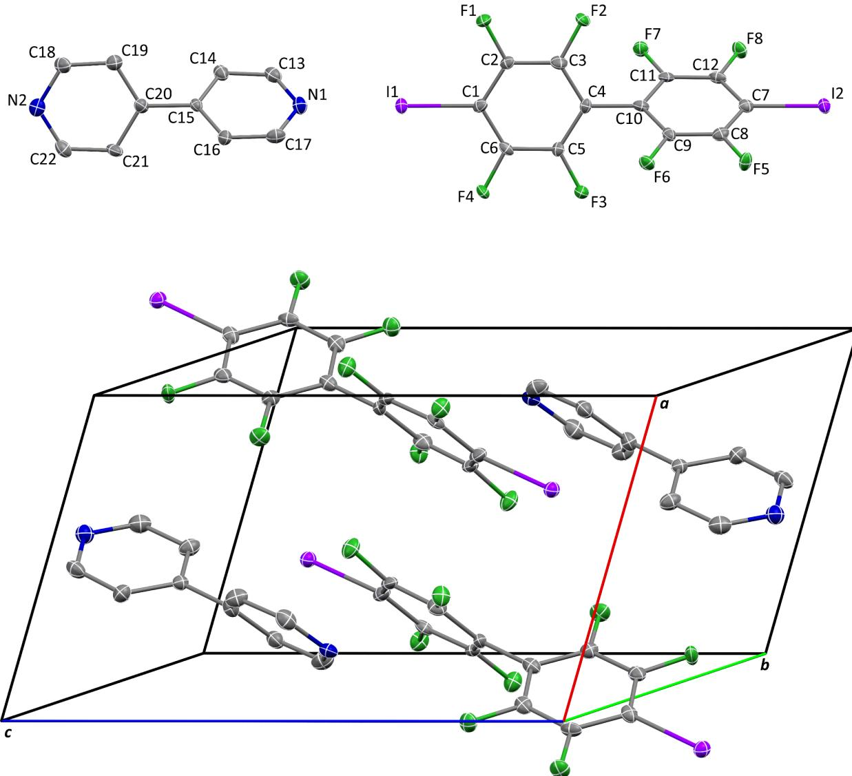
**Figure SI57.** Solid-state structure (top) and unit cell packing (bottom) of  $(\text{I}_2\text{F}_8\text{bph})(4,4'\text{-bipy})$ . Atomic displacement ellipsoids are shown at the 50% probability level. Hydrogen atoms have been omitted for clarity.
