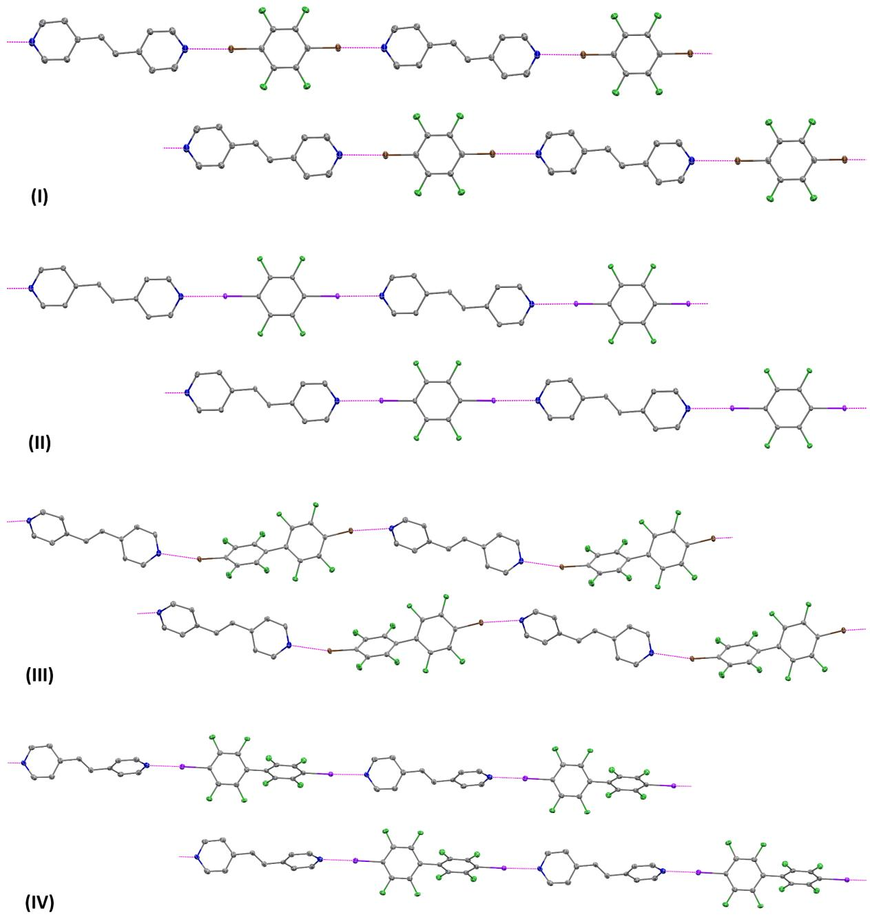
**Figure SI35.** Neighboring 1-d halogen bonding chains in  $(\text{Br}_2\text{F}_4\text{bz})(\text{dpe})$  (I),  $(\text{I}_2\text{F}_4\text{bz})(\text{dpe})$  (II),  $(\text{Br}_2\text{F}_8\text{bph})(\text{dpe})$  (III), and  $(\text{I}_2\text{F}_8\text{bph})(\text{dpe})$  (IV). Halogen bonds are shown as magenta dashed lines.
