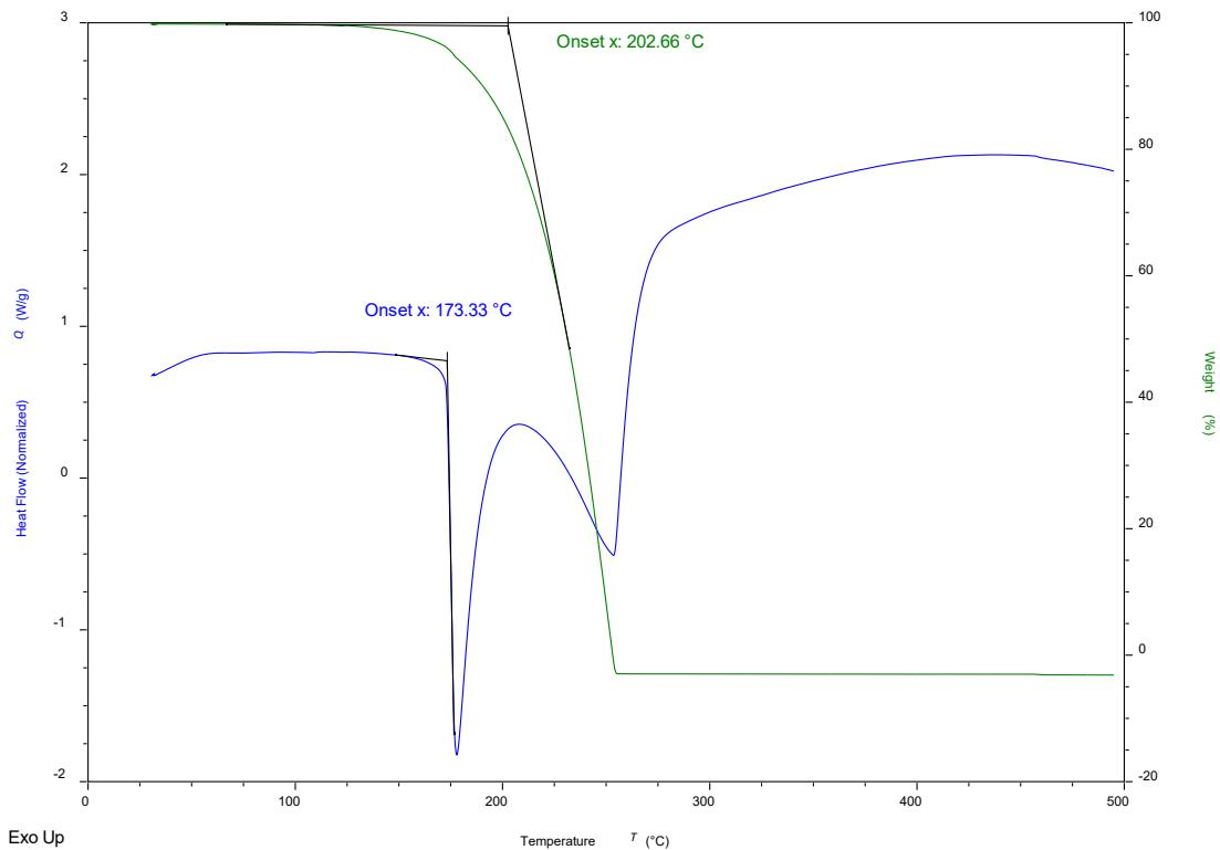
**Figure SI8.** SDT of  $(\text{I}_2\text{F}_8\text{bph})(\text{Me}_4\text{pyrz})$
