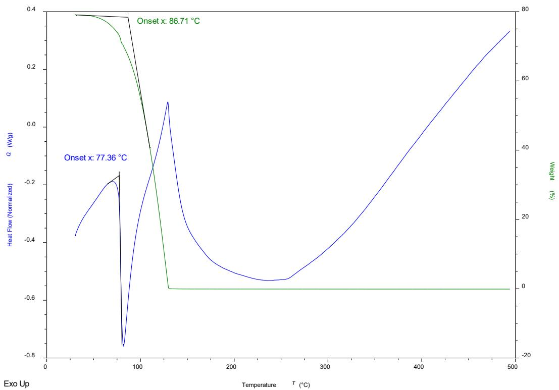
**Figure SI1.** SDT of  $(\text{Br}_2\text{F}_4\text{bz})(\text{Me}_2\text{pyrz})$
