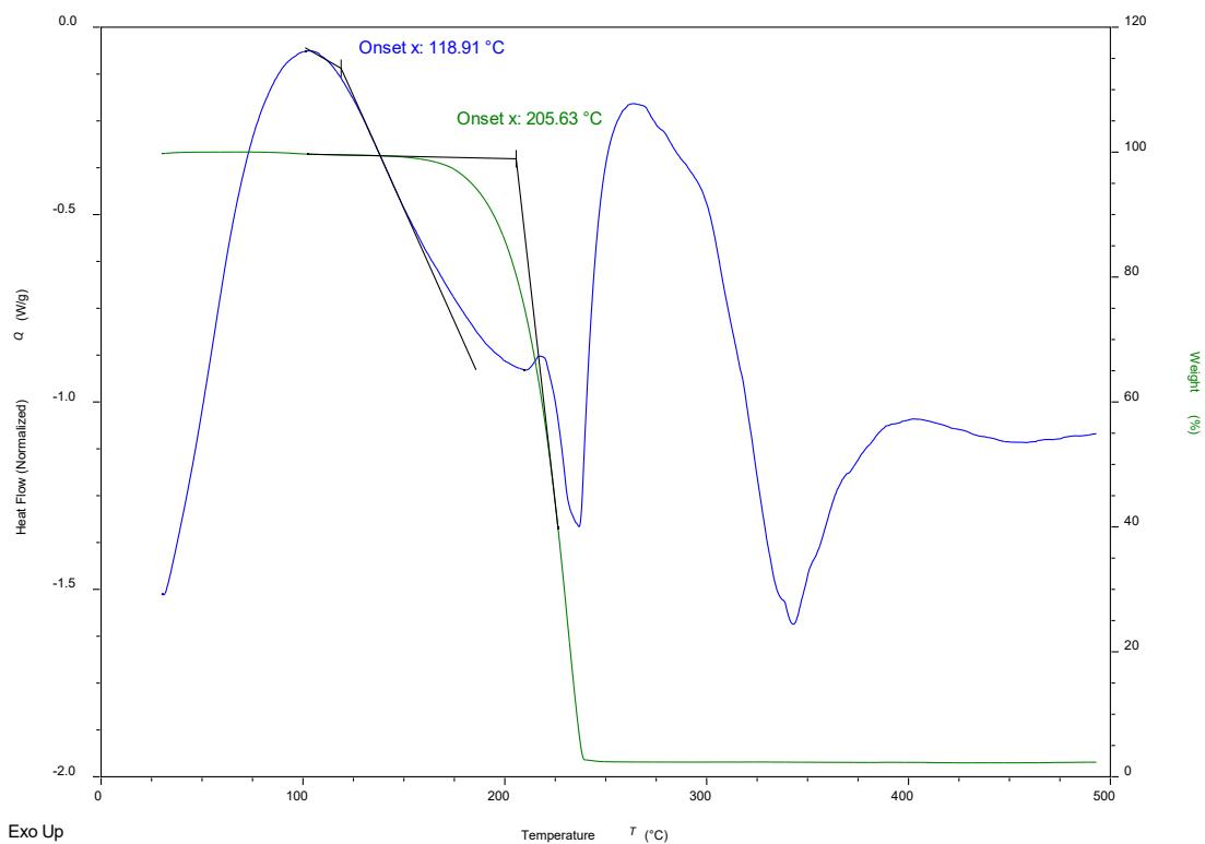
**Figure SI22.** SDT of  $(\text{I}_2\text{F}_8\text{bph})(4,4'\text{-bipy})$
