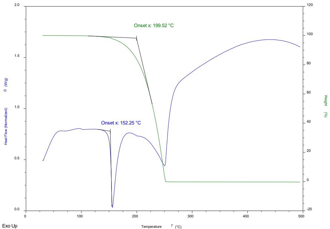
**Figure SI4.** SDT of  $(\text{I}_2\text{F}_8\text{bph})(\text{Me}_2\text{pyrz})$
