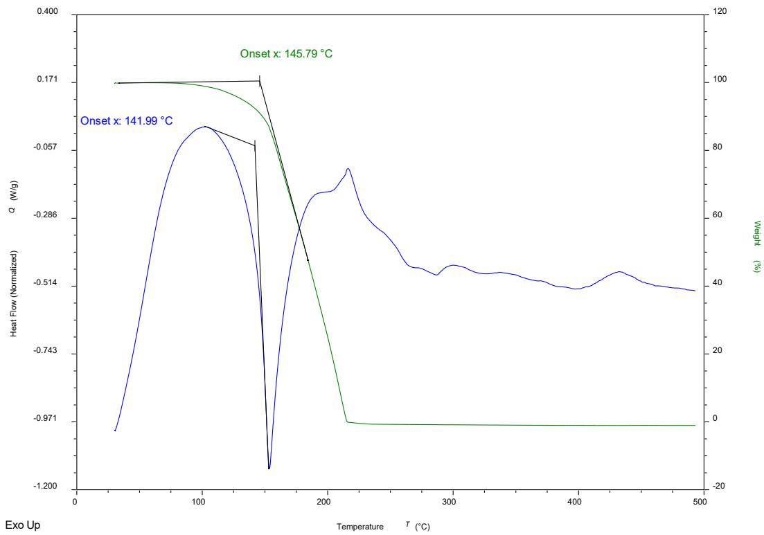
**Figure SI11.** SDT of  $(I_2F_8bph)(\text{quinox})$
