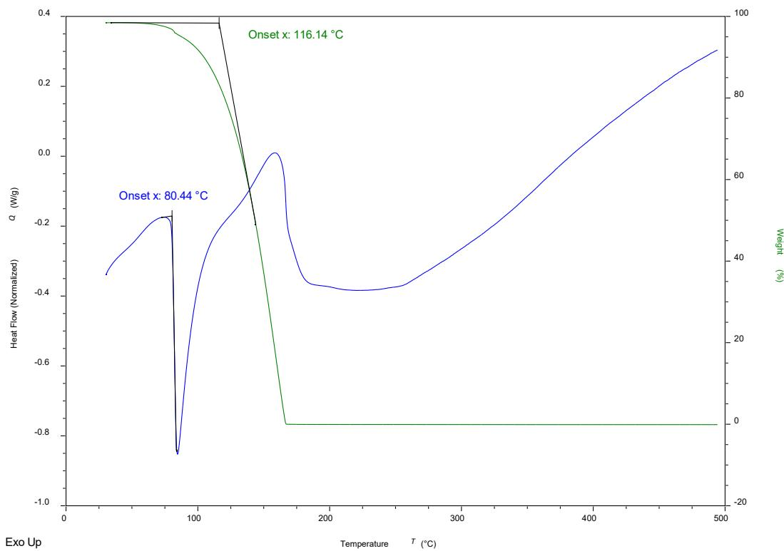
**Figure SI9.** SDT of  $(\text{Br}_2\text{F}_4\text{bz})(\text{quinox})$
