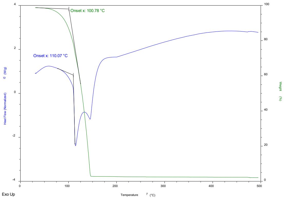
**Figure SI3.** SDT of  $(\text{Br}_2\text{F}_8\text{bph})(\text{Me}_2\text{pyrz})$
