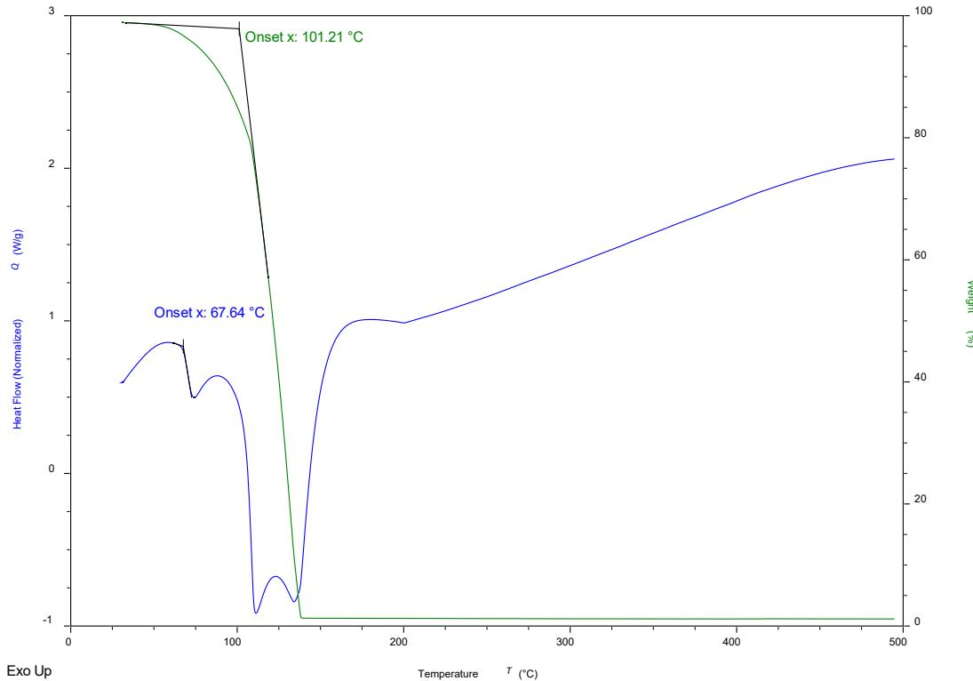
**Figure SI6.** SDT of  $(\text{Br}_2\text{F}_4\text{bz})(\text{Me}_4\text{pyrz})_2$
