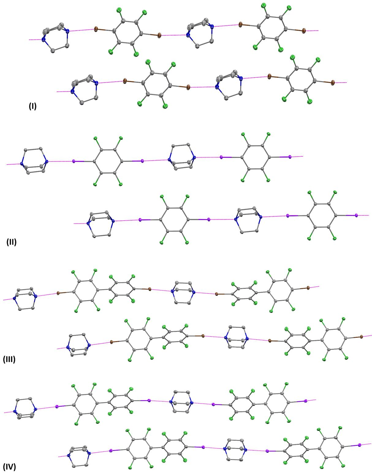
**Figure SI36.** Neighboring 1-d halogen bonding chains in  $(\text{Br}_2\text{F}_4\text{bz})(\text{DABCO})$  (I),  $(\text{I}_2\text{F}_4\text{bz})(\text{DABCO})$  (II),  $(\text{Br}_2\text{F}_8\text{bph})(\text{DABCO})$  (III), and  $(\text{I}_2\text{F}_8\text{bph})(\text{DABCO})$  (IV). Halogen bonds are shown as magenta dashed lines.
