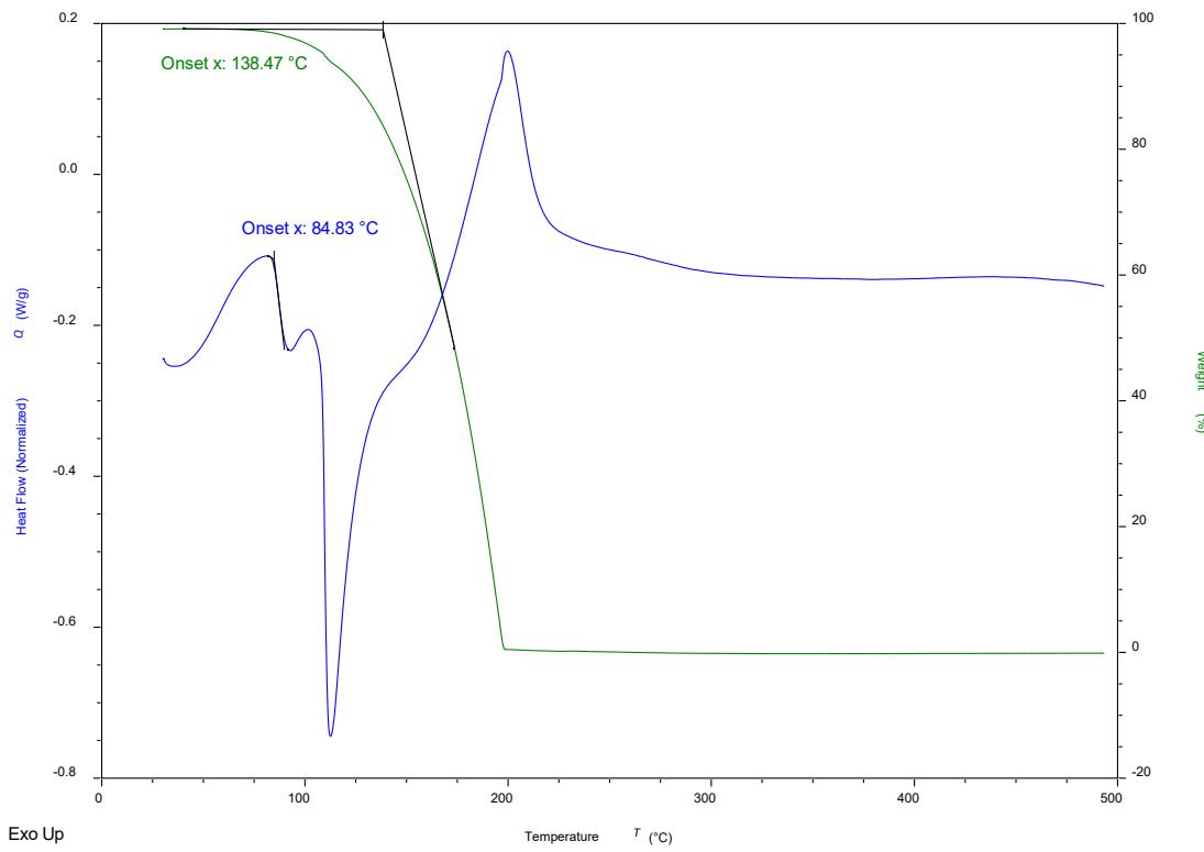
**Figure SI5.** SDT of  $(\text{I}_2\text{F}_4\text{bz})(\text{Me}_3\text{pyrz})$
