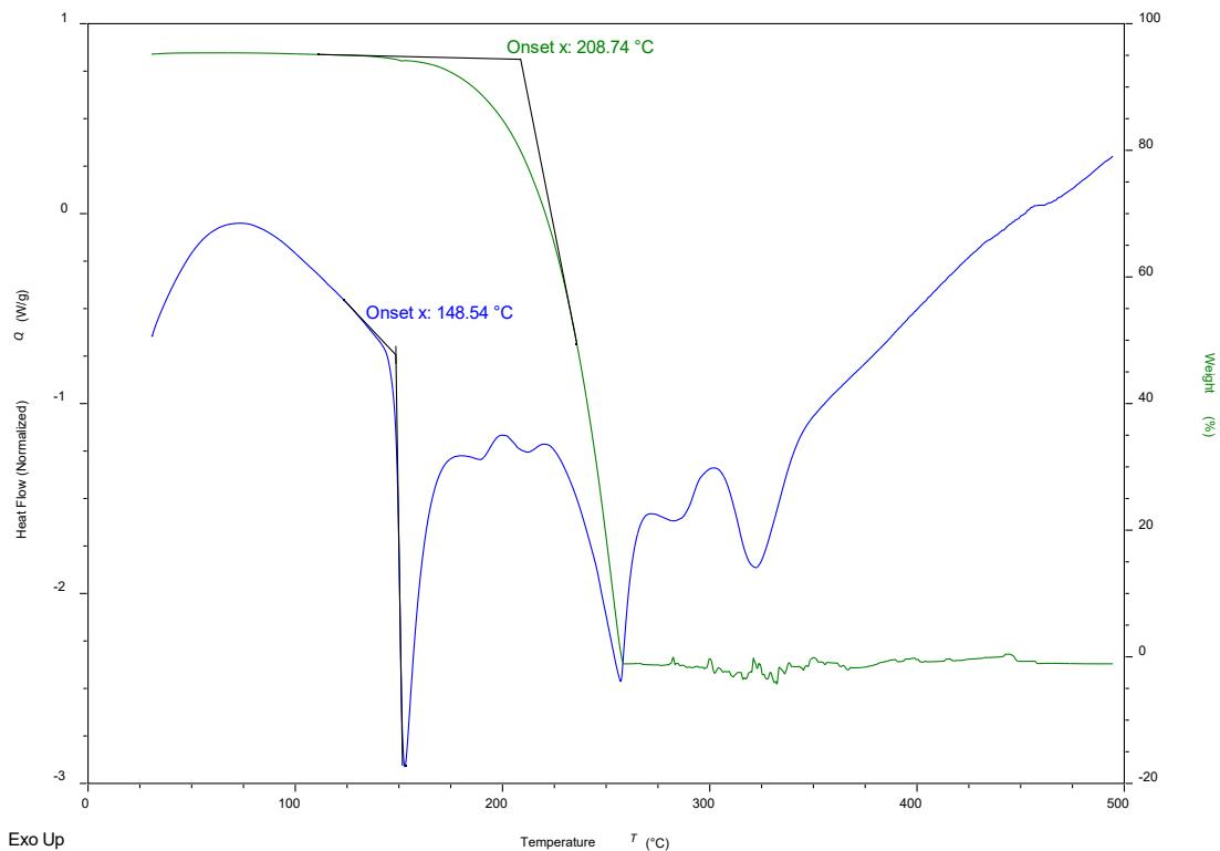
**Figure SI16.** SDT of  $(\text{I}_2\text{F}_8\text{bph})(2,2'\text{-bipy})$
