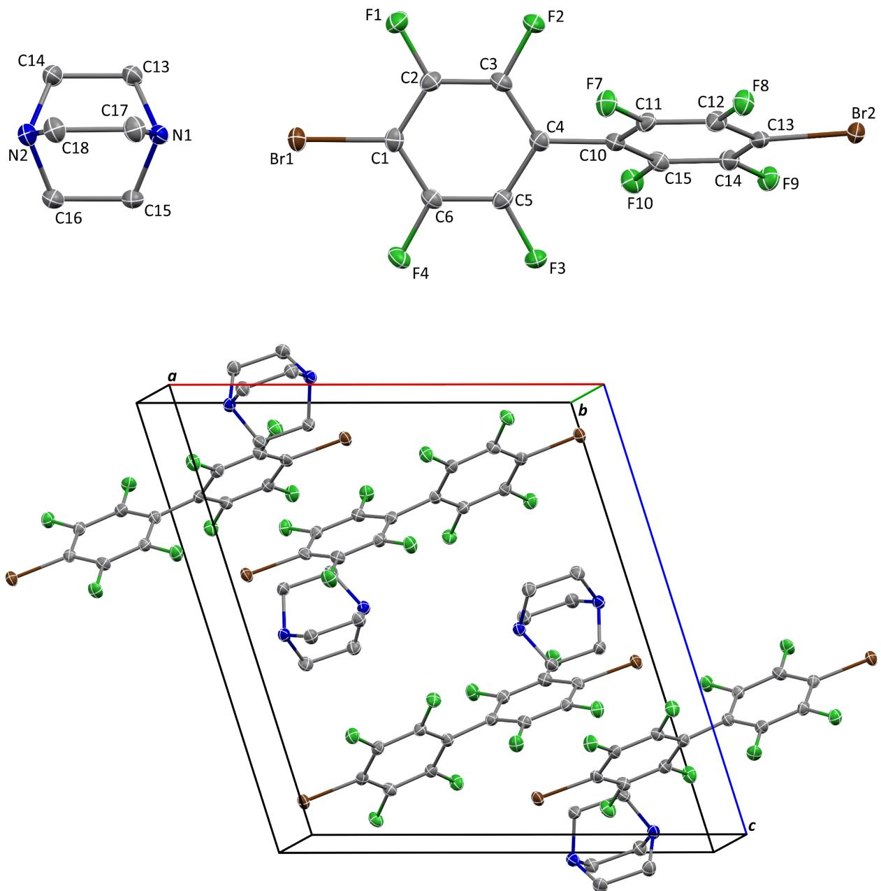
**Figure SI61.** Solid-state structure (top) and unit cell packing (bottom) of  $(\text{Br}_2\text{F}_8\text{bph})(\text{DABCO})$ . Atomic displacement ellipsoids are shown at the 50% probability level. Hydrogen atoms have been omitted for clarity.
