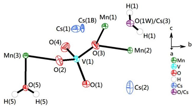
Figure S7. *Ortep* drawing (50% ellipsoid probability) of the asymmetric unit of 3.
