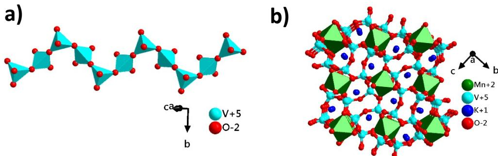
Figure S5. a) The  $(\text{VO}_3)_n$  chain in **1**. b) The 3D structure of **1** viewed along the  $a$ -axis.
