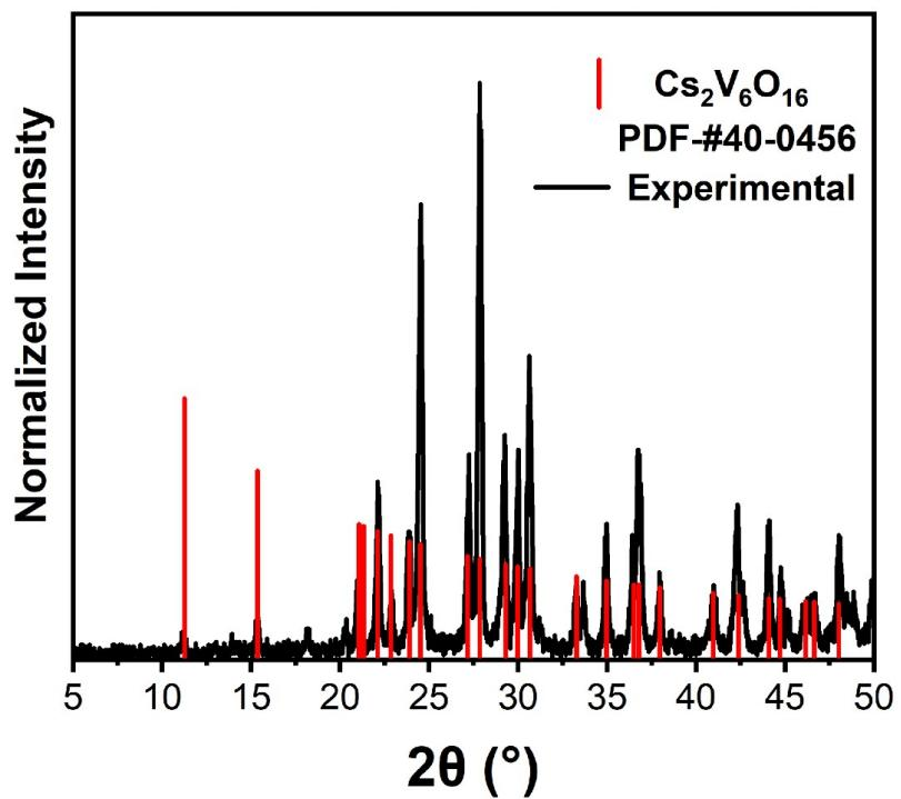
Figure S4. PXRD pattern of the brown powder compared with that from the standard PDF card of  $\text{Cs}_2\text{V}_6\text{O}_{16}$ .
