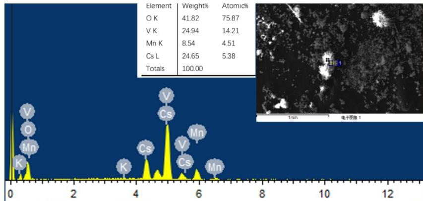
Figure S3. EDS spectrum for the unknown phase obtained in the  $\text{Cs}^+$  solutions with varied concentrations of 2500-4000 ppm, displaying elemental composition in weight and atomic percentage. Inset is the EDS image; the magnification is 1 mm, and the area of material is only one point on the face.
