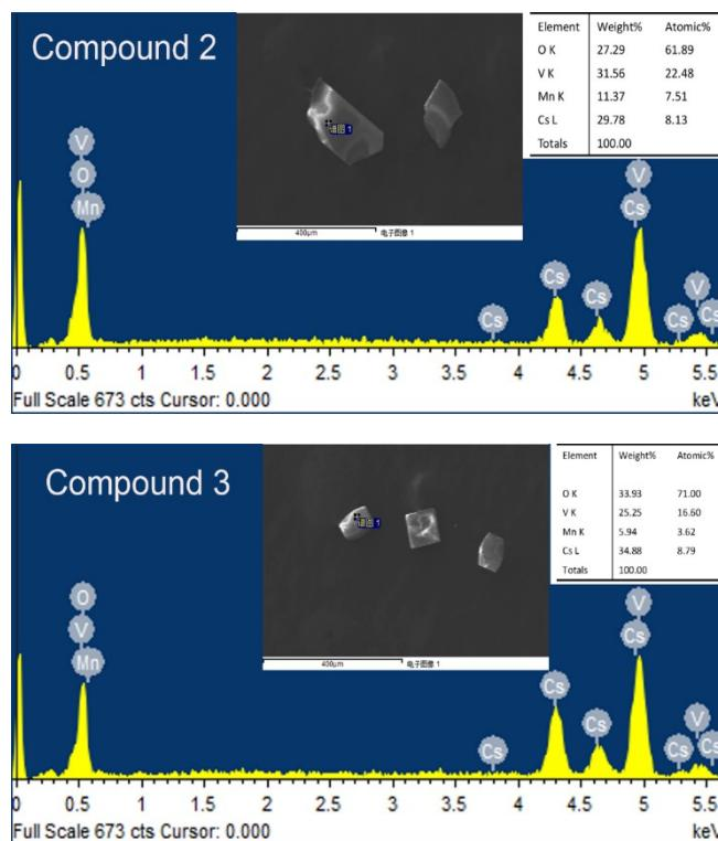
Figure S1. EDS spectra for 2 and 3 displaying the elemental compositions in both weight percentage and atomic percentage. Inset is the EDS image; the magnification is 400  $\mu\text{m}$ , and the area of material is only one point on the face.
