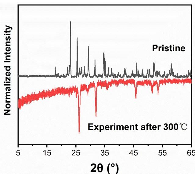
Figure S13. The original PXRD pattern of **3** compared with that of sample after heating to 300 °C.
