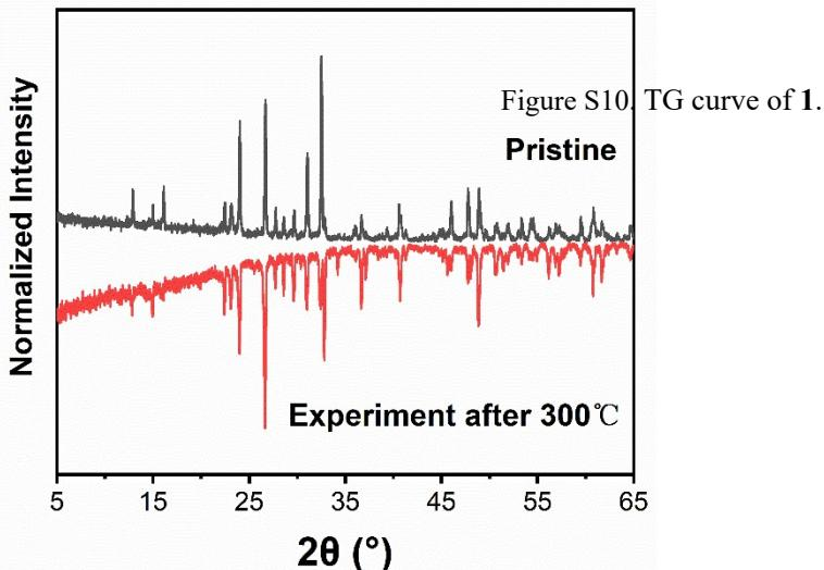
Figure S11. The original PXRD pattern of **1** compared with that of sample after heating to 300 °C.
