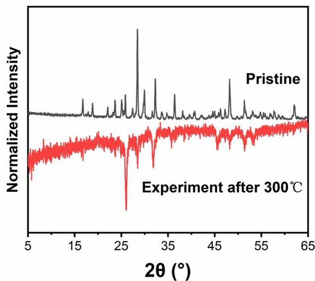
Figure S12. The original PXRD pattern of **2** compared with that of sample after heating to 300 °C.
