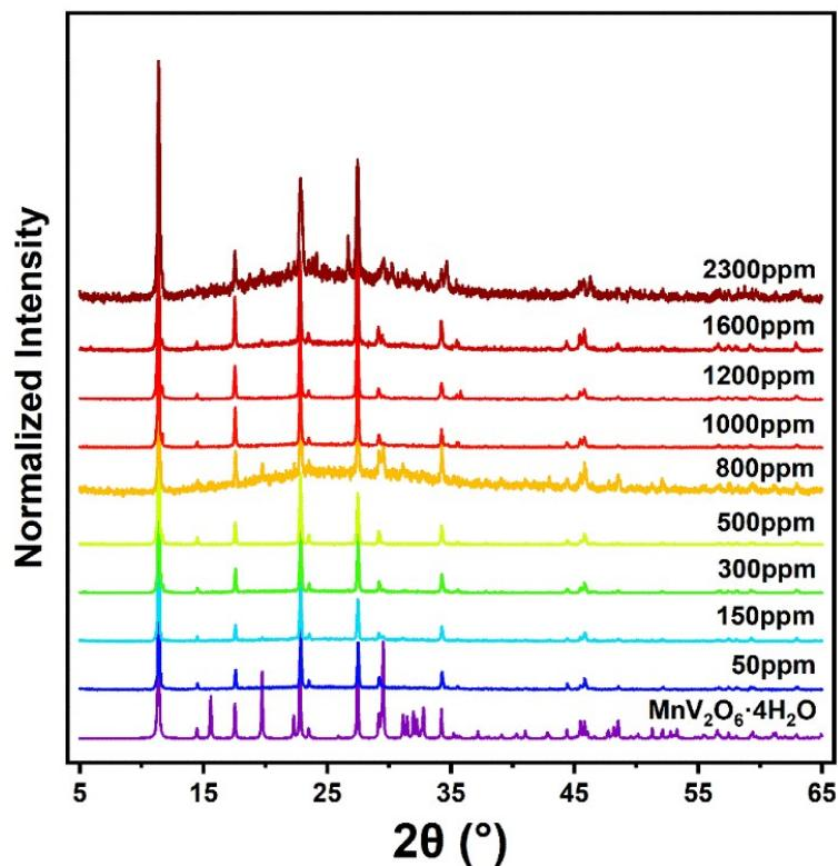
Figure S2. Comparison of the simulated PXRD pattern of  $\text{MnV}_2\text{O}_6 \cdot 4\text{H}_2\text{O}$  with the experimental ones for the samples generated by immersing **1** in the  $\text{Cs}^+$  solutions with varied concentrations of 50-2300 ppm.
