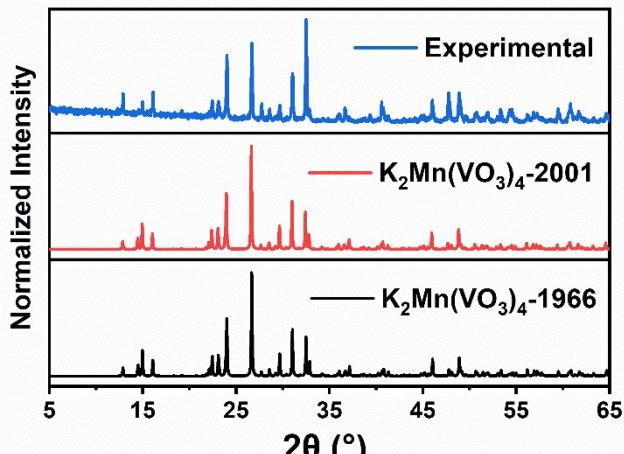
Figure S9. Simulated and experimental PXRD patterns for  $\text{K}_2\text{Mn}(\text{VO}_3)_4$ .
