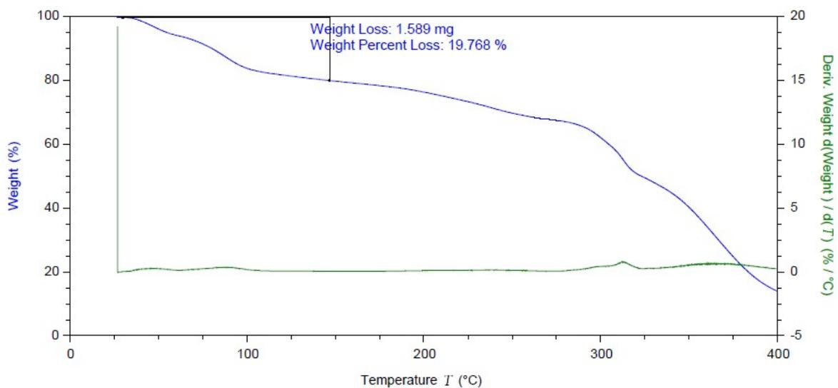
Figure S6: TGA traces of Cu-MOF.
