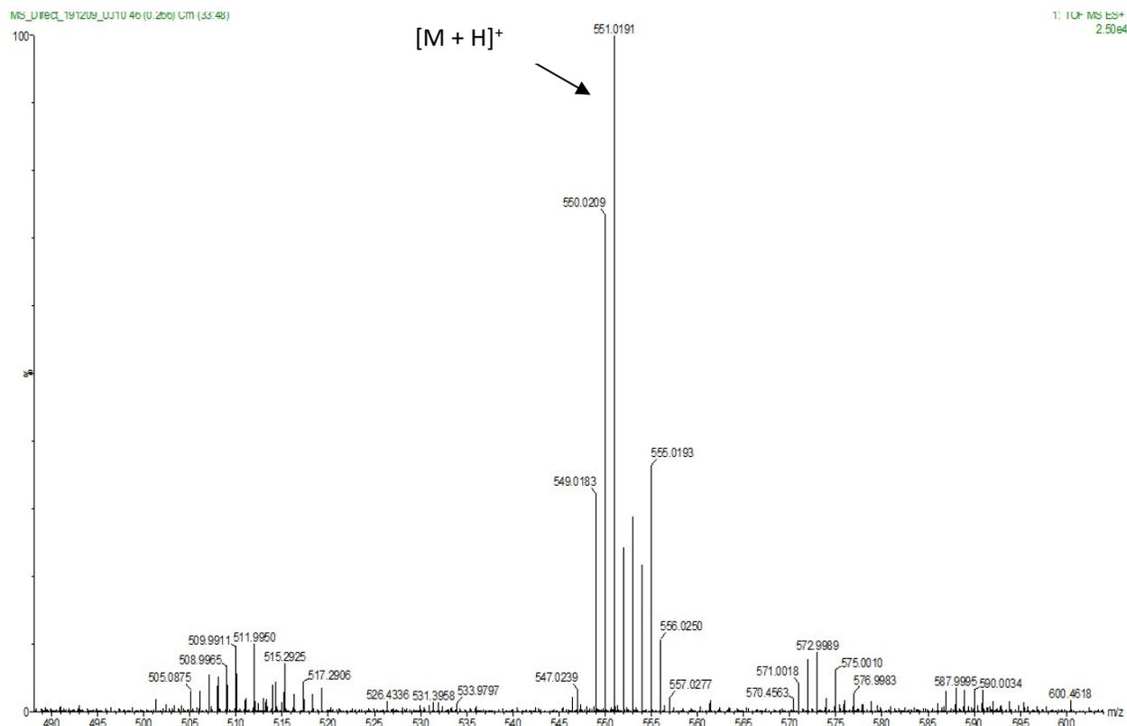
**Figure S3:** Mass spectrum of **C1** showing a base peak fragment of a monomeric palladium(II) species.
