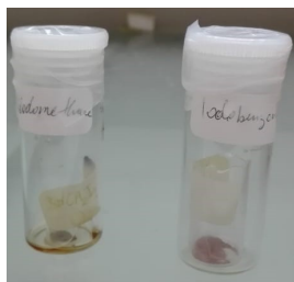
Figure S1: Sorption of VOCs (large vials) into the MOF adsorbents 1d or 2d in narrow vials. The examples shown here are 1d and iodomethane (left) and 1d and iodobenzene (right)
