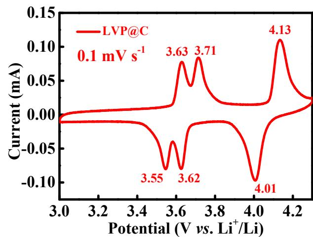
**Fig. S7** CV curves of LVP@C at a scan rate of  $0.1 \text{ mV s}^{-1}$
