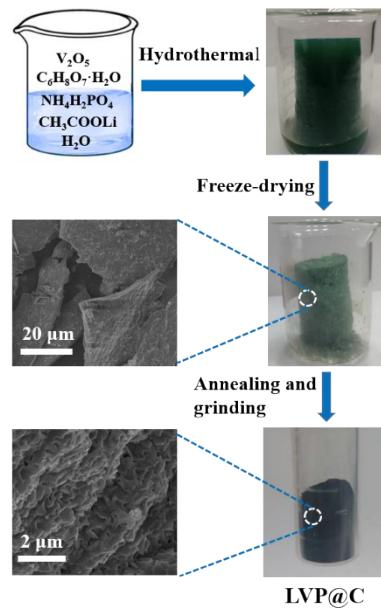
**Fig. S1** Digital photographs and FESEM images of hydrothermal synthesis materials and LVP@C.
