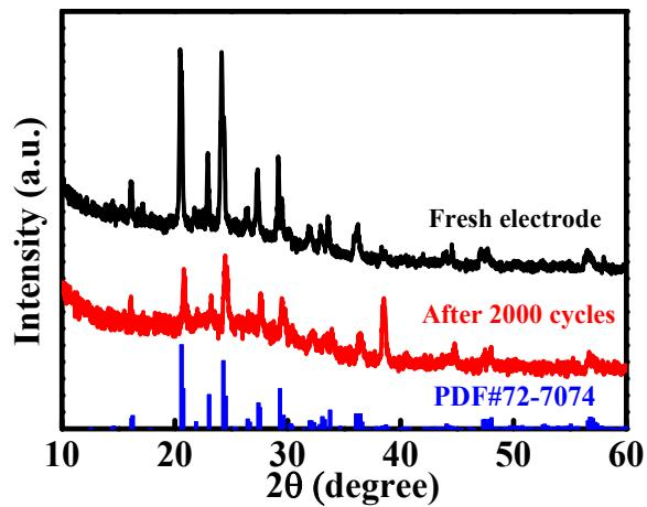
**Fig. S8** XRD patterns of LVP@C electrode (fresh and after 2000 cycles).
