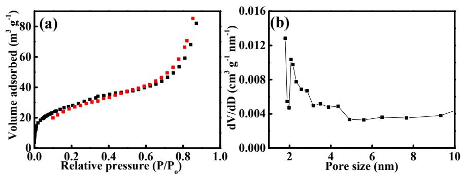
**Fig. S4** N<sub>2</sub> adsorption-desorption isotherm (a) and pore size distribution (b) of LVP@C according to the NLDFT model.
