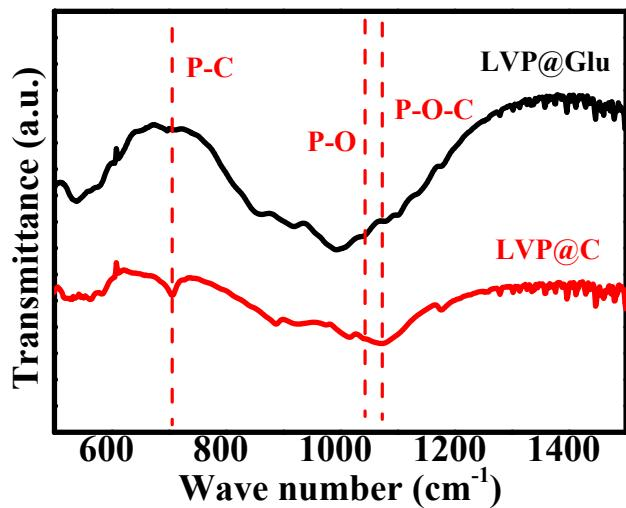
**Fig. S6** The FTIR spectra curves of LVP@C and LVP@Glu.
