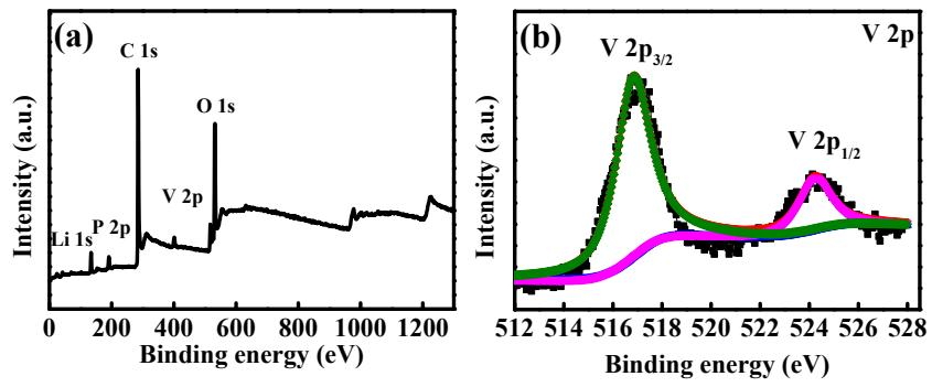
**Fig. S5** (a) XPS curve of survey spectrum of LVP@C; (b) The high-resolution spectrum of V 2p.
