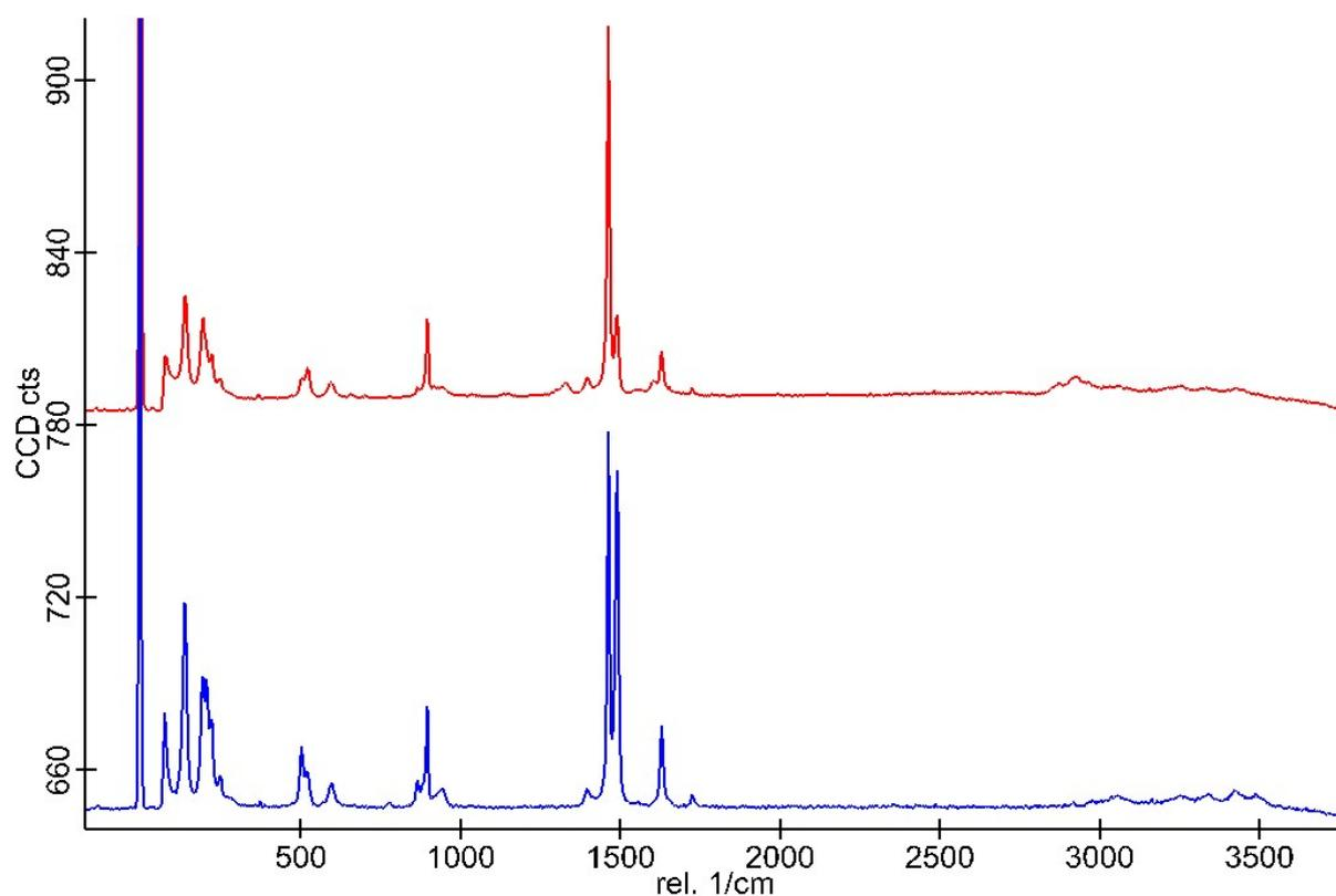
Figure S4. Raman spectrum collected with 532 nm laser. PCLys (red) vs COM pure (blue) showing the signals from COM on the crystals formed in the presence of PCLys
