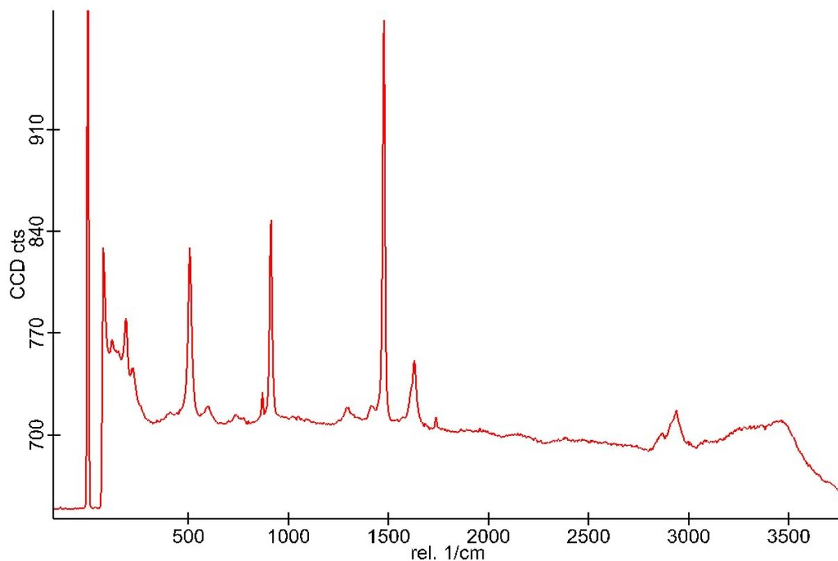
Figure S3. Recorded signal for the PRAsP crystals formed showing singlet at 1500  $1/\text{cm}$  representing COD
