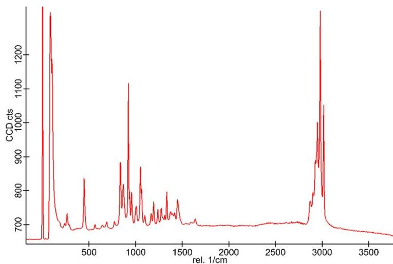
Figure S8. Raman spectrum of DL-Pro amino acid showing strong signals in the 2800-3000  $1/cm$  region
