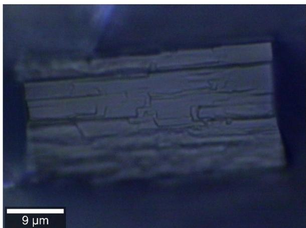
*Figure S9. Optical image of the COD crystal formed in the presence of PRAsp scanned in depth analysis*
