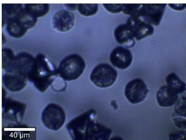
*Figure S11. Optical image of the COM crystals formed in the presence of CPro scanned in depth analysis*
