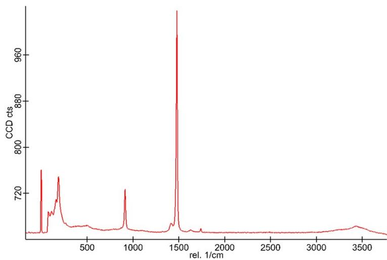
Figure S5. Raman spectrum of pure COD in SUM obtained from crystallisation at approximately 4°C for 24 hours
