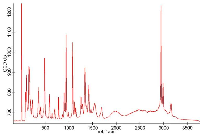
Figure S6. Raman spectrum of DL-Asp amino acid showing strong signals in the 2800-3000 1/cm region
