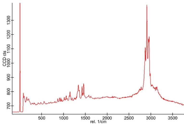
Figure S7. Raman spectrum of DL-Lys-HCl amino acid showing strong signals in the 2800-3000  $1/cm$  region
