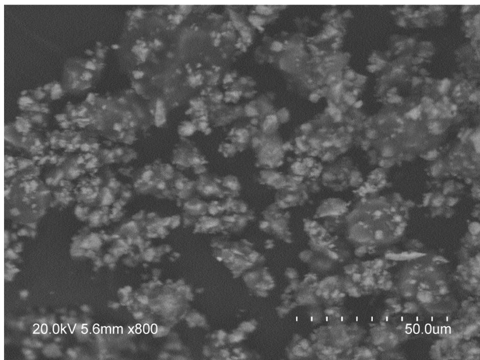
**Figure S31:** Secondary and backscattered images of solid  $m_{15}\text{-UO}_3\text{-Na}_2\text{O}_2$
