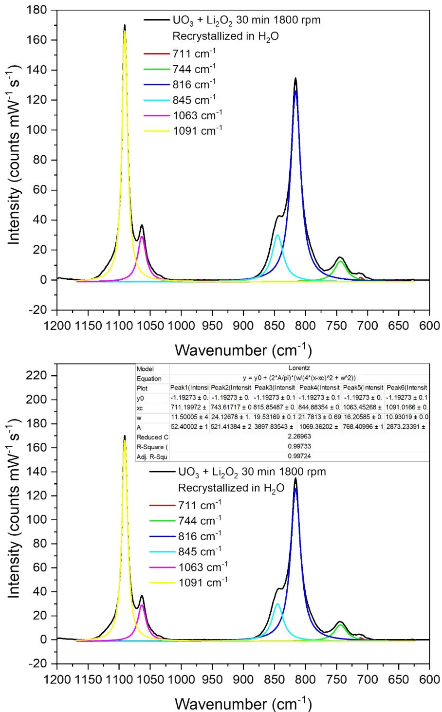
**Figure S13:** Raman fitting parameters of recrystallized  $m_{30}$ -UO<sub>3</sub>-Li<sub>2</sub>O<sub>2</sub>
