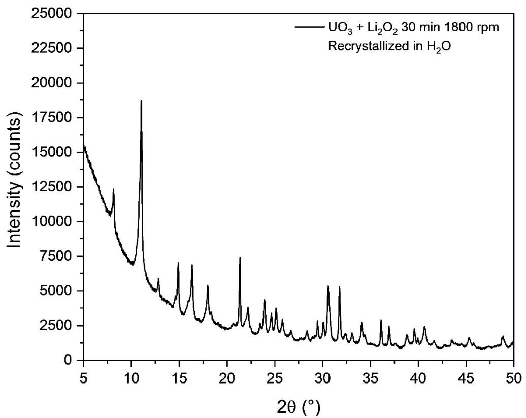
**Figure S2:** Raw PXRD pattern of recrystallized  $m_{30}\text{-UO}_3\text{-Li}_2\text{O}_2$
