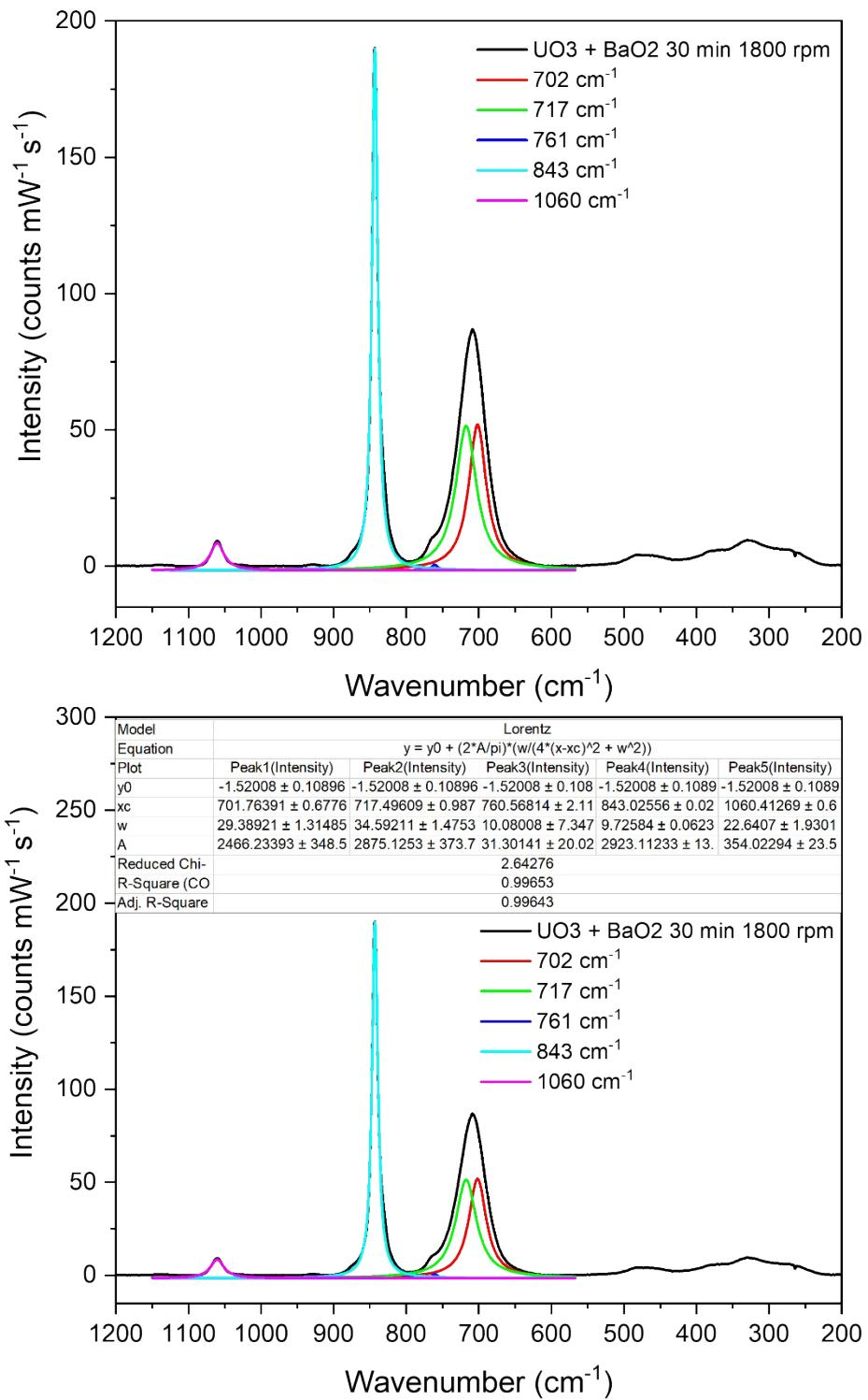
**Figure S21:** Raman fitting parameters of solid UO<sub>3</sub> + BaO<sub>2</sub> 30 min 1800 rpm
