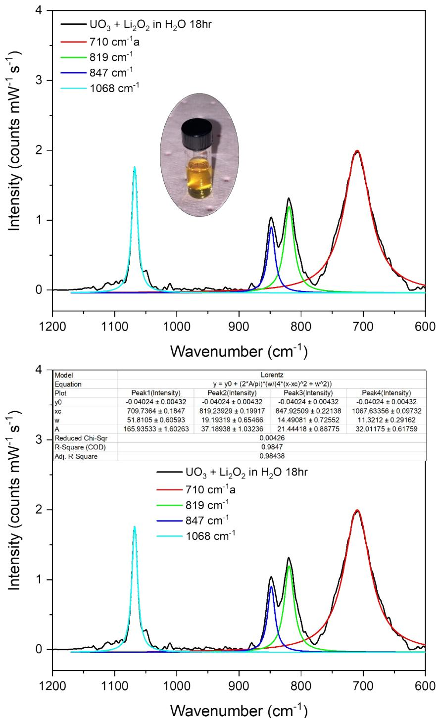
**Figure S12:** Raman fitting parameters of dissolved  $m_{30}\text{-UO}_3\text{-Li}_2\text{O}_2$  in  $\text{H}_2\text{O}$  18 hr
