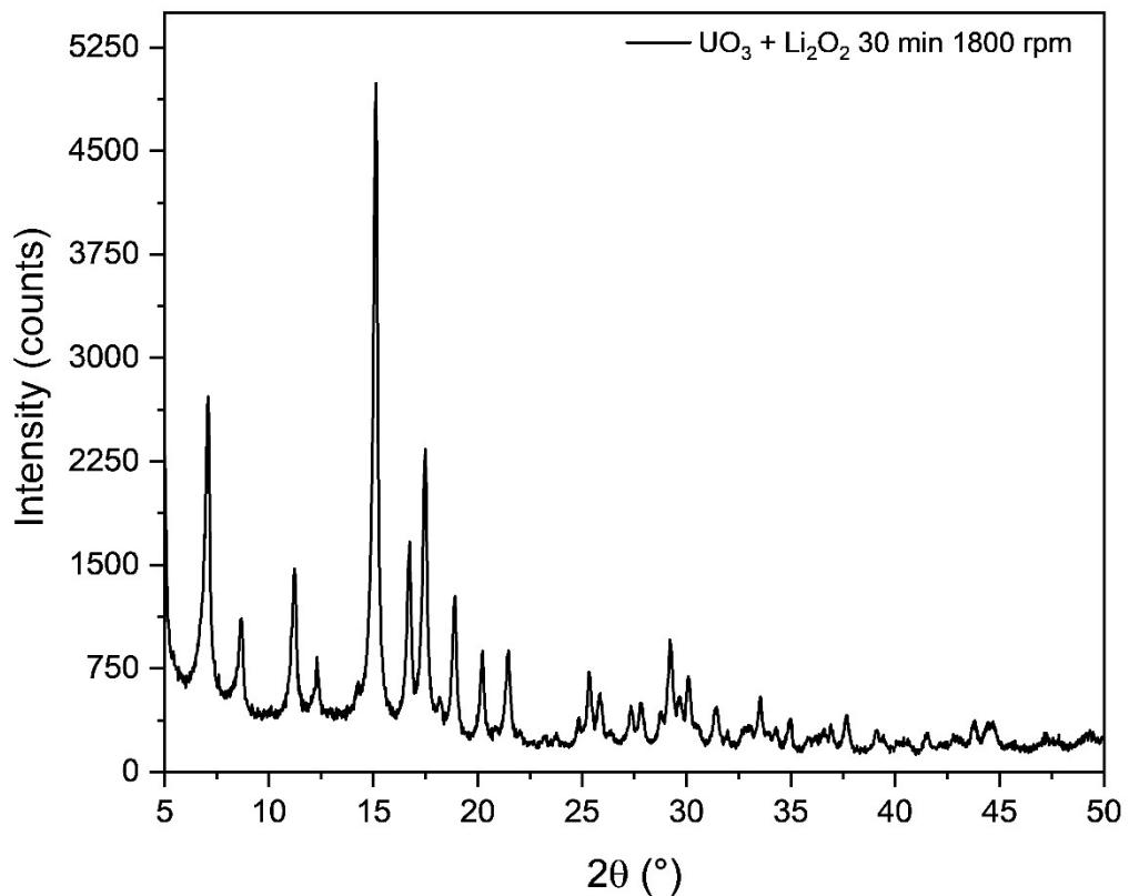
**Figure S1:** Raw PXRD pattern of  $m_{30}$ -UO<sub>3</sub>-Li<sub>2</sub>O<sub>2</sub>
