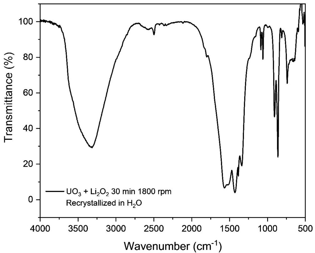
**Figure S23:** Infrared spectrum of recrystallized  $m_{30}$ -UO<sub>3</sub>-Li<sub>2</sub>O<sub>2</sub>
