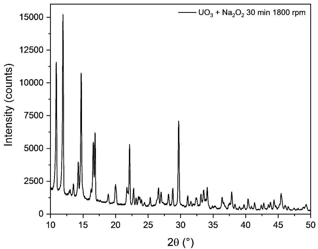
**Figure S5:** Raw PXRD pattern of  $m_{30}\text{-UO}_3\text{-Na}_2\text{O}_2$  enhanced  $2\theta$   $10^{\circ}\text{-}50^{\circ}$
