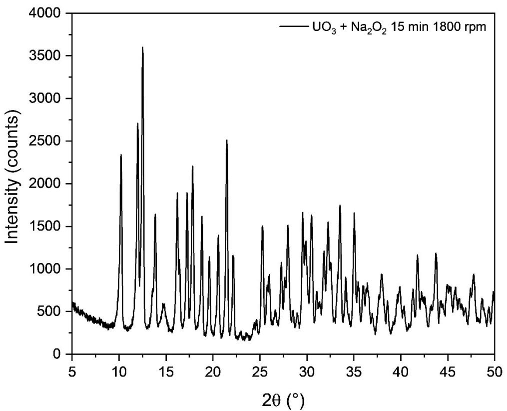
**Figure S3:** Raw PXRD pattern of  $m_{15}\text{-UO}_3\text{-Na}_2\text{O}_2$
