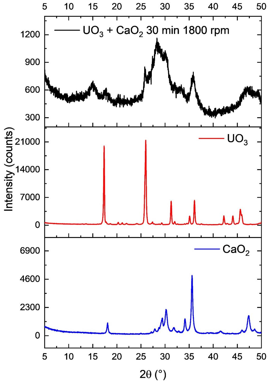
**Figure S8:** Raw PXRD patterns of  $\text{UO}_3 + \text{CaO}_2$  30 min 1800 rpm and starting materials
