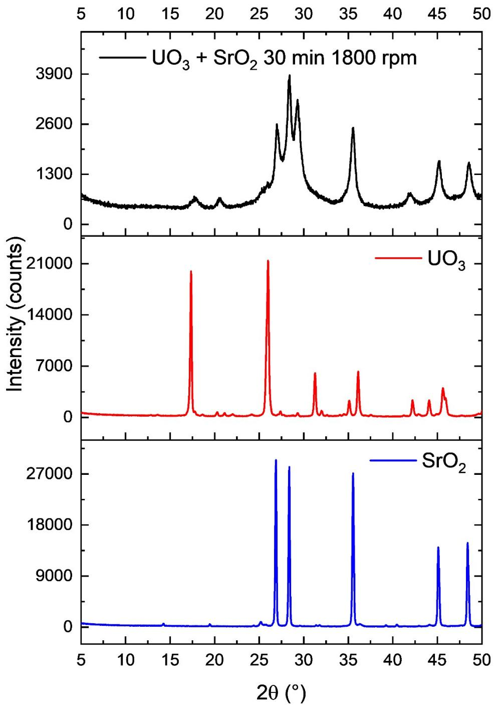
**Figure S9:** Raw PXRD patterns of  $\text{UO}_3 + \text{SrO}_2$  30 min 1800 rpm and starting materials
