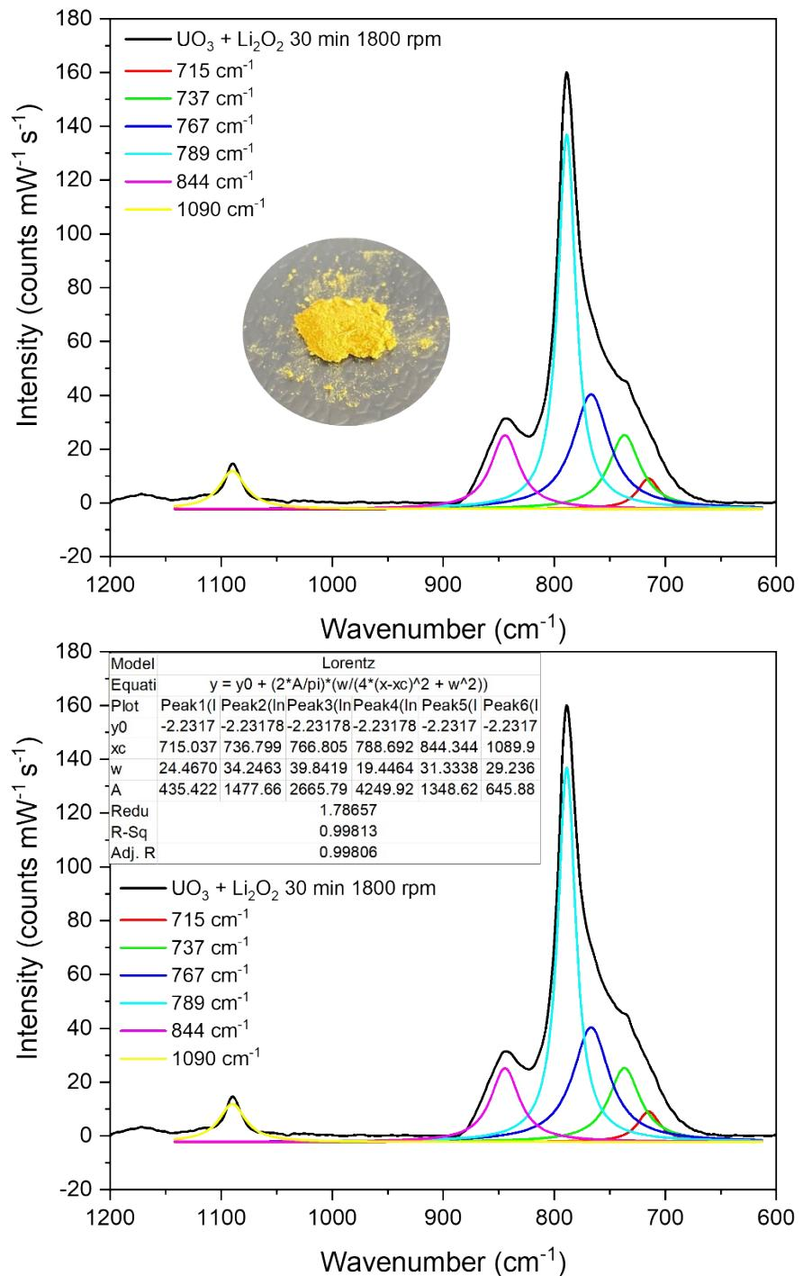
**Figure S11:** Raman fitting parameters of solid  $m_{30}\text{-UO}_3\text{-Li}_2\text{O}_2$
