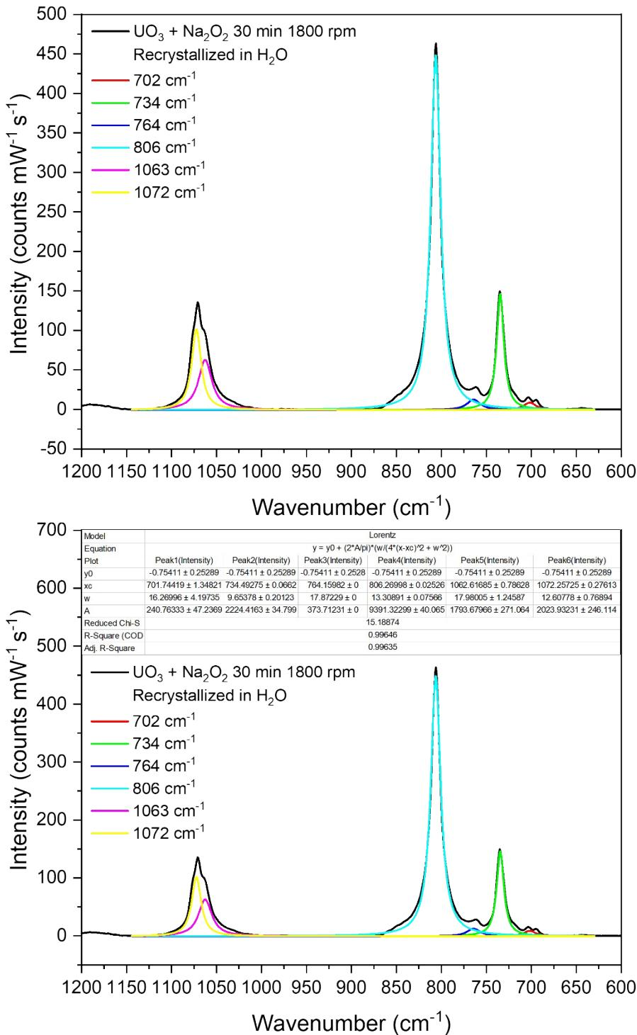
**Figure S17:** Raman fitting parameters of recrystallized  $m_{30}\text{-UO}_3\text{-Na}_2\text{O}_2$
