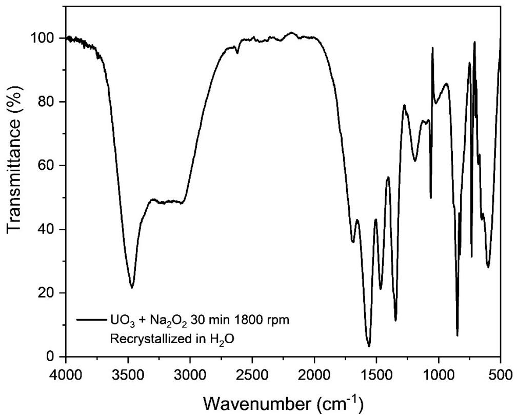
**Figure S26:** Infrared spectrum of recrystallized  $m_{30}$ - $\text{UO}_3\text{-Na}_2\text{O}_2$
