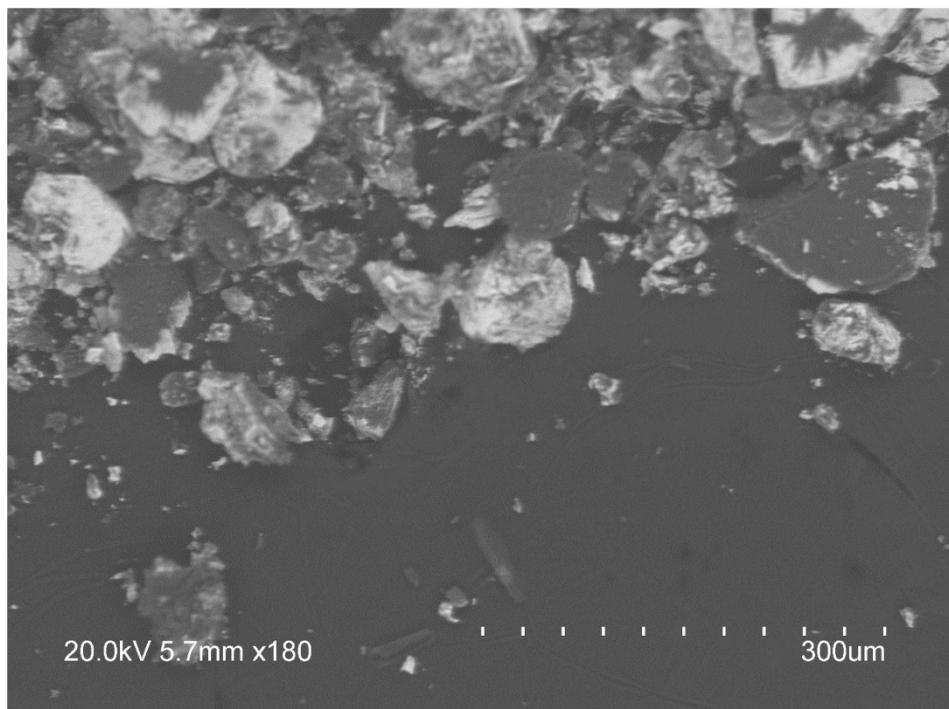
**Figure S30:** Secondary and backscattered images of recrystallized  $m_{30}\text{-UO}_3\text{-Li}_2\text{O}_2$
