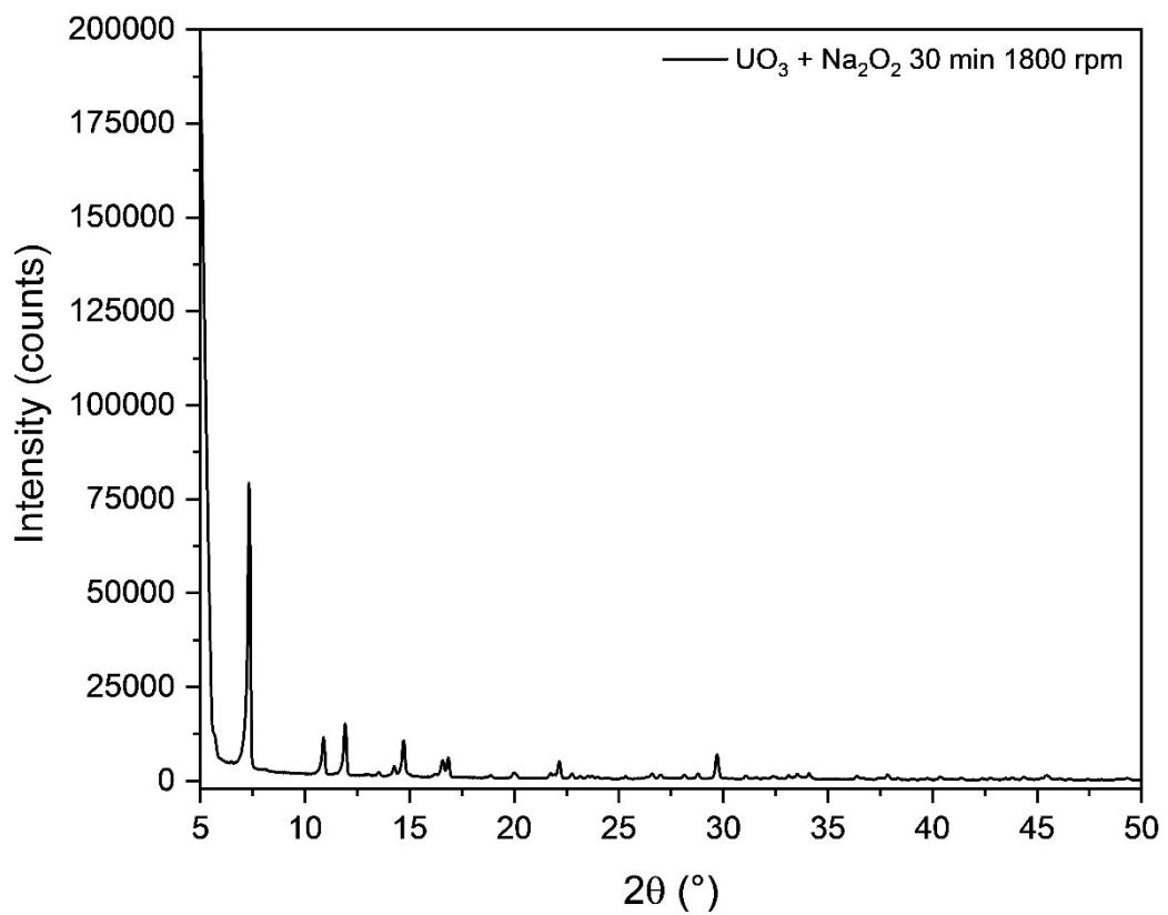
**Figure S4:** Raw PXRD pattern of  $m_{30}\text{-UO}_3\text{-Na}_2\text{O}_2$
