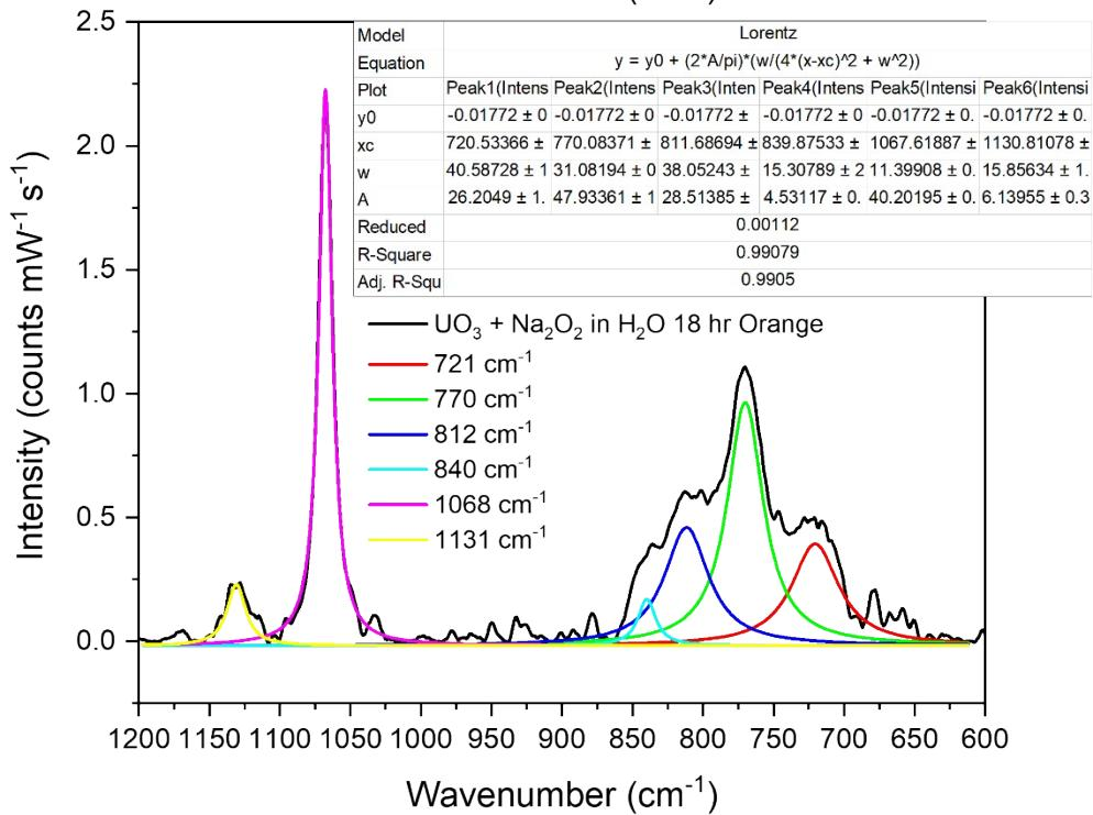
**Figure S16:** Raman fitting parameters of dissolved  $m_{30}\text{-UO}_3\text{-Na}_2\text{O}_2$  in  $\text{H}_2\text{O}$  18 hr
