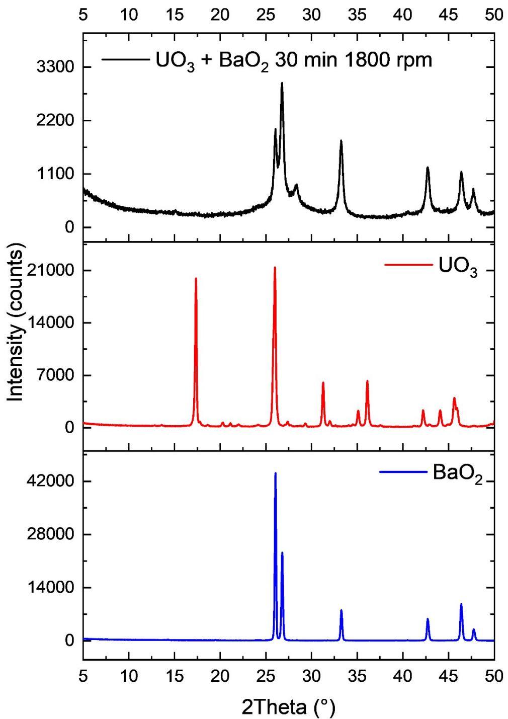
**Figure S10:** Raw PXRD patterns of  $\text{UO}_3 + \text{BaO}_2$  30 min 1800 rpm and starting materials
