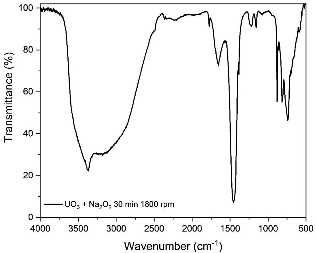
**Figure S25:** Infrared spectrum of solid  $m_{30}$ -UO<sub>3</sub>-Na<sub>2</sub>O<sub>2</sub>
