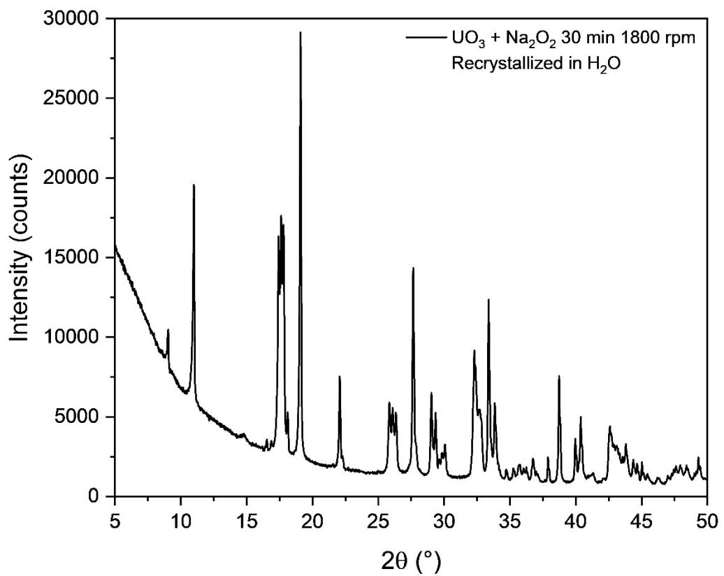
**Figure S6:** Raw PXRD pattern of recrystallized  $m_{30}\text{-UO}_3\text{-Na}_2\text{O}_2$
