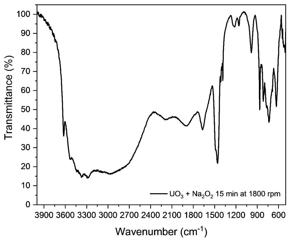
**Figure S24:** Infrared spectrum of solid  $m_{15}$ - $\text{UO}_3\text{-Na}_2\text{O}_2$
