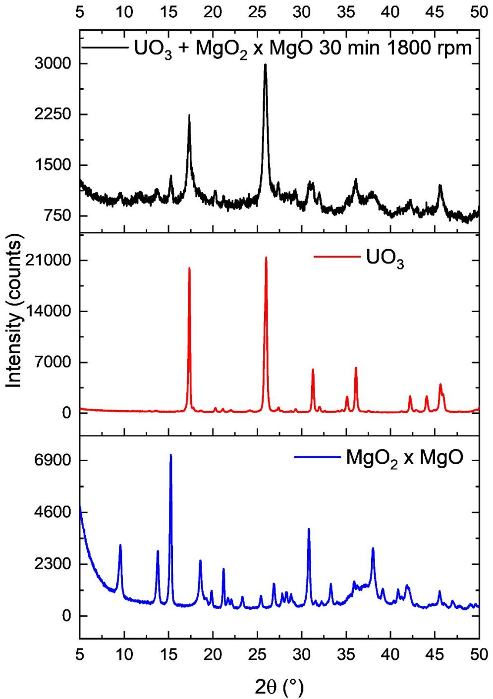
**Figure S7:** Raw PXRD patterns of  $\text{UO}_3 + \text{MgO}_2$  30 min 1800 rpm and starting materials
