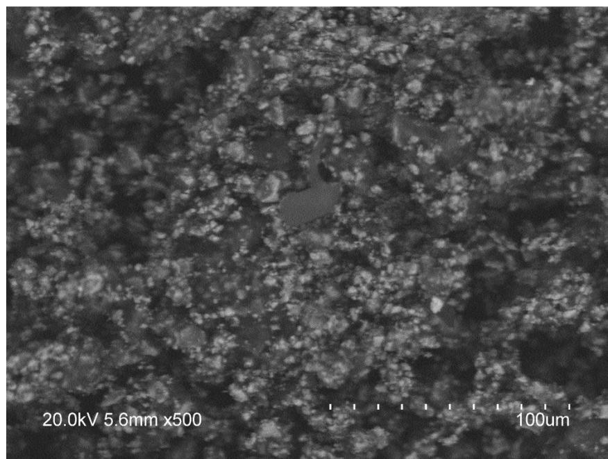
**Figure S29:** Secondary and backscattered images of recrystallized  $m_{30}$ - $\text{UO}_3$ - $\text{Li}_2\text{O}_2$
