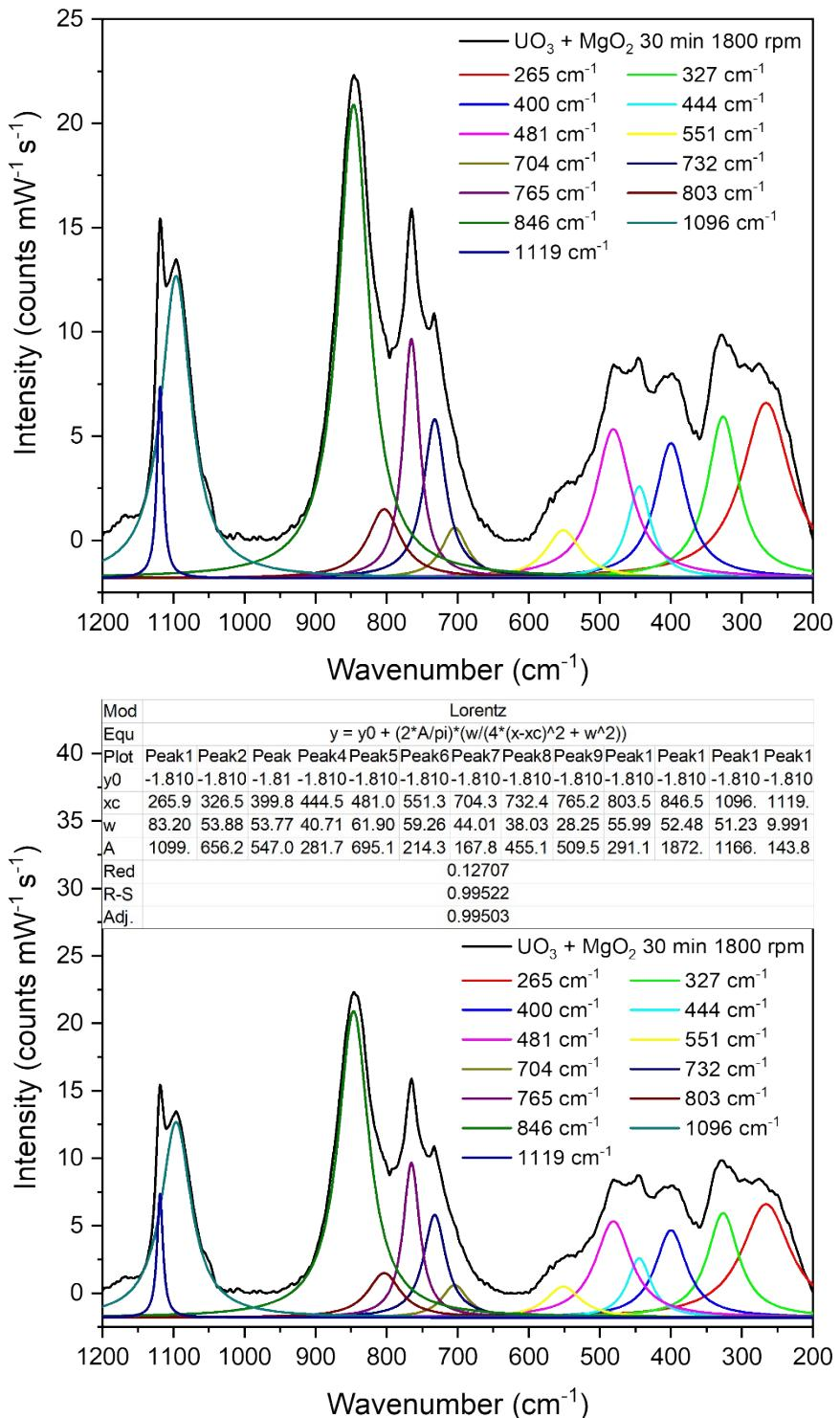
**Figure S18:** Raman fitting parameters of solid  $\text{UO}_3 + \text{MgO}_2$  30 min 1800 rpm
