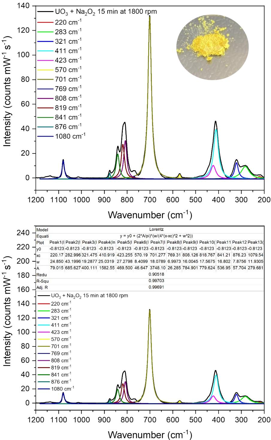
**Figure S14:** Raman fitting parameters of solid  $m_{15}$ -UO<sub>3</sub>-Na<sub>2</sub>O<sub>2</sub>
