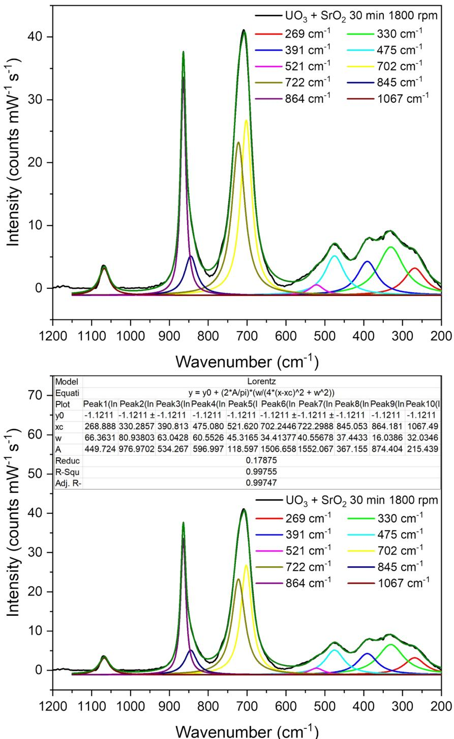
**Figure S20:** Raman fitting parameters of solid  $\text{UO}_3 + \text{SrO}_2$  30 min 1800 rpm
