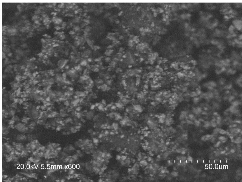
**Figure S28:** Secondary and backscattered images of solid  $m_{30}$ - $\text{UO}_3$ - $\text{Li}_2\text{O}_2$
