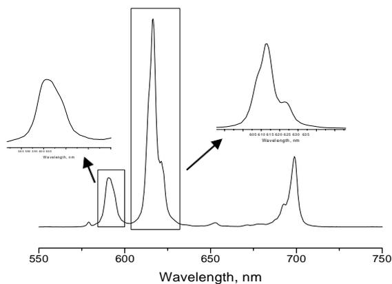
**Figure S2.** Study of the Stark splitting of the luminescence bands of the Eu(naph)<sub>3</sub> complex (powder, λ<sub>ex</sub> = 337 nm)
