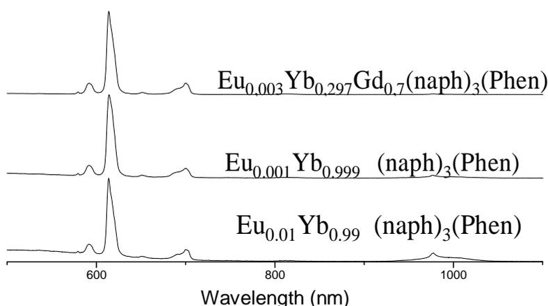
**Figure S6.** Luminescence spectra of  $Eu_xYb_yGd_{1-x-y}(naph)_3(Phen)$
