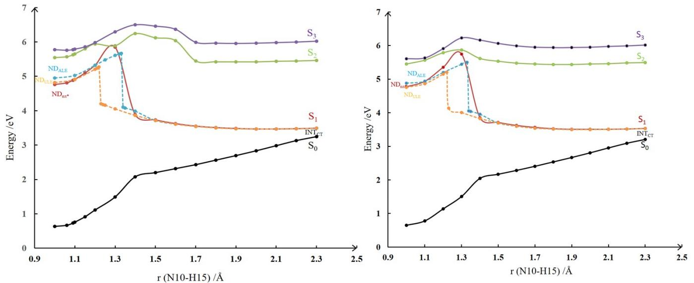
Figure S10 The potential energy profiles as a function of  $r(\text{N-H})$  along  $\text{N-H}\cdots\text{O}$  in the lowest 4 states calculated (a) at the (TD-)CAM-B3LYP/6-31G(d) level and (b) at the (TD-)CAM-B3LYP/TZVP level.
