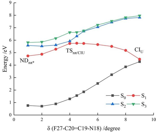
Figure S12 The potential energy profiles of the LIIC between  $ND_{n\pi^*}$  and  $CI_U$  at the (TD-)CAM-B3LYP/6-31G(d) level
