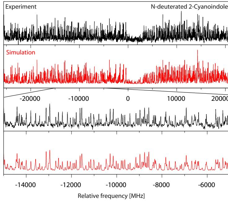
FIG. S1. Rotationally resolved electronic spectrum of the electronic origin of 2-cyanoindole(1-d<sub>1</sub>), along with a simulation with the best CMA-ES fit parameters.
