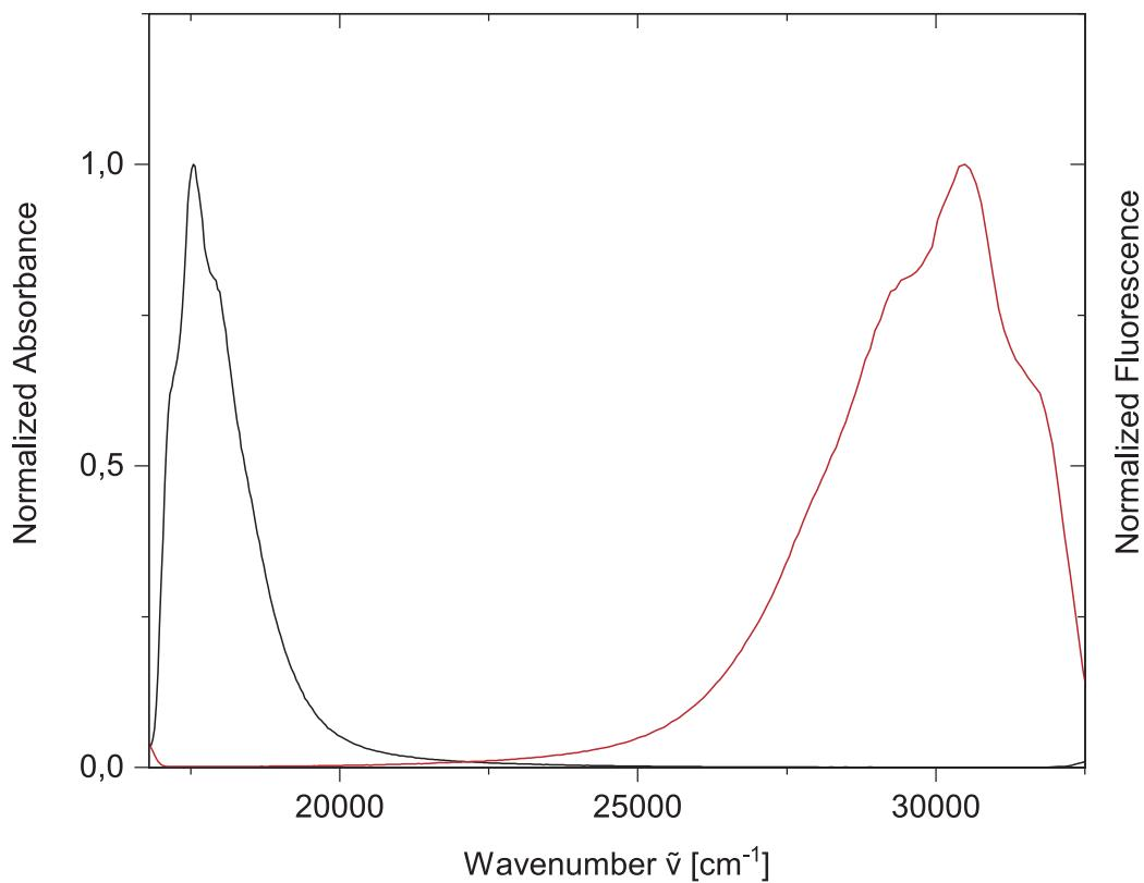
FIG. S4. Steady state absorption and fluorescence spectrum of 2-cyanoindole in ethylacetate.
