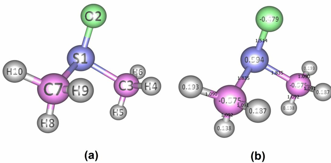
**Fig. S1.** The geometry of DMSO optimized by the DFT B3LYP/6-311++G(d,p) level of theory: (a) atoms with labels (b) atoms with charges and bond lengths.
