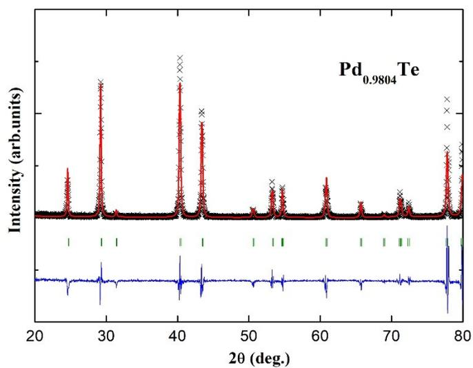
Fig S10. Le Bail refinement plot of Pd<sub>1-y</sub>Te ( $y = 1.96\%$ ).
