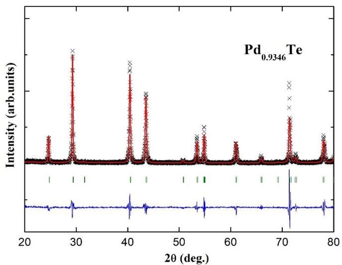
Fig S14. Le Bail refinement plot of  $\text{Pd}_{1-y}\text{Te}$  ( $y = 6.54\%$ ).
