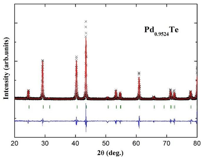
Fig S13. Le Bail refinement plot of  $\text{Pd}_{1-y}\text{Te}$  ( $y = 4.76\%$ ).
