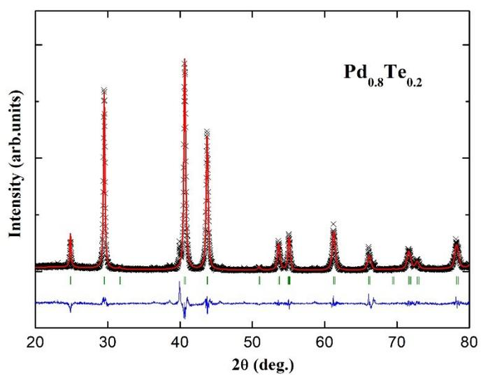
Fig S7. Le Bail refinement plot of  $\text{PdTe}_{1-x}\text{Sb}_x$  ( $x = 0.2$ ).
