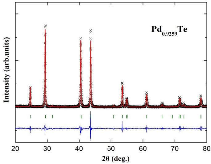
Fig S15. Le Bail refinement plot of  $\text{Pd}_{1-y}\text{Te}$  ( $y = 7.41\%$ ).
