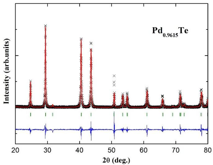
Fig S12. Le Bail refinement plot of  $\text{Pd}_{1-y}\text{Te}$  ( $y = 3.85\%$ ).
