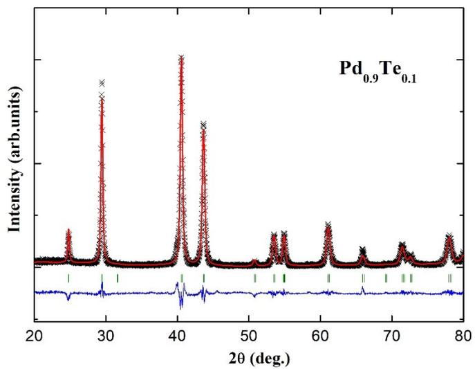
Fig S3. Le Bail refinement plot of  $\text{PdTe}_{1-x}\text{Sb}_x$  ( $x = 0.1$ ).
