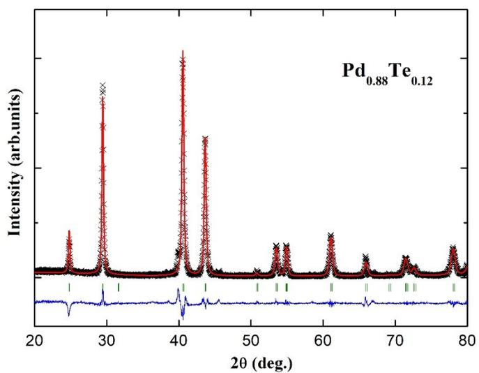
Fig S4. Le Bail refinement plot of  $\text{PdTe}_{1-x}\text{Sb}_x$  ( $x = 0.12$ ).
