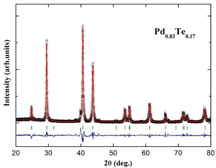
Fig S6. Le Bail refinement plot of  $\text{PdTe}_{1-x}\text{Sb}_x$  ( $x = 0.17$ )
