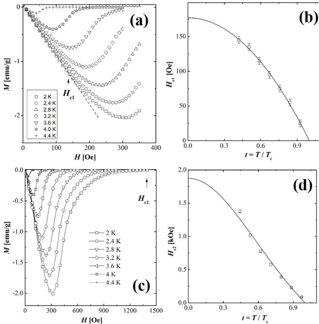
Fig S16. (a)  $M$ - $H$  plots of PdTe at various temperatures. (b)  $H_{c1}$  of PdTe against normalized  $t$  is depicted and fitted using the formula  $H_{c1}(T) = H_{c1}(0) * (1 - t^2)$ . (c)  $M$ - $H$  plots of PdTe in higher fields at fixed Ts. (d)  $H_{c2}$  of PdTe against  $t$  is depicted and
