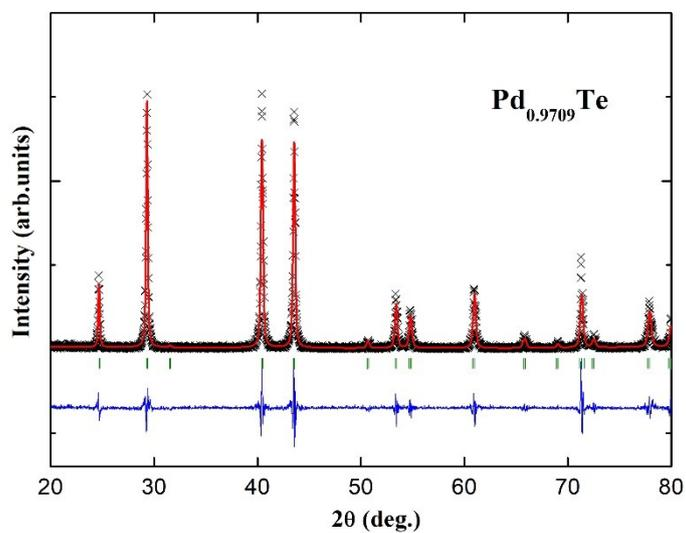
Fig S11. Le Bail refinement plot of Pd<sub>1-y</sub>Te ( $y = 2.91\%$ ).
