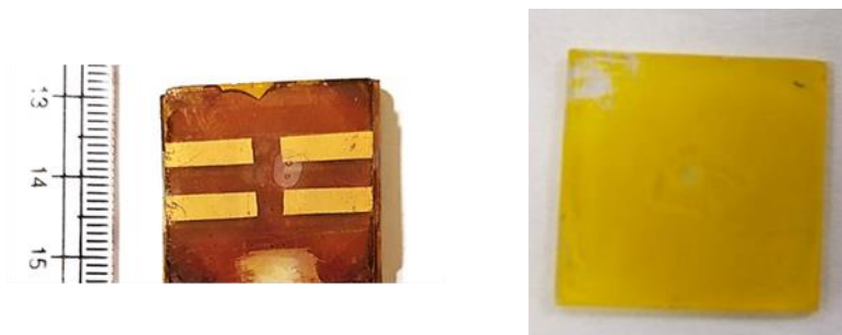
Figure S3: Photographs of the S-S and L-E devices. Electrochemical cell was fabricated by placing a PDMS stamp with a hole to hold the electrolyte during the measurement.
