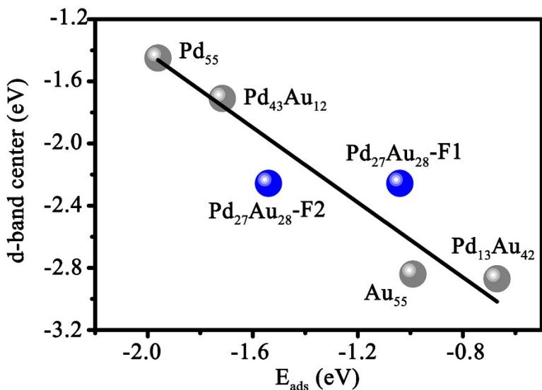
Figure S15 The relationship between the  $\text{SO}_2$  adsorption energies and the calculated  $d$ -band centers of the shell atoms for the  $\text{Pd}_{55}$ ,  $\text{Pd}_{43}\text{Au}_{12}$ ,  $\text{Pd}_{27}\text{Au}_{28}$ ,  $\text{Pd}_{13}\text{Au}_{42}$ , and  $\text{Au}_{55}$  nanoparticles.
