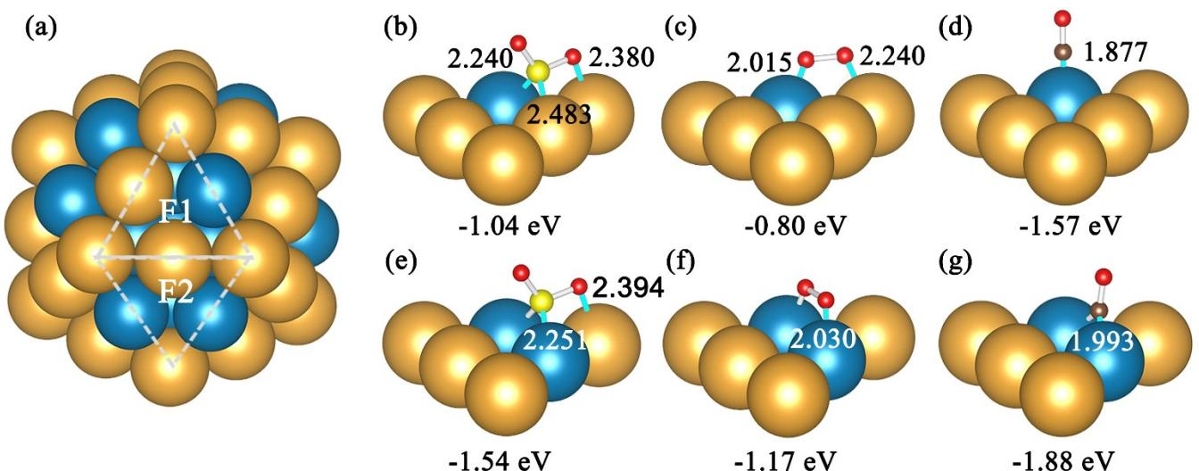
Figure S14 The accepted configurations of the icosahedral Pd<sub>27</sub>Au<sub>28</sub> with two types of LET facets (F1 and F2) (a) and the adsorption configurations of SO<sub>2</sub>, O<sub>2</sub>, and CO on F1 (b-d) and F2 (e-g), respectively. The adsorption energy data is labeled below the structural picture and the bond length information (in the unit of Å) is labeled in color cyan.
