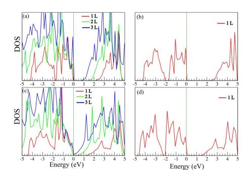
Figure S2: Electronic density of states using HSE of the (a) BiTeBr and (b) BiTeCl .Electronic density of states using HSE+SOC of (c) BiTeBr (d) BiTeCl monolayers.
