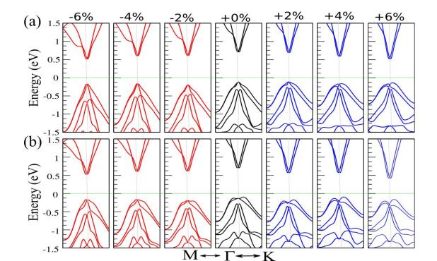
Figure S1: The electronic band structure of the BiTeCl monolayer under the influence of uniaxial strain.
