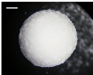
Fig. S6. Photograph for an alumina ball with cellulose powder after milling. Scale bar 1 mm.
