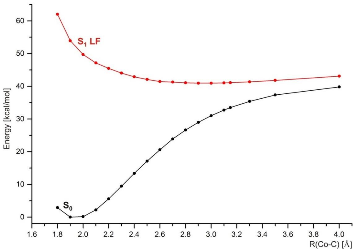
**Figure S5.** Potential energy curves of S<sub>0</sub> ground state and S<sub>1</sub> singlet state for {[Co<sup>III</sup>(corrin)]-CH<sub>3</sub>}<sup>+</sup> model complex as function Co-C axial bond length, obtained on the basis of calculation
