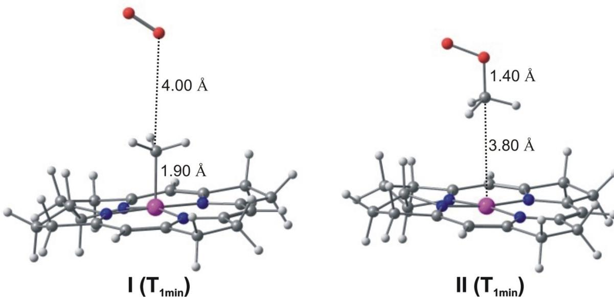
**Figure S4.** Corresponding optimized geometries of the I (T<sub>1min</sub>) and II (T<sub>1min</sub>) on the PES (Figures 4a and 4b).
