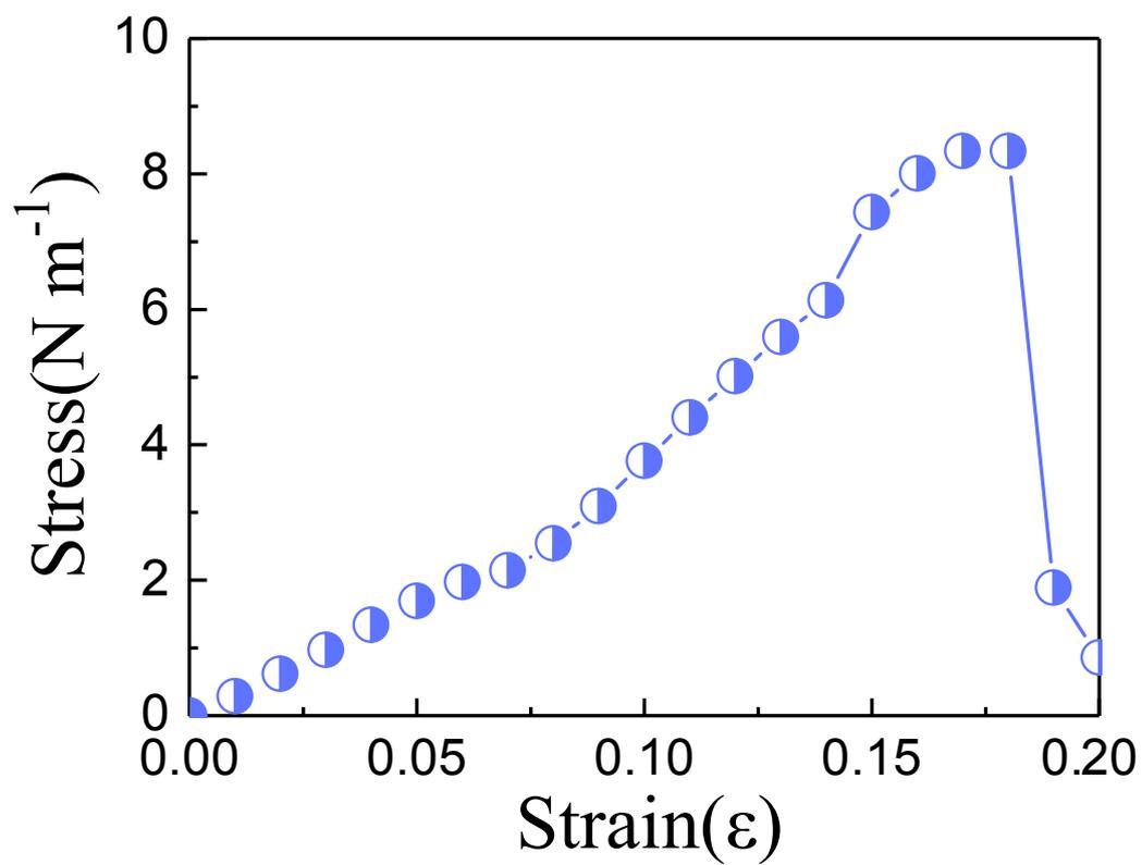
**Fig. S2.** The stress-strain diagram of the h1-B3S monolayer.
