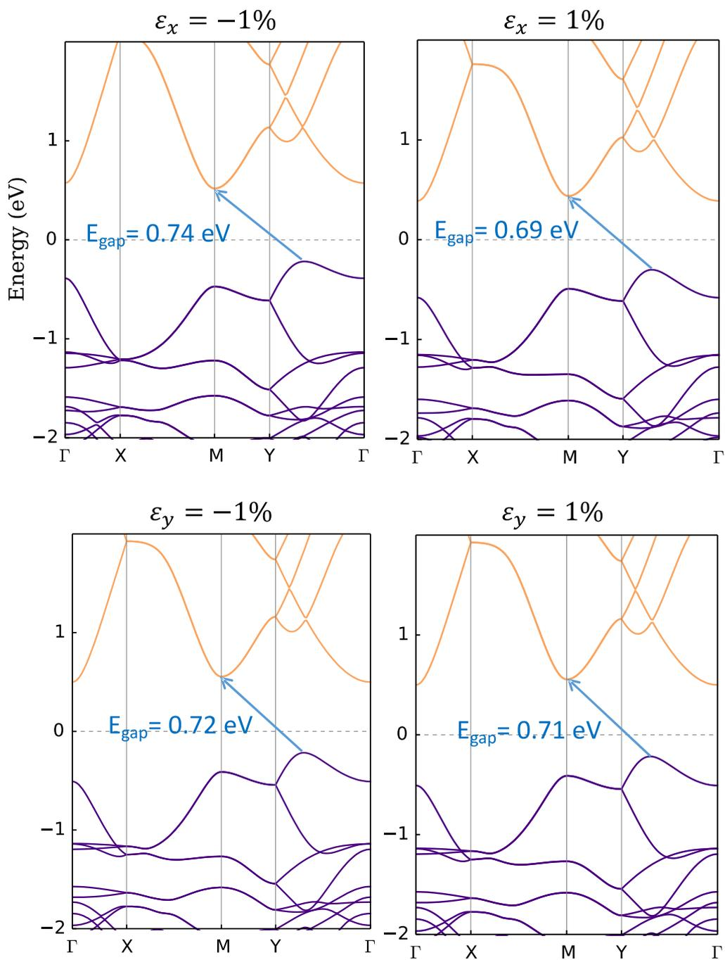
**Fig. S4.** Band structures of oxidized B<sub>3</sub>S monolayer under uniaxial strains.
