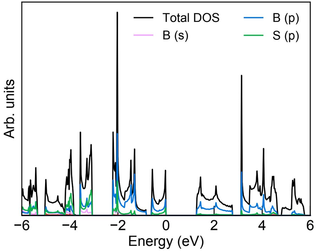
**Fig. S3.** Total and orbital projected DOS of the h1-B3S monolayer.
