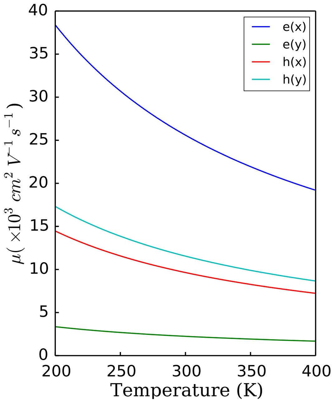
**Fig. S5.** Temperature dependent carrier mobilities along x and y directions.
