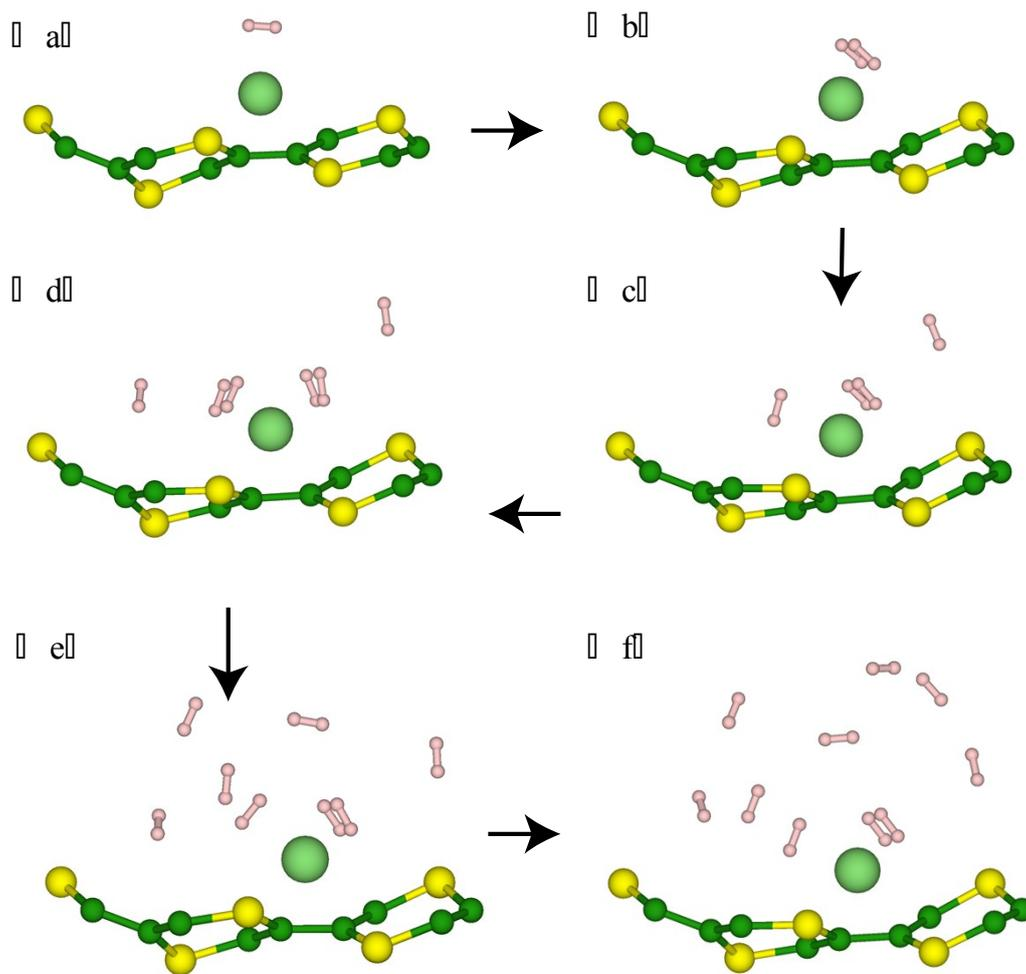
**Fig. S6.** Atomic configurations of H<sub>2</sub> adsorbed on Li-decorated h1-B<sub>3</sub>S monolayer.
