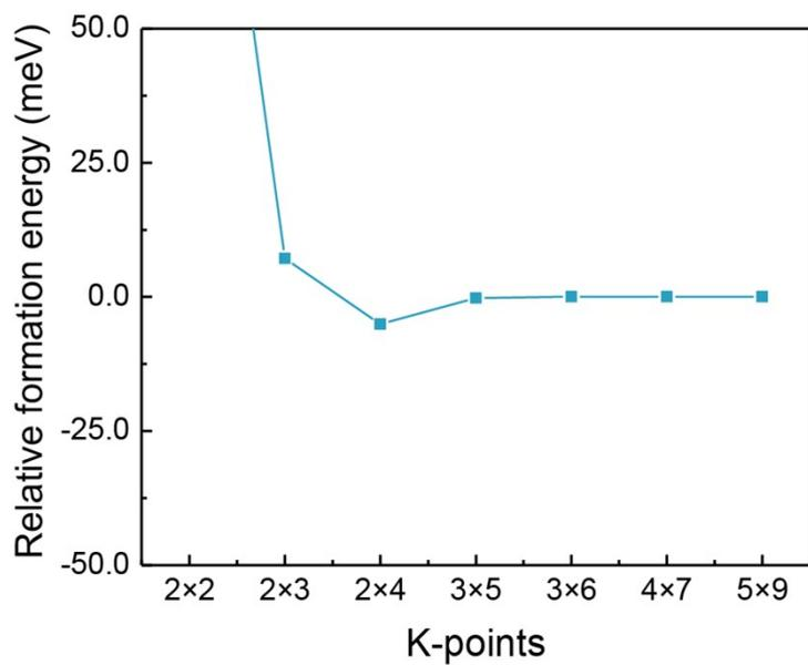
**Fig. S1.** The convergence test with respect to cutoff energy and K-point mesh of the h1-B<sub>3</sub>S monolayer using an orthogonal supercell.
