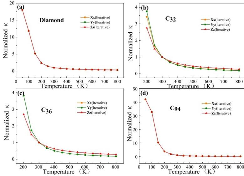
Figure S3. The thermal conductivity which is normalized at 300 K
