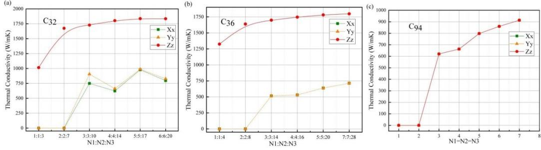
Figure S1. The convergence of thermal conductivity with respect to the grid sampling in  $Q$  space.
