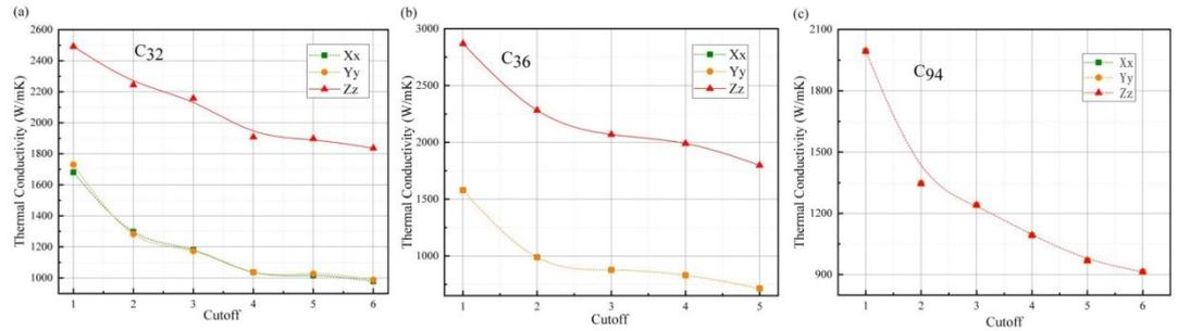
Figure S2. The convergence of thermal conductivity with respect to the cutoff distance of all cases.
