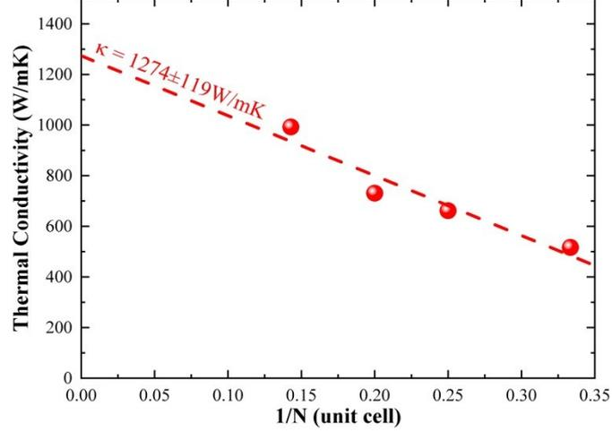
Figure S7. The dependence of thermal conductivity of  $C_{32}$  on the size of supercell for SED calculations. The fitted thermal conductivity of  $C_{32}$  is presented onsite.
