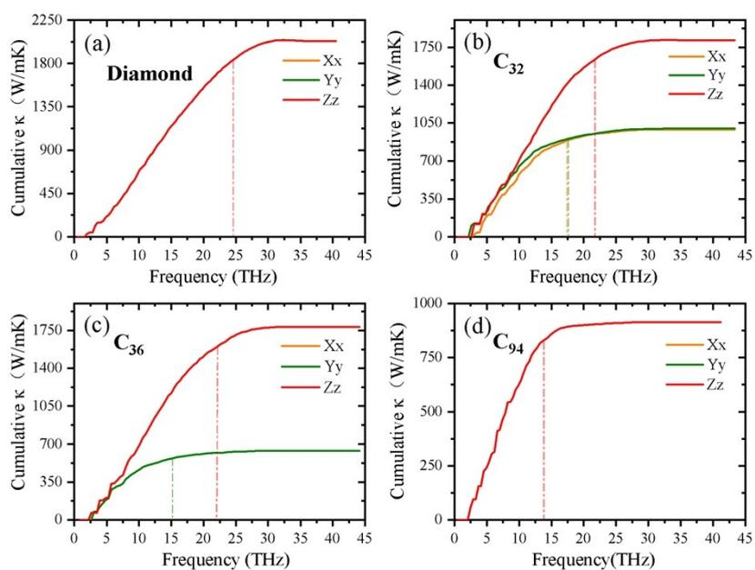
Figure S6. The cumulative thermal conductivities as a function of phonon frequencies. The dotted lines mark the 90% cumulated contribution to  $\kappa$ .
