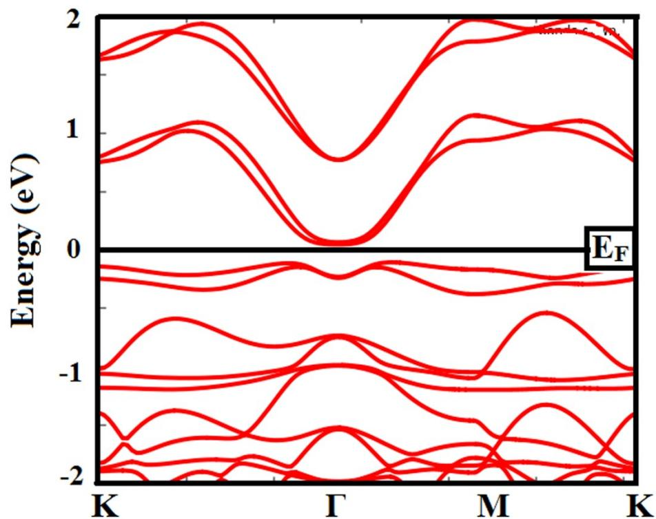
Fig. S1. Band structure of AB stacked ‘twin-graphene’ at electric field 1.5 V/Å.
