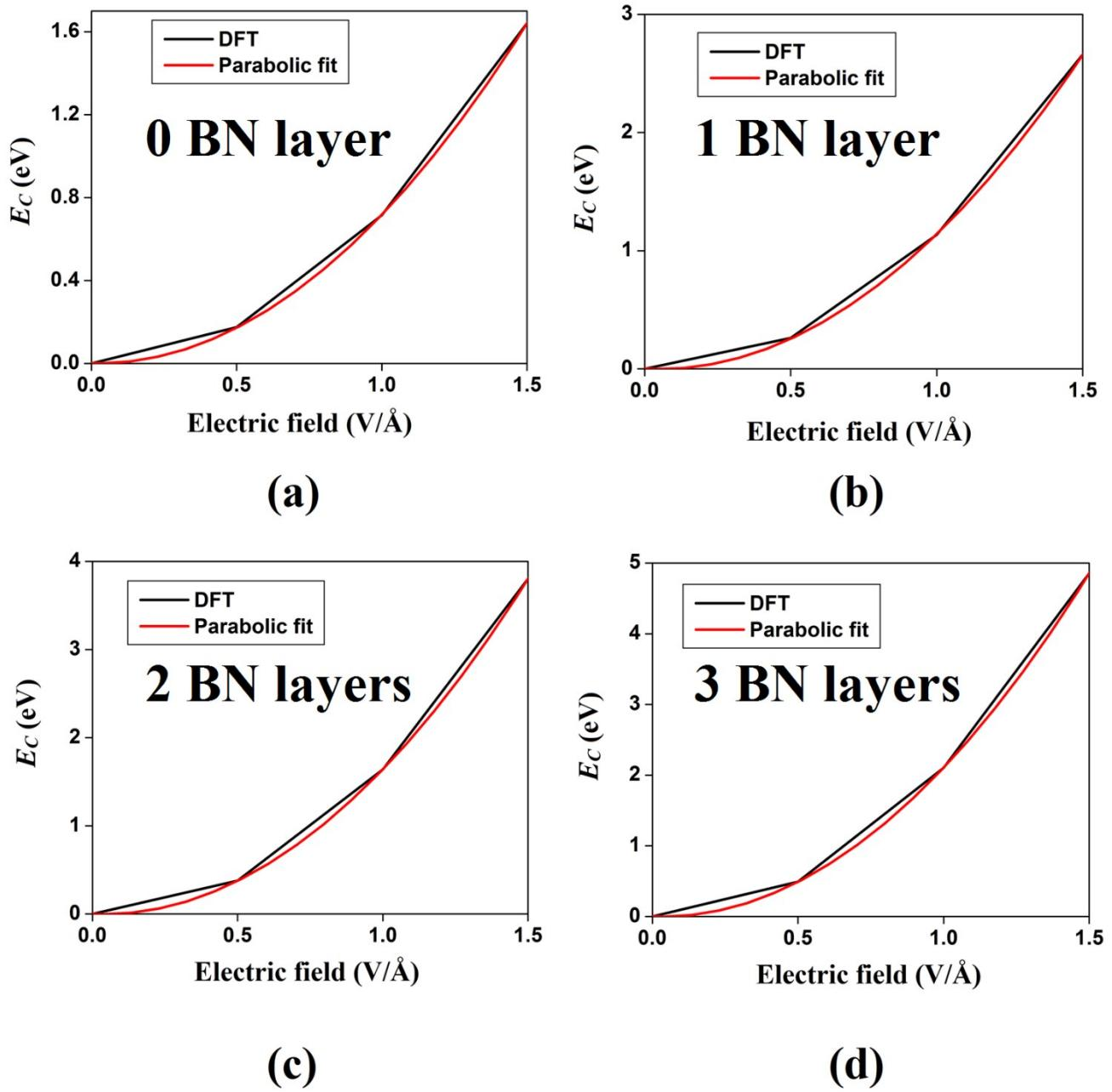
Fig. S3. Variation of the energy stored of NC and NDC models as a function of external electric field ( $\vec{E}_f$ ) for different number of ‘twin-graphene like BN sheet’ sandwiched between the pristine ‘twin-graphene’ layers.
