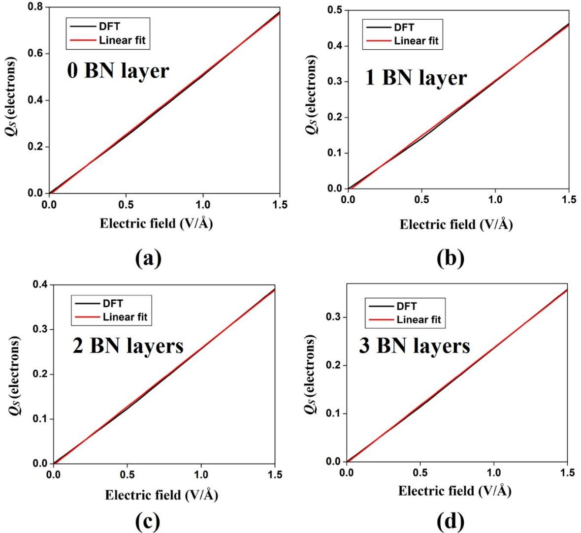
Fig. S2. Variation of the charge stored of NC and NDC models as a function of external electric field ( $\vec{E}_f$ ) for different number of ‘twin-graphene like BN sheet’ sandwiched between the pristine ‘twin-graphene’ layers.
