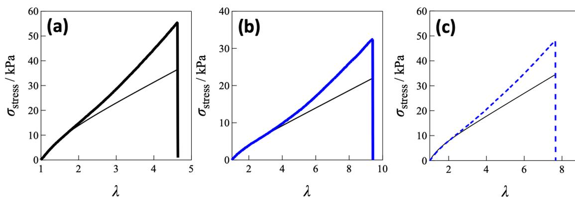
**Figure S4.** The fitting results (thin black line) using an equation,  $\sigma_{\text{stress\_calc}} = G(\lambda - \lambda^{-2})$ , for the experimental stress-elongation curves of (a) 5 wt% tetra/tetra-PEG ion gel, (b) 5 wt% and (c) 10 wt% tetra/linear-PEG ion gels.
