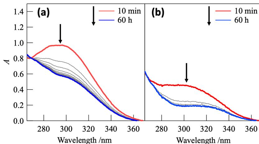
**Figure S1.** Time-dependent ultraviolet–visible spectra of the (a) tetra-PEG-MA and linear-PEG-SH (MA/SH = 1:0.5) and (b) (MA/SH = 1:2) in a 0.85 M LiTFSA/IL solution. The total polymer content in the solution was fixed at 2 wt% for both systems.
