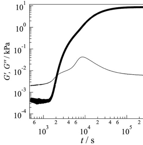
**Figure S2.** Storage ( $G'$ , bold line) and loss ( $G''$ , thin line) elastic moduli profiles for the 5 wt% tetra/tetra-PEG gelation system with the MA/SH ratio of 1:1.
