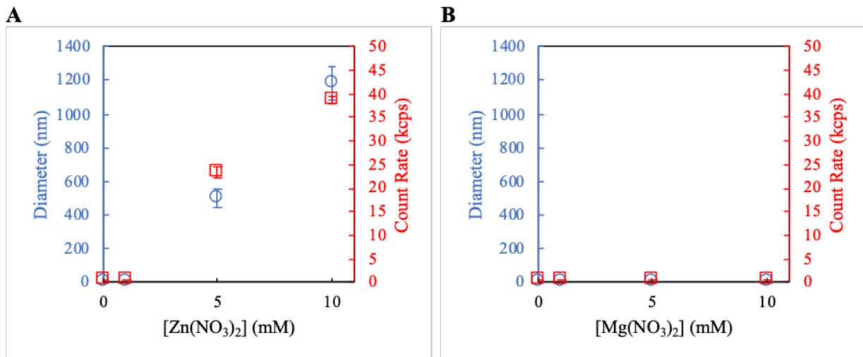
**Fig. S3. DLS Data of AkP with increasing concentrations of Zn<sup>2+</sup> and Mg<sup>2+</sup>.**
