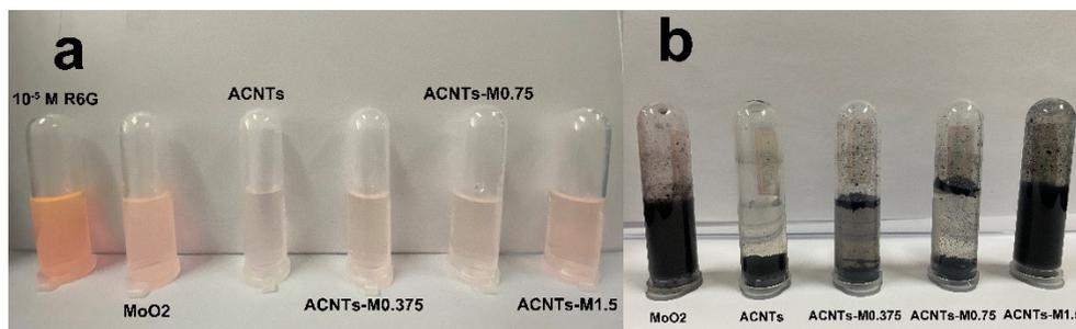
Fig. S5 the adsorption performance of R6G of different samples, (a) the upper layer of liquid after centrifugation after mixing for 30 seconds and (b) static settlement for 5 minutes.
