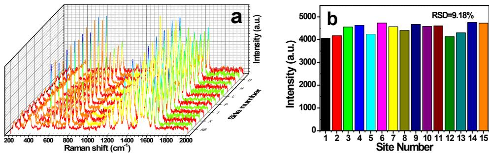
Fig. S3 (a) SERS spectra of R6G collected randomly from 15 spots of ACNTs-M0.75 substrate, (b) SERS intensity distribution at  $612\text{ cm}^{-1}$  corresponding to part (a).
