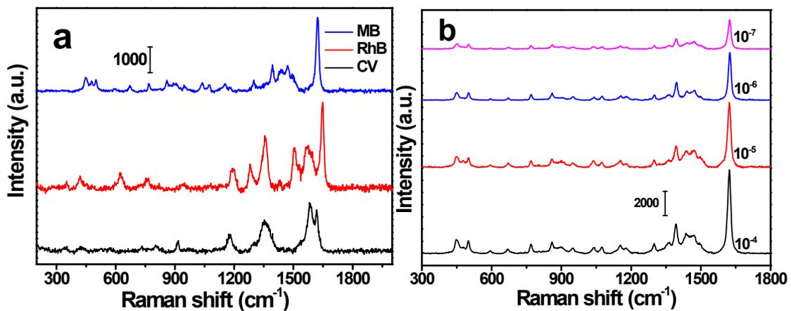
Fig. S4 (a) SERS spectra of a series of organic dyestuff with concentration of  $10^{-6}\text{ M}$  (MB, RhB and CV), (b) Raman spectra of MB with different concentrations on ACNTs-M0.5.
