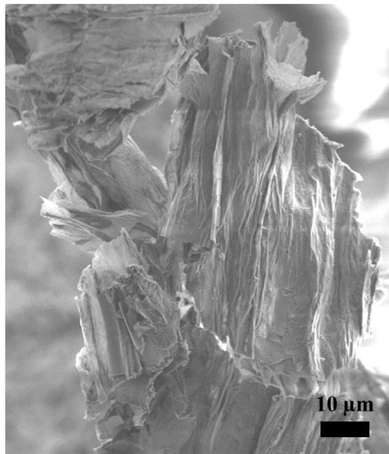
**Figure S6. SEM of Graphene Fiber Fracture after Uniaxial Tension.** The surface morphology of an accordion-folded graphene fiber after uniaxial tension and breaking.
