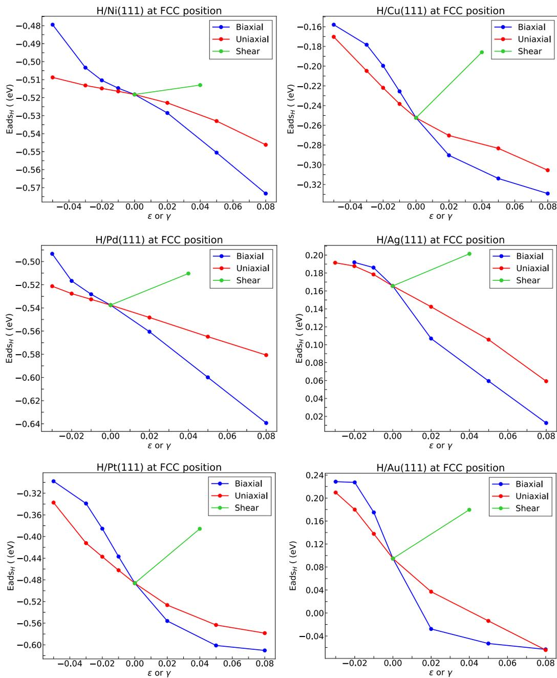
Figure S3: Adsorption energy of H as a function of strain from 5% compression to 8% tension at FCC positions for Ni, Cu, Pd, Ag, Pt, and Au. The legend indicates the type of strain.
