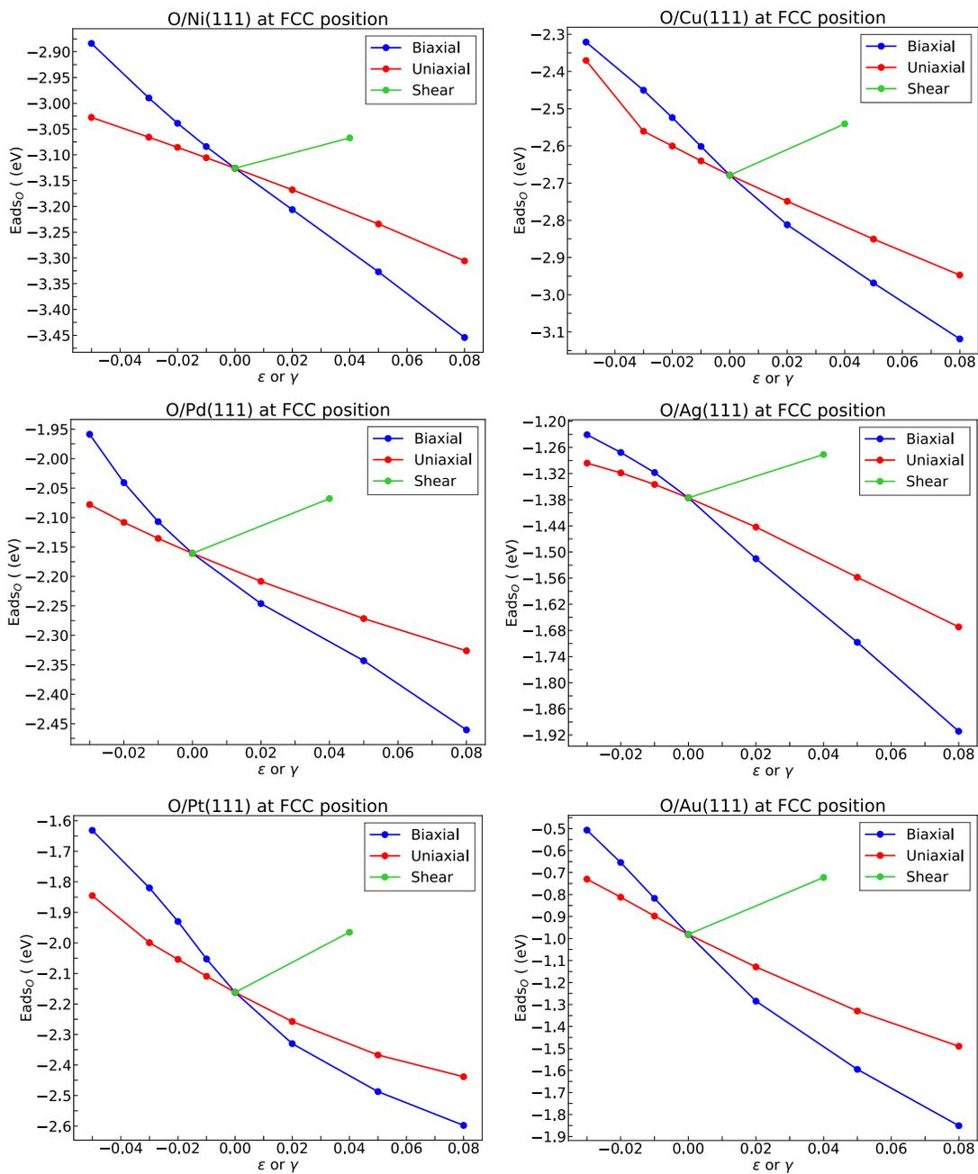
Figure S5: Adsorption energy of O as a function of strain from 5% compression to 8% tension at FCC positions for Ni, Cu, Pd, Ag, Pt, and Au. The legend indicates the type of strain.
