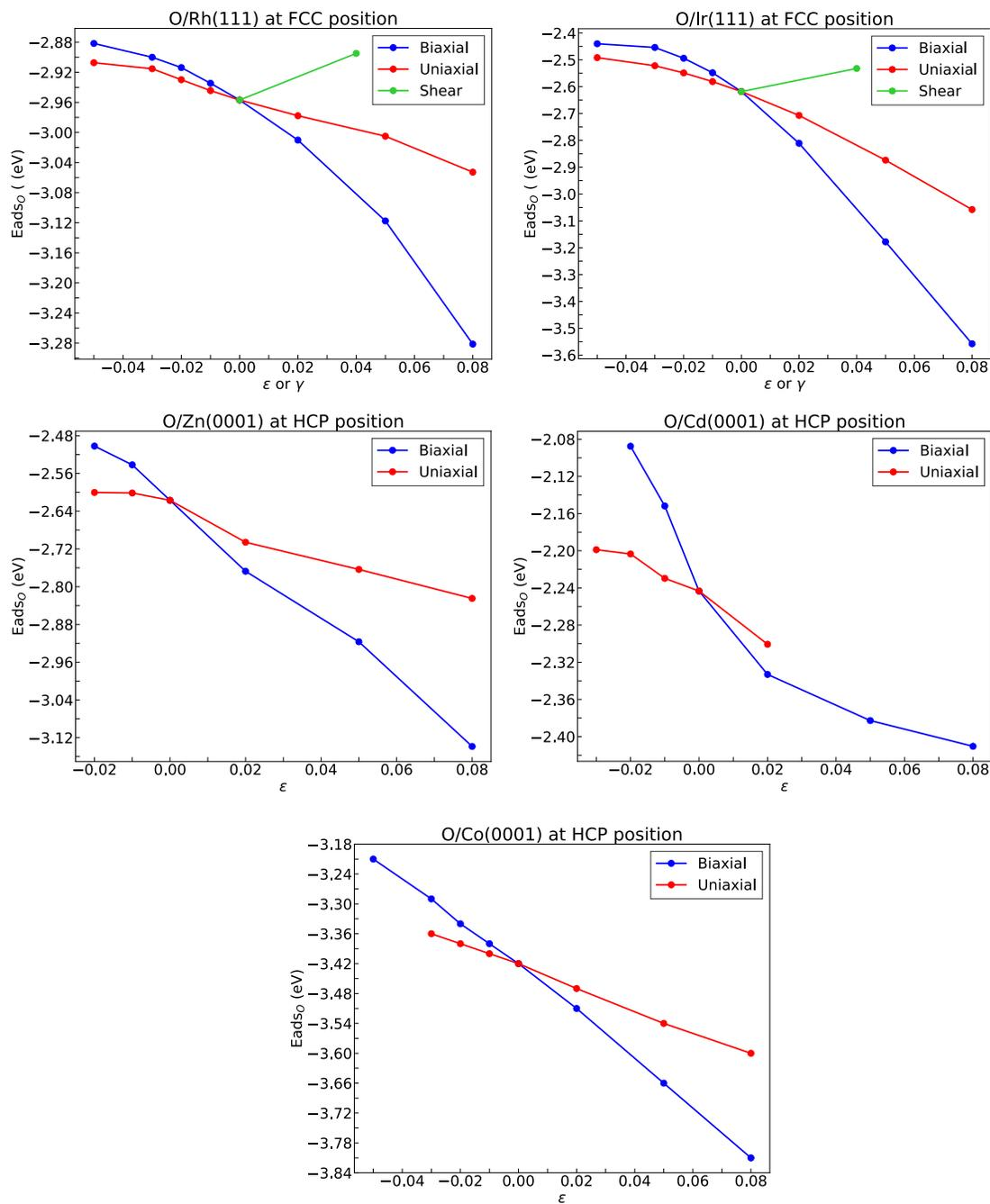
Figure S6: Adsorption energy of O as a function of strain from 5% compression to 8% tension at FCC positions for Rh, and Ir, and HCP positions for Zn, Cd, and Co. The legend indicates the type of strain.
