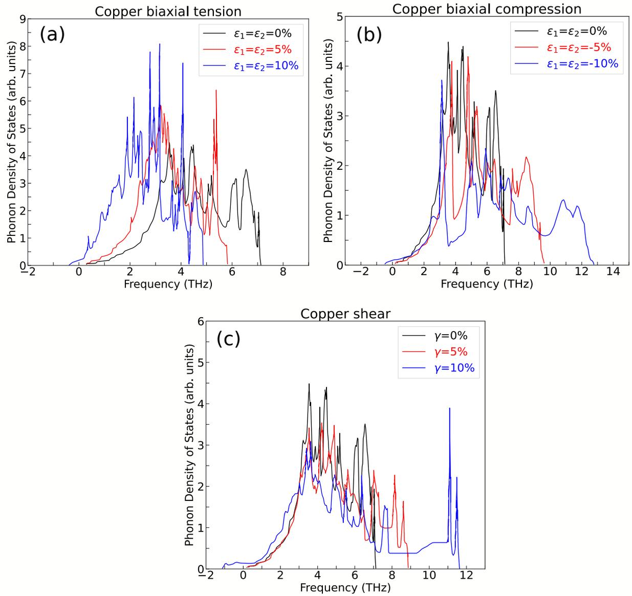
Figure S2: Phonon density of states for the (111) fcc Cu slab subjected to: (a) biaxial tensile strains. (b) Biaxial compressive strains. (c) Shear strains.
