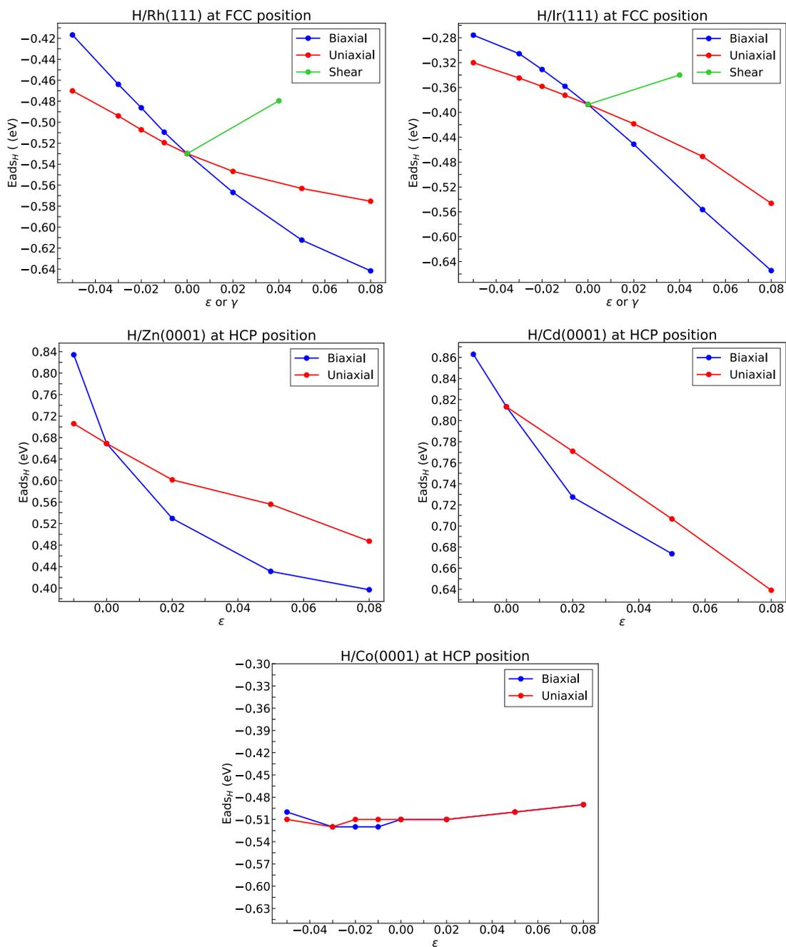
Figure S4: Adsorption energy of H as a function of strain from 5% compression to 8% tension at FCC positions for Rh, and Ir, and HCP position for Zn, Cd, and Co. The legend indicates the type of strain.
