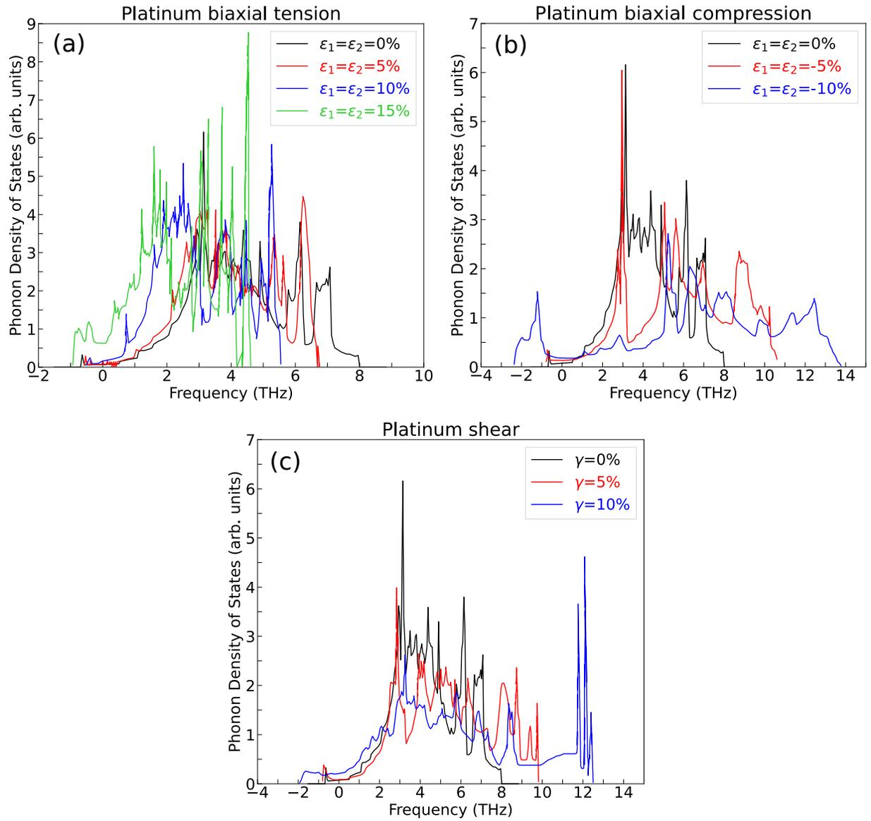
Figure S1: Phonon density of states for the (111) fcc Pt slab subjected to: (a) biaxial tensile strains. (b) Biaxial compressive strains. (c) Shear strains.
