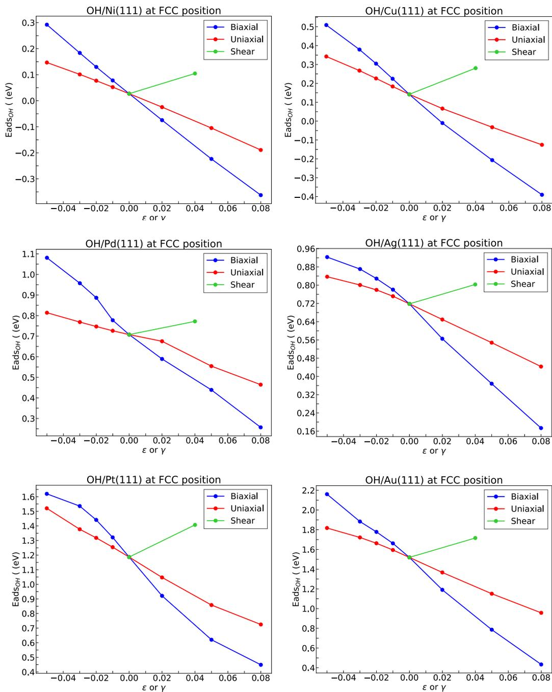
Figure S7: Adsorption energy of OH as a function of strain from 5% compression to 8% tension at FCC positions for Ni, Cu, Pd, Ag, Pt, and Au. The legend indicates the type of strain.
