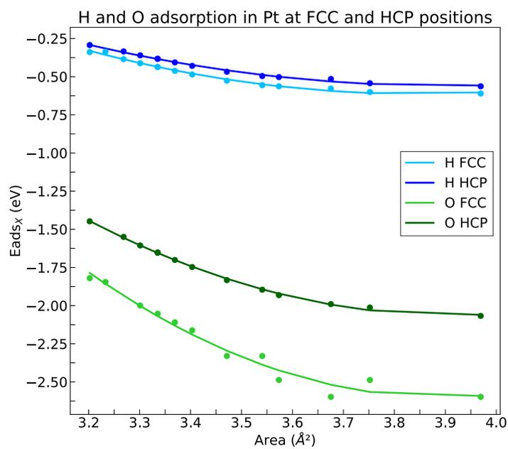
Figure S9: Adsorption energy of H and O in platinum as a function of the area of the FCC and the HCP sites from 5% compression to 8% tension. Dots represent the DFT calculations and lines show the quadratic fittings.
