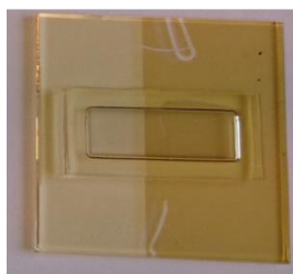
Figure S1. Image of a representative sample. A 20-nm lying \alpha -6T layer with a half of the layer covered with C 60 . The size of the sample is 5 \times 20 \text{ mm}^2 (inside the encapsulation cap).
