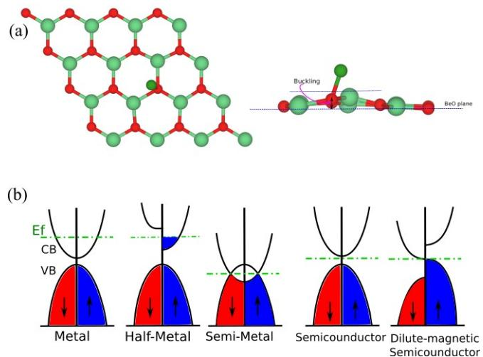
Fig S3. (a) Optimized atomic structure of BeO monolayer with adsorbed B atom at top of O host atom. Buckling of O bonded to B indicated as schematically. (b) Schematic diagram of different electronic states including of metal, half-metal(HM), semiconductor (SC) and dilute magnetic semiconductors (DMSC).
