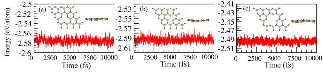
Fig S4. Ab initio molecular dynamics (AIMD) for Be monolayer with (a) a single Be vacancy, (b) a single O vacancy and (c) double vacancy Be+O defects. at 400 K temperature. Top and side views of the structure after 5 ps of simulation demonstrated as insets.
