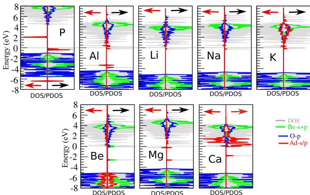
Fig S4. Total DOS and PDOS of different adatom adsorbed on the BeO monolayer
