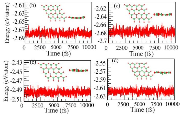
Fig S5. Ab initio molecular dynamics (AIMD) for BeO monolayer doped with (a) B Be , (b) N Be , (c) C Be , and (d) B O at 400 K temperature. Top and side views of the structure after 5 ps of simulation demonstrated as insets.
