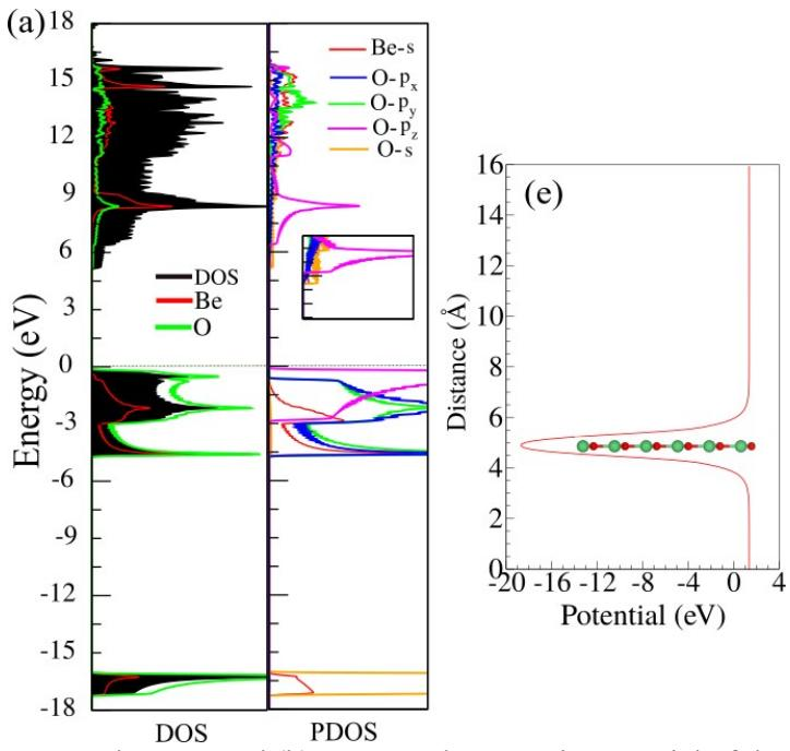
Fig S1. (a) DOS and PDOS and (b) average electrostatic potential of the BeO monolayer
