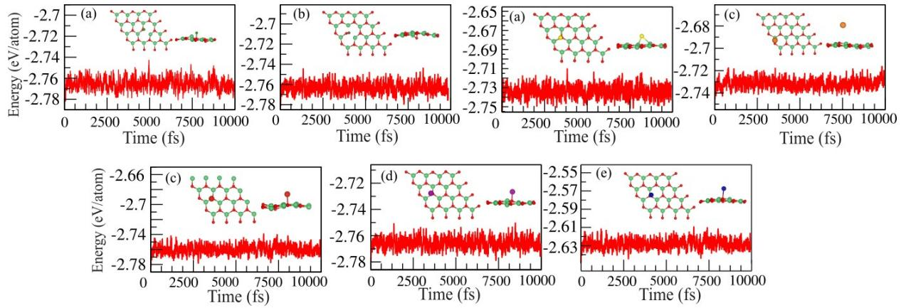
Fig S2. Ab initio molecular dynamics (AIMD) for BeO monolayer adsorbed with (a) B , (b) C , (c) S , (d) Mg , (e) V , (f) Mn and (f) Co adatoms at 400 K temperature. Top and side views of the structure after 5 ps of simulation demonstrated as insets.:
