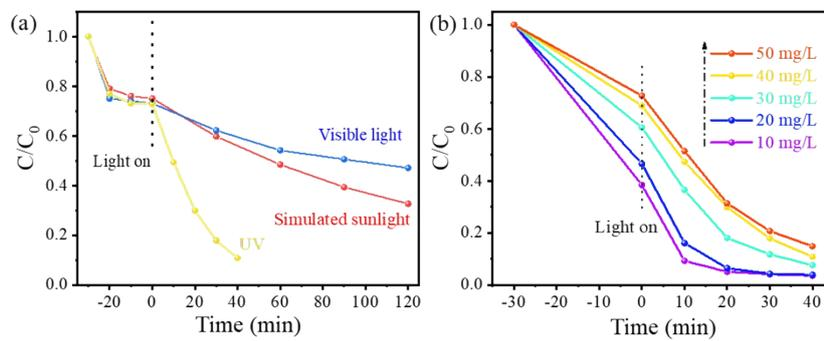
Fig. S10 Degradation of TC solutions (a) under different light sources (50 mg/L), and (b) with different TC concentrations
