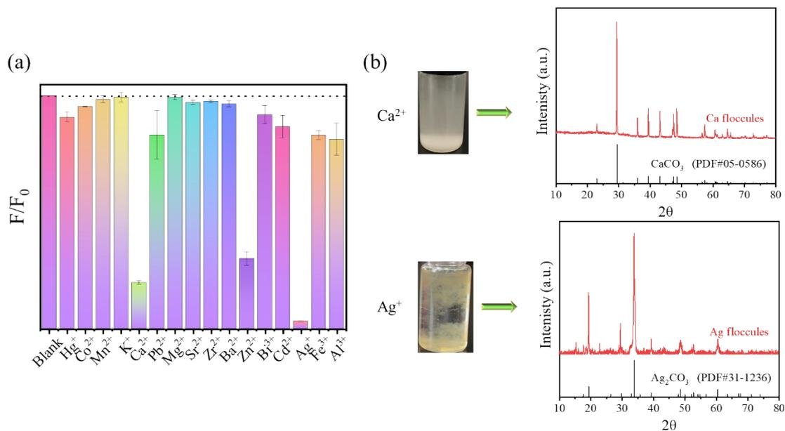
Fig. S4 (a) Fluorescence responses of CNQDs in the presence of different metal ion (24  $\mu\text{M}$ ) or calcium hydroxide saturated solution; (b) XRD patterns of floccules
