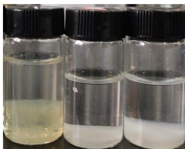
Fig. S5 Digital photo of different carbon source with urea after adding  $\text{Zn}(\text{NO}_3)_2$  (from left to right: citric acid, propanedioic acid, and glutaric acid)
