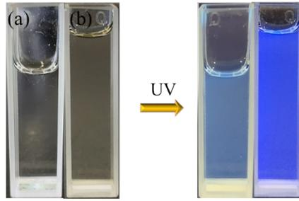
Fig. S7 Photos of CNQDs synthesized from (a) urea, (b) urea and BA (1:0.1) under daylight (left) and UV light (right)
