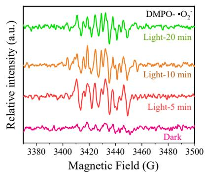
Fig. S11 ESR spectra of DMPO-•O<sub>2</sub><sup>-</sup> adduct recorded with of ZnO in the dark and under UV-Vis light irradiation
