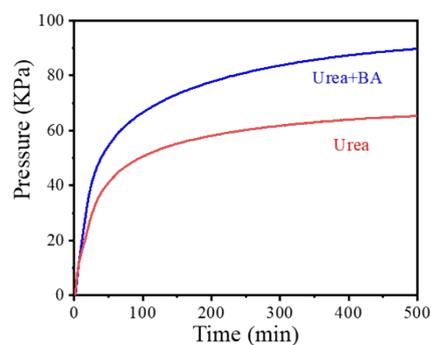
Fig. S6 Time dependence of the gas pressure under the temperature of 453K (the fitting curves of the decomposition rate versus time was determined by the P versus T curves measured by DVST)
