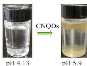
Fig. S3 Preparation of CNQD/BZC from saturated solution of zinc nitrate
