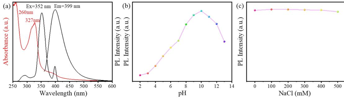
Fig. S8 (a) Absorbance, excitation, and emission spectra of CNQDs; PL intensities of CNQDs (b) in different pH values, and (c) in ionic strength
