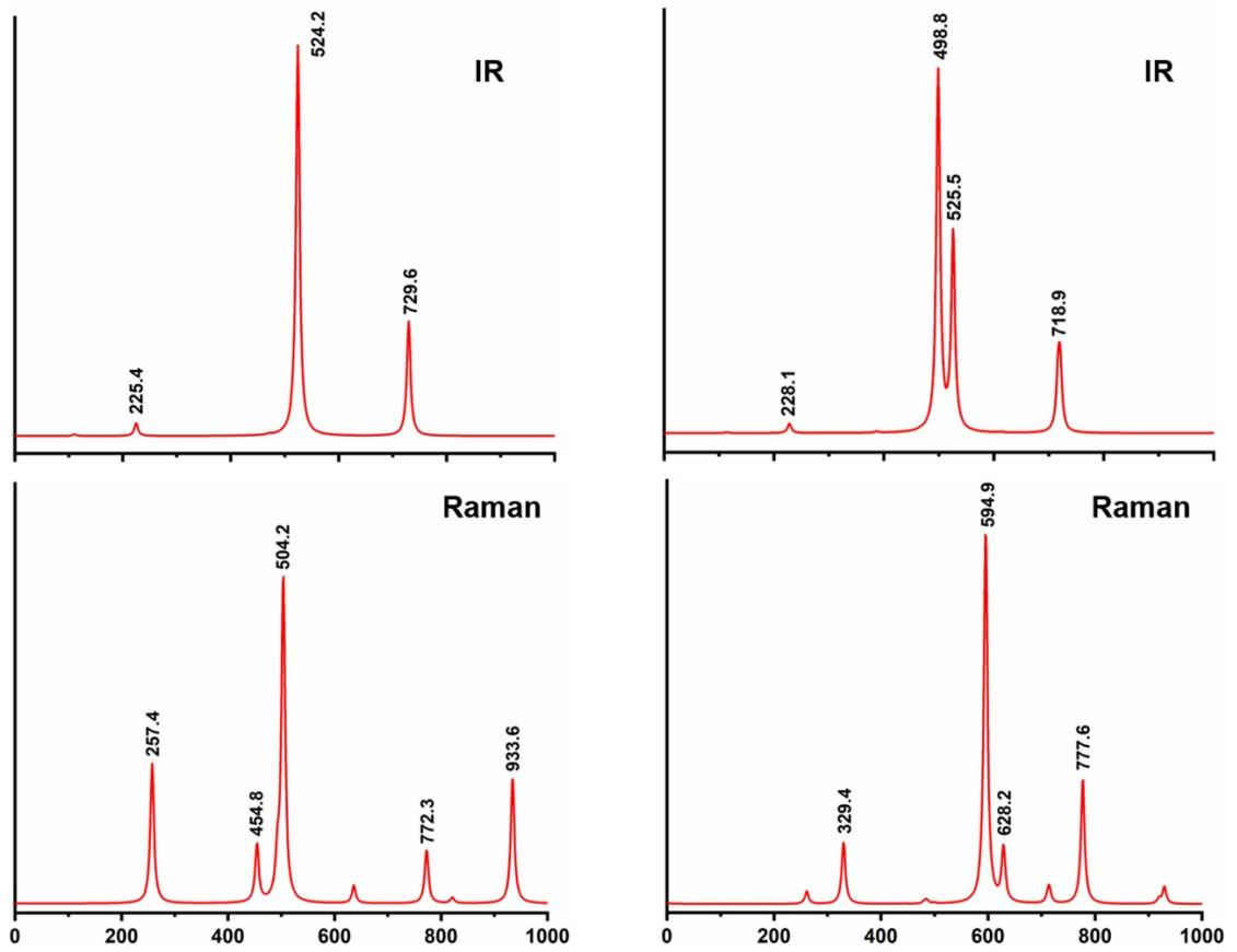
**Fig. S13** The simulated IR and Raman of Np@B<sub>20</sub> (left) and Pu@B<sub>20</sub> (right) at the DFT/PBE0/6-311+G\*/RECP level of theory.
