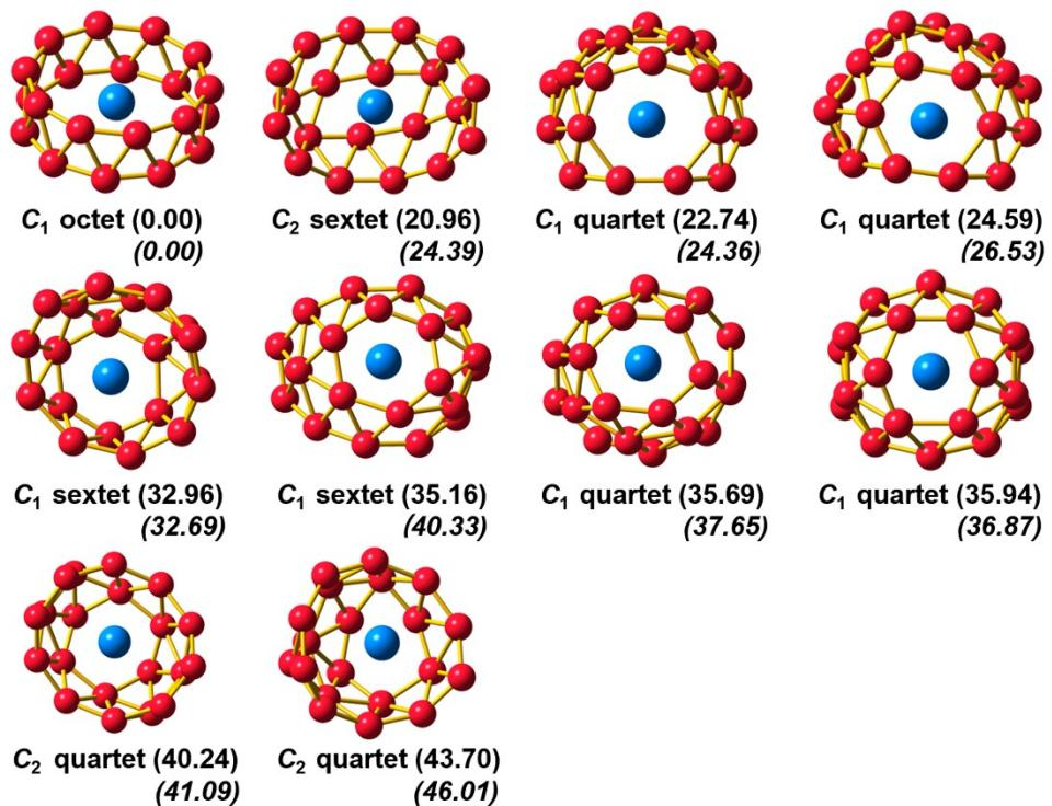
**Fig. S2** Low-lying isomers of Np@B<sub>20</sub> with the relative energies (kcal/mol) at the DFT/PBE0/6-311+G\*/RECP in the first row and DFT/TPSSh/6-311+G\*/RECP levels in the second rows (*in italic*). Red and blue spheres represent B and Np, respectively. All the energies have been corrected for zero-point energies.
